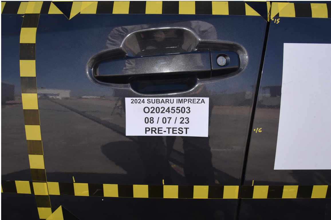
FIGURE 21. Pre-Test Left Front Door Latch Close-Up
