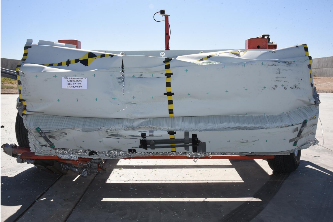
FIGURE 85. Post-Test Front View of MDB Impactor Face
