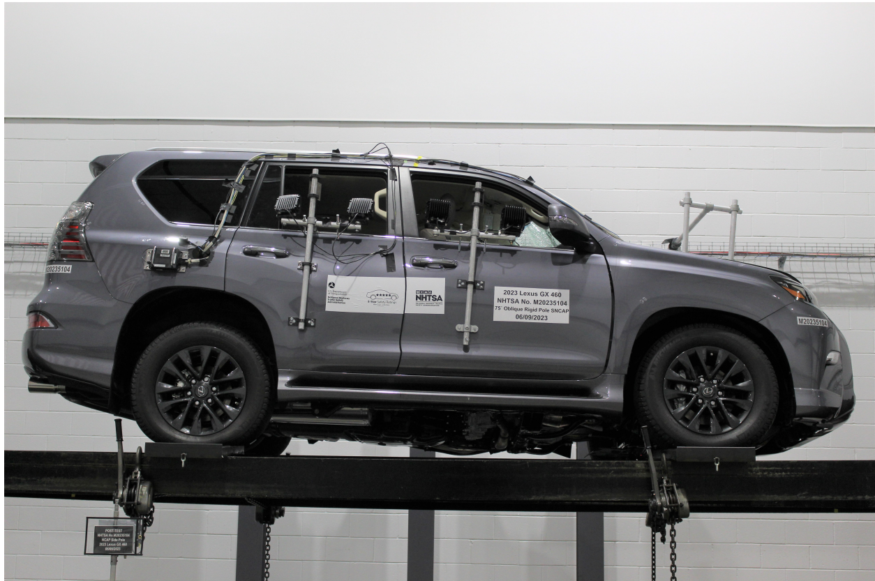
Figure A-69: FMVSS No. 301 Static Rollover 360 Degrees
