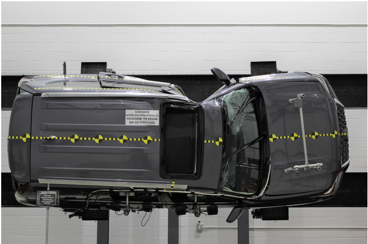
Figure A-68: FMVSS No. 301 Static Rollover 270 Degrees
