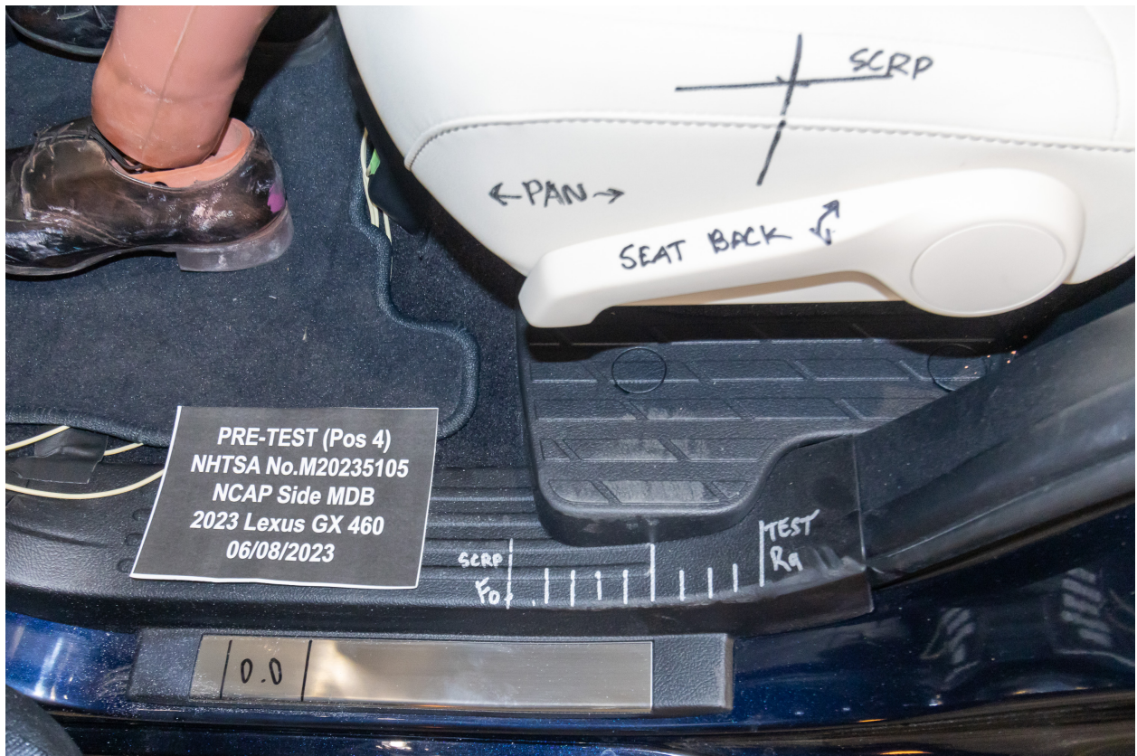
Figure A-66: Pre-Test Close-Up Left Side View of Rear Passenger Seat Track
