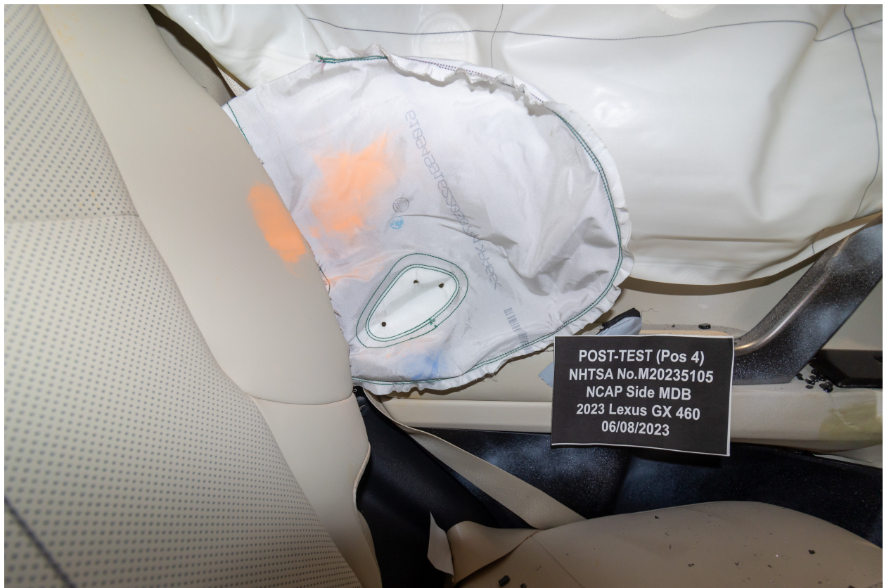
Figure A-78: Post-Test Rear Passenger Dummy Close-Up Torso Contact with Side Air bag View
