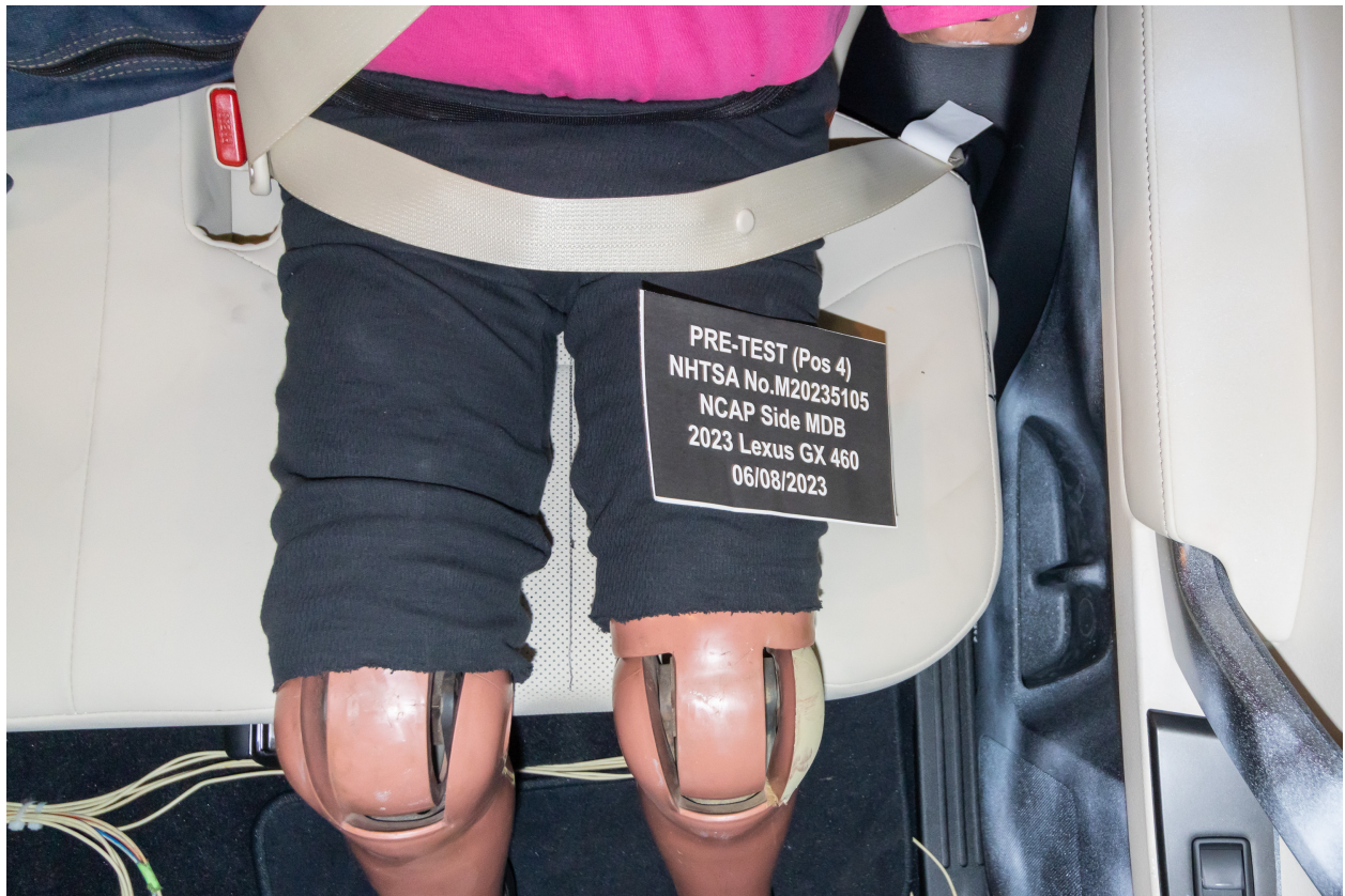
Figure A-61: Pre-Test Overhead View of Rear Passenger Dummy Thighs on Seat Pan
