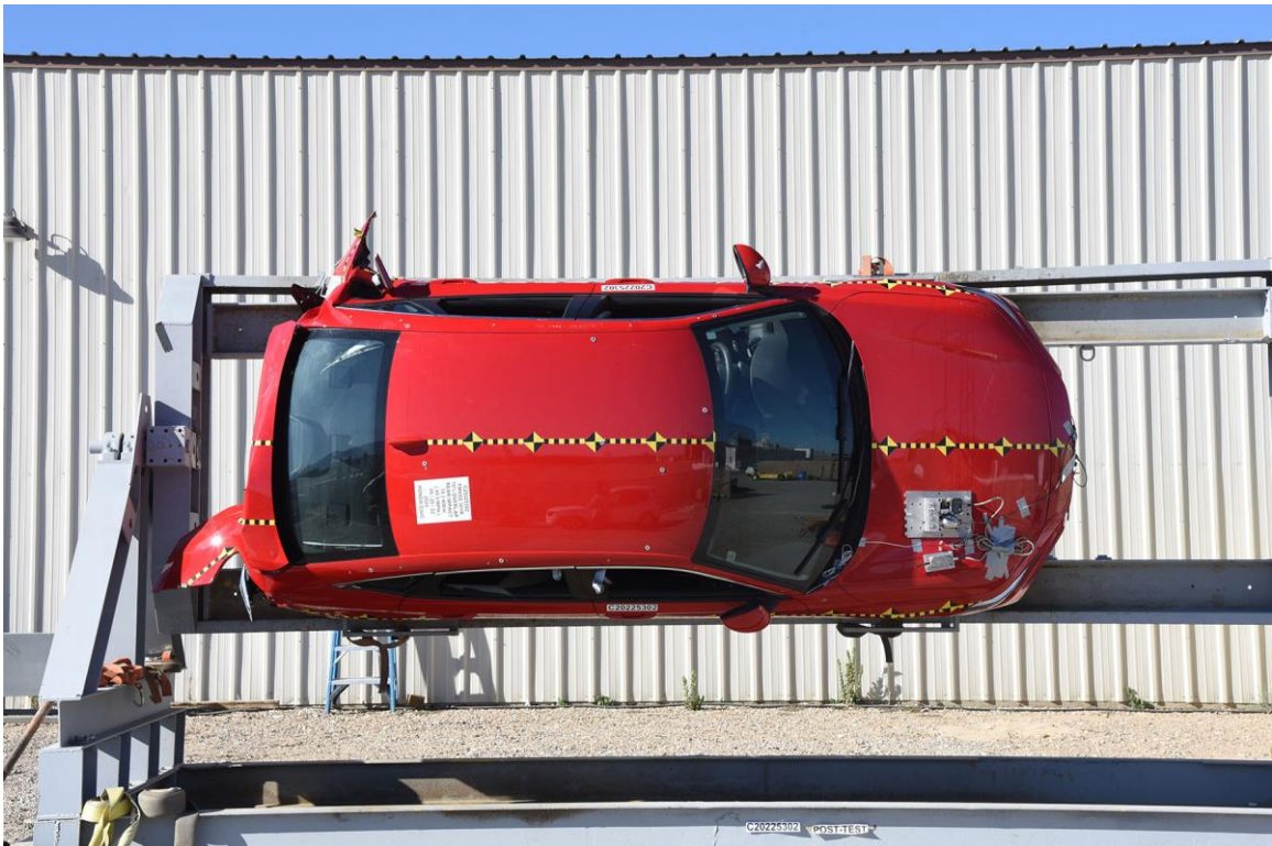
FIGURE 26. Test Vehicle at 270° on FMVSS 301 Static Rollover Device
