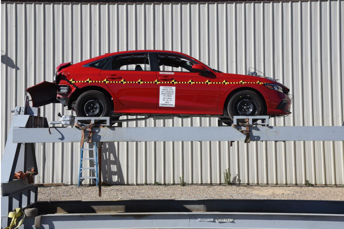
FIGURE 23. Test Vehicle at 0° on FMVSS 301 Static Rollover Device
