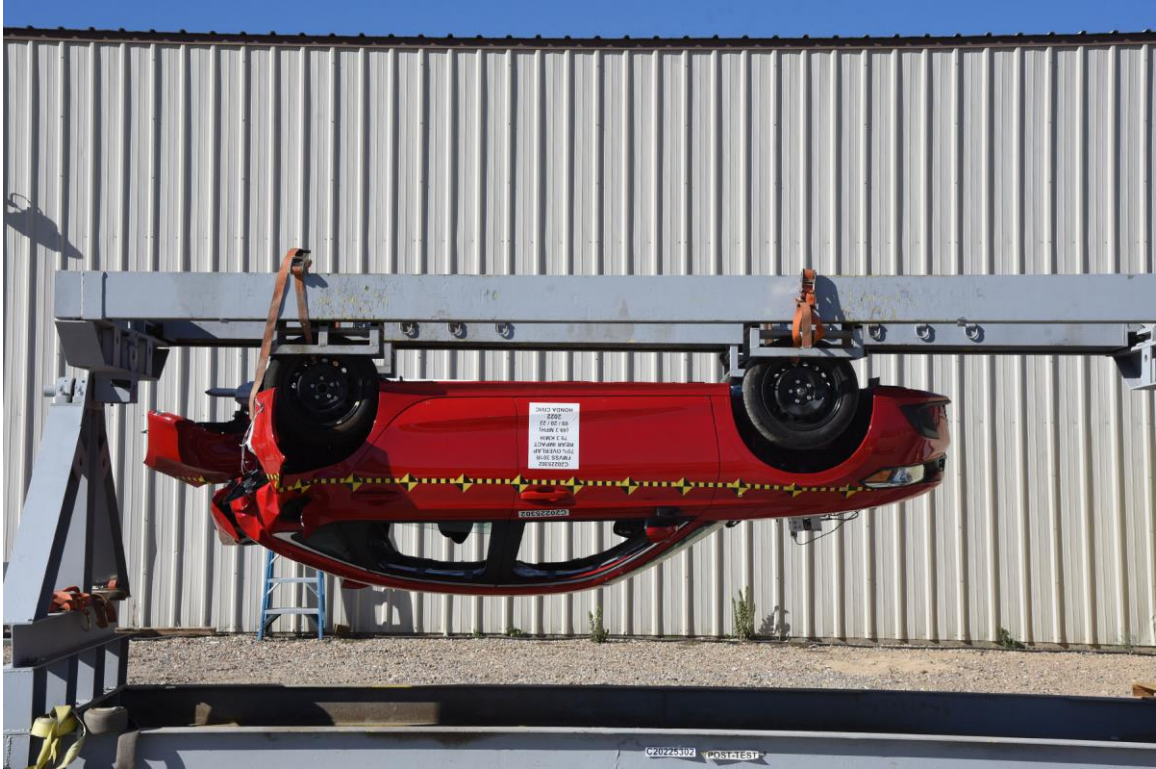
FIGURE 25. Test Vehicle at 180° on FMVSS 301 Static Rollover Device
