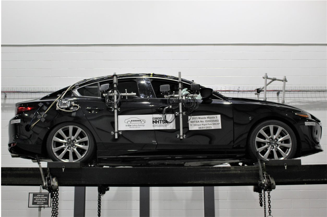
Figure A-69: FMVSS No. 301 Static Rollover 360 Degrees
