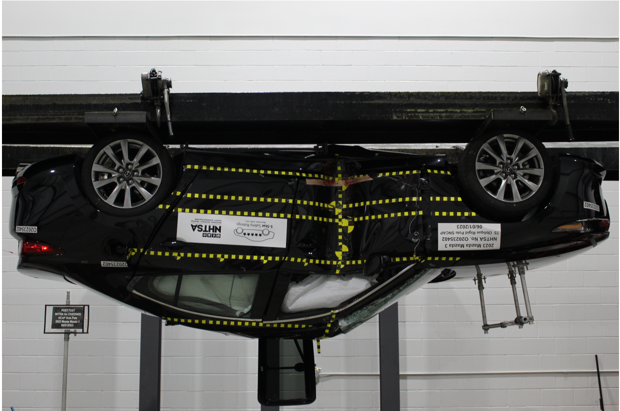
Figure A-67: FMVSS No. 301 Static Rollover 180 Degrees
