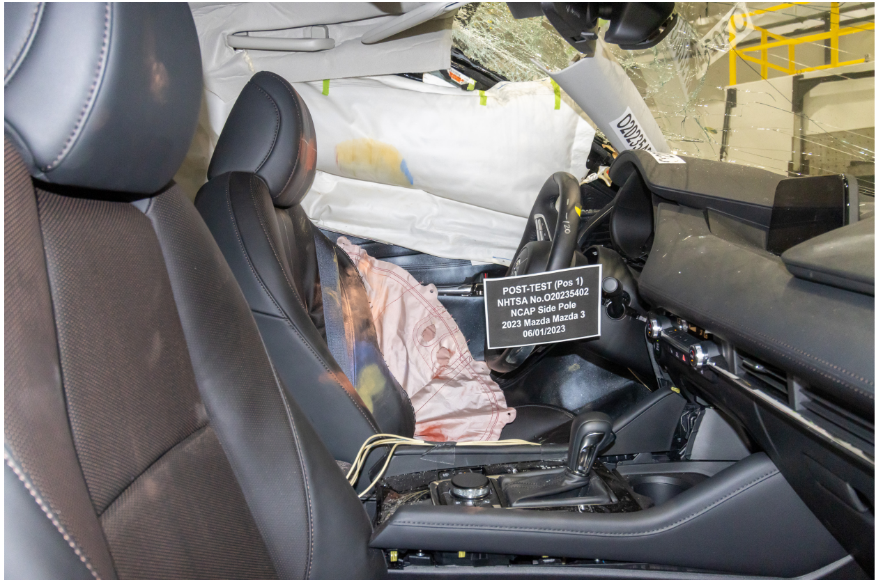
Figure A-45: Post-Test Inner Door Panel View Showing Dummy Contact Location
