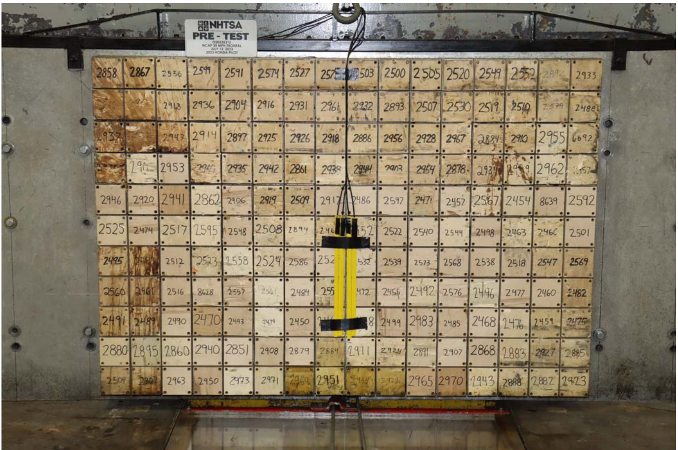
Photo No. 002 - Pre-Test Load Cell Wall
