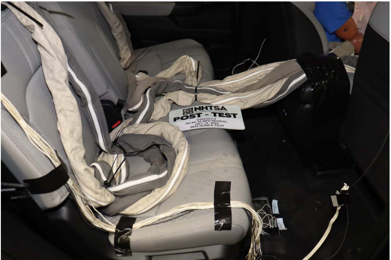
Photo No. 029 - Post-Test Dummy Cable Routing
