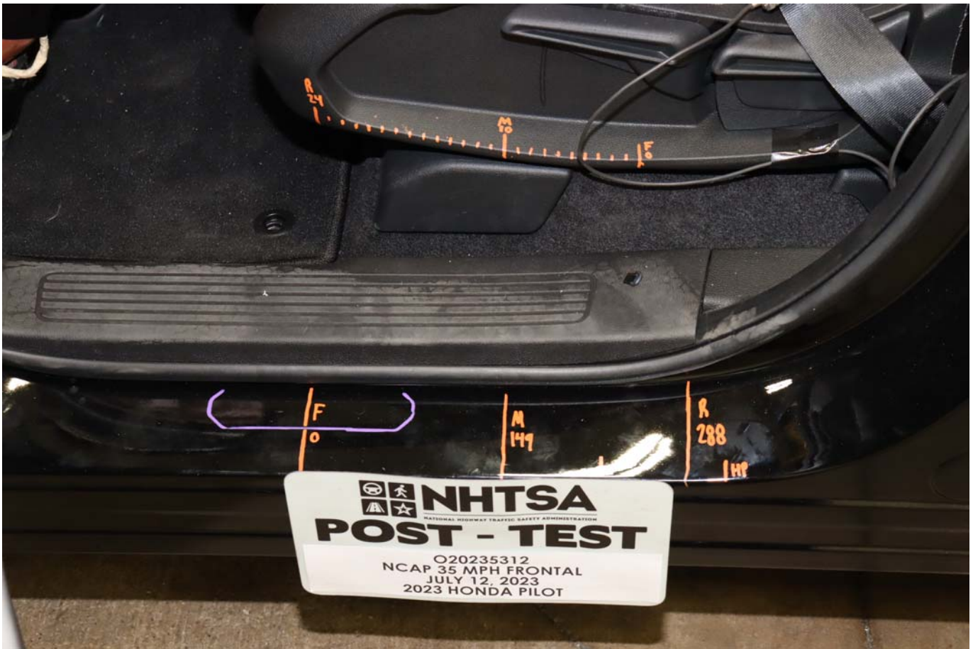
Photo No. 037 - Post-Test Driver's Seat Fore-Aft Markings
