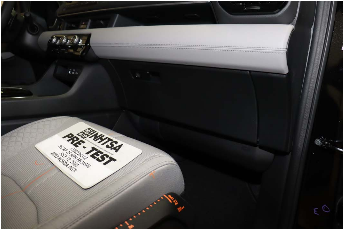
Photo No. 067 - Pre-Test Passenger's Side Knee Bolster
