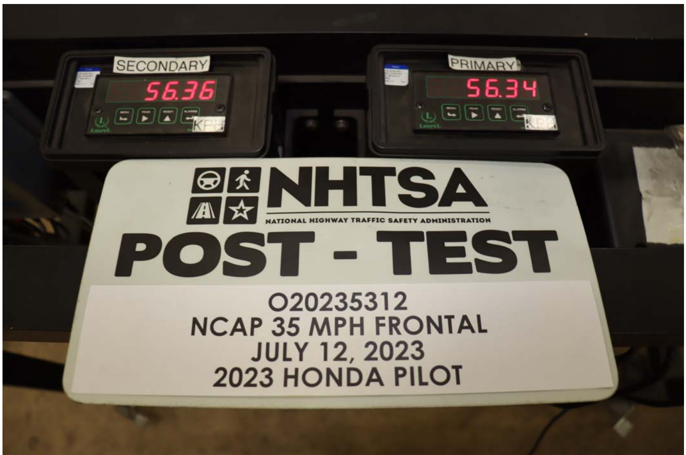
Photo No. 076 - Post-Test Speed Trap Read-Out
