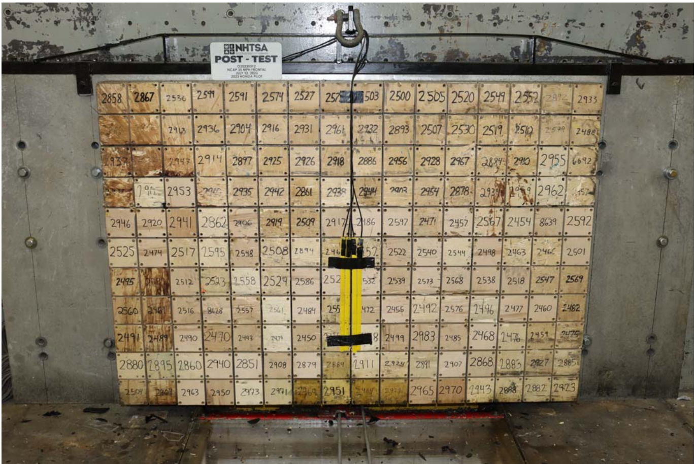
Photo No. 003 - Post-Test Load Cell Wall
