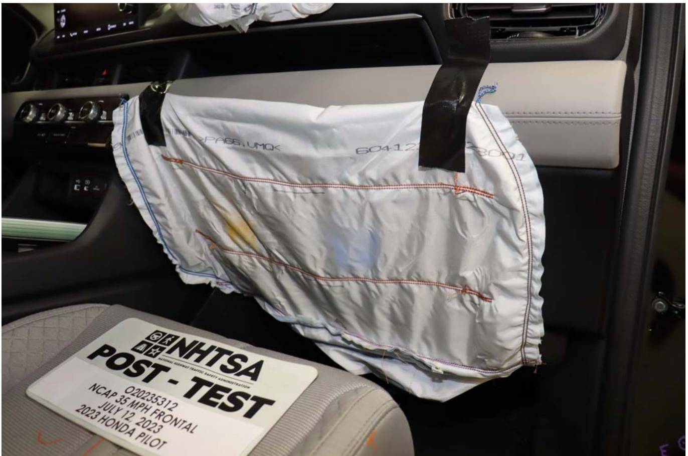
Photo No. 068 - Post-Test Passenger's Side Knee Bolster
