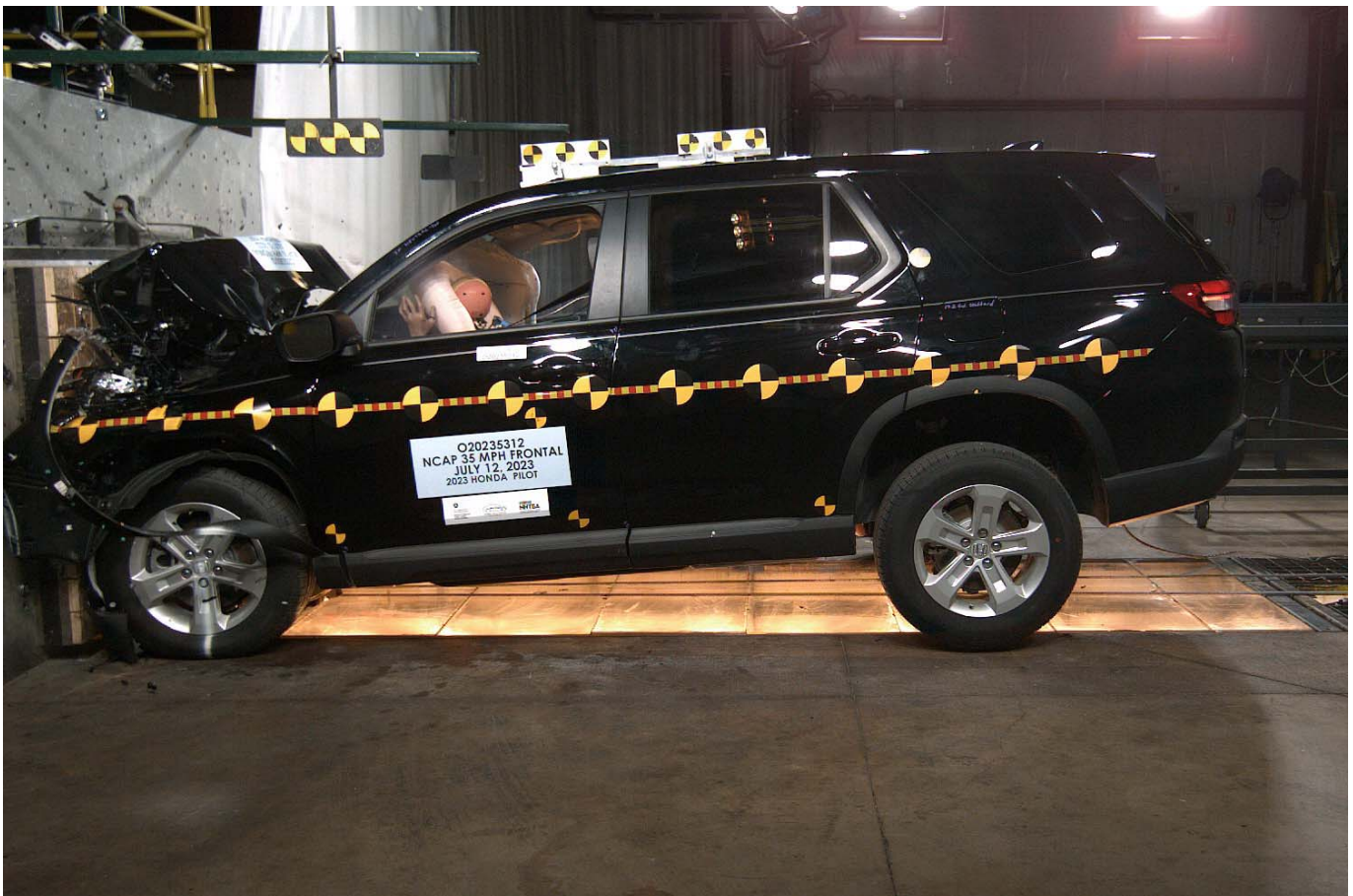
Photo No. 082 - 2023 Honda Pilot AWD LX 5-Door SUV Frontal Impact Event
