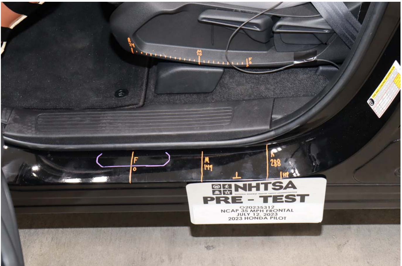
Photo No. 036 - Pre-Test Driver's Seat Fore-Aft Markings
