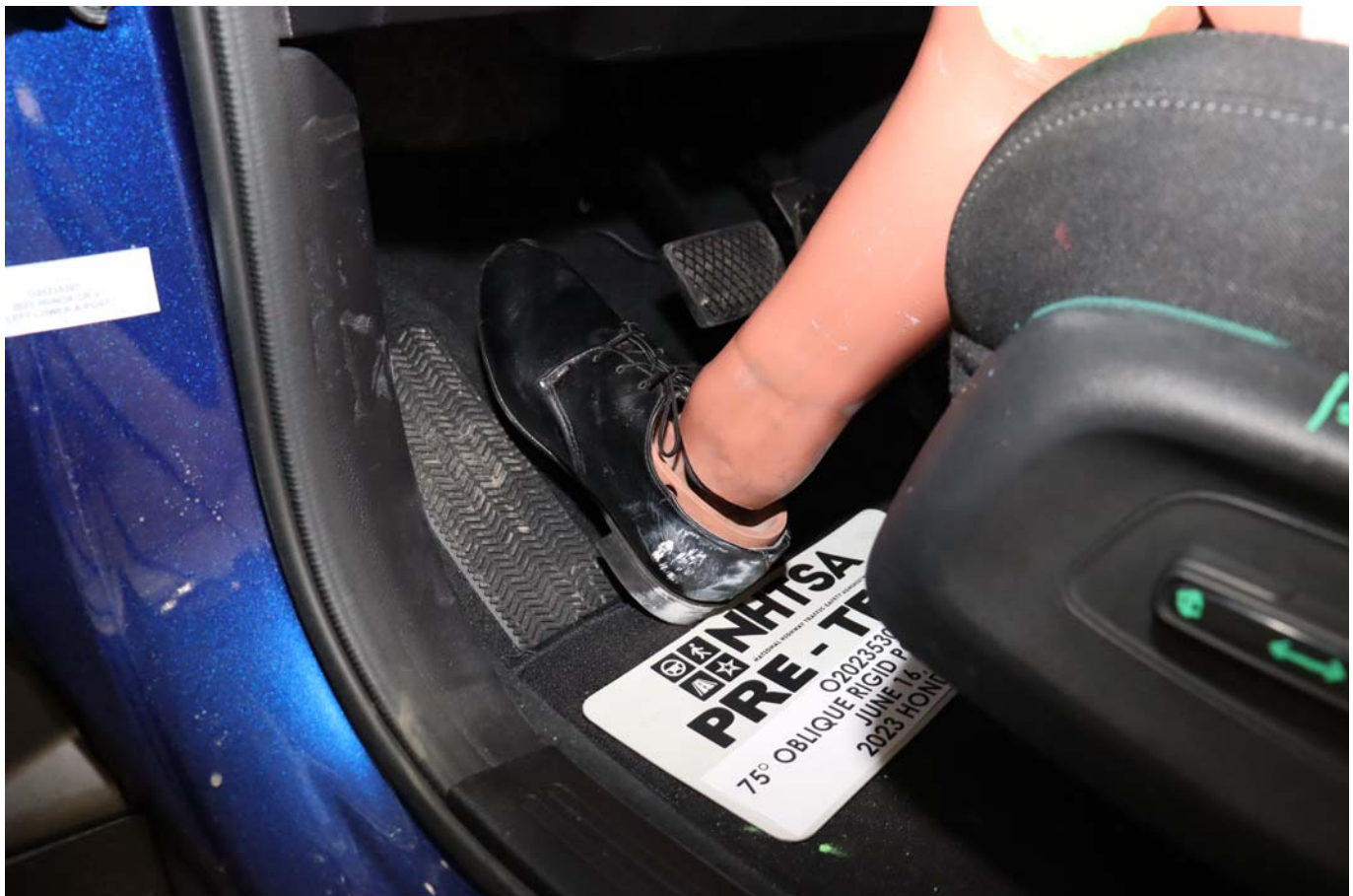
Photo No. 032 - Pre-Test Placement of Dummy's Feet
