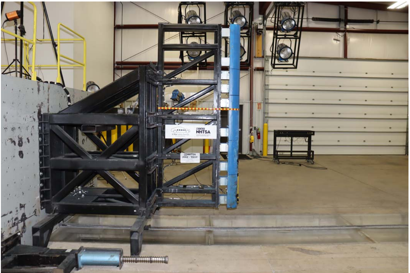
Photo No. 061 - Pre-Test Pole Barrier Side View
