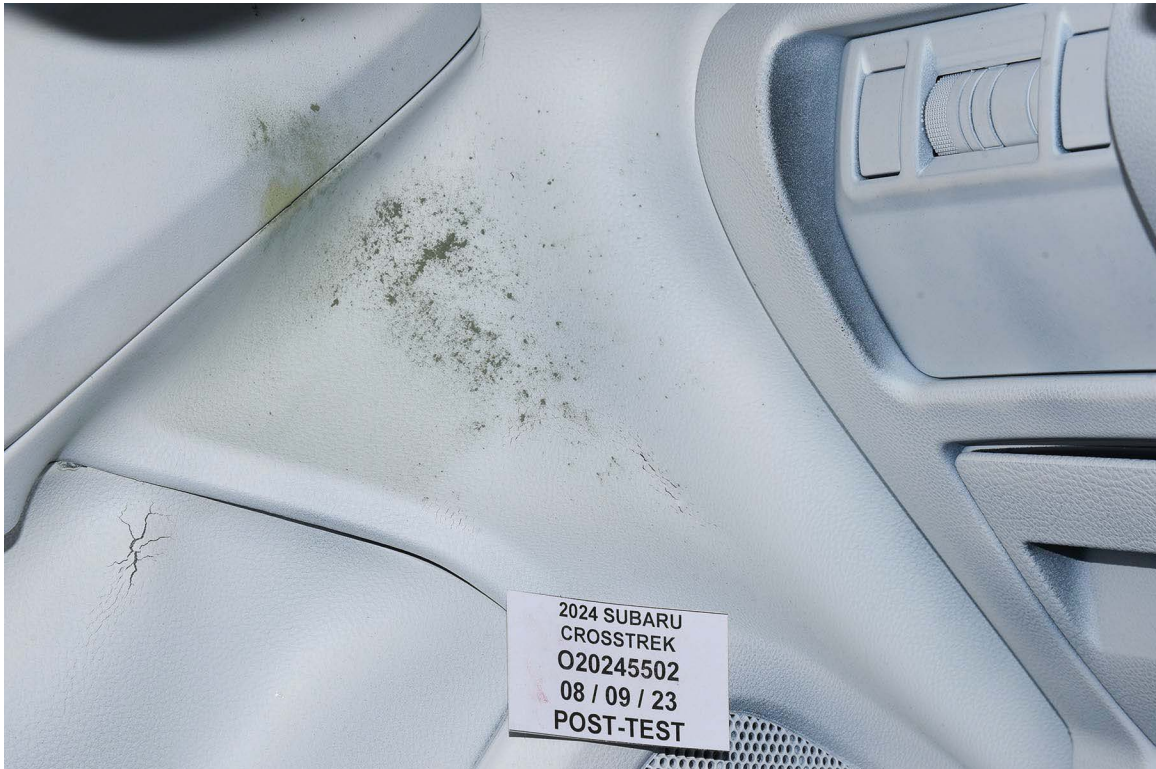
FIGURE 54. Post-Test Driver Dummy Close-Up Knee Contact View
