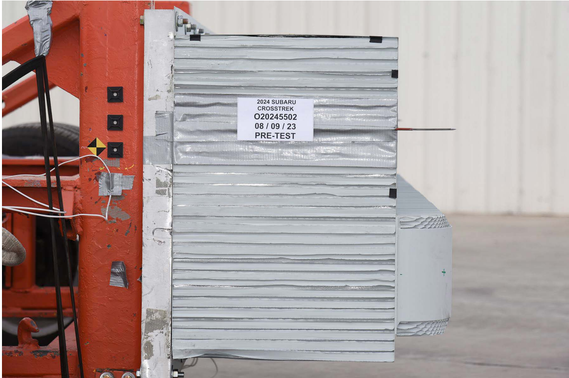
FIGURE 90. Pre-Test Right View of MDB Impactor Face
