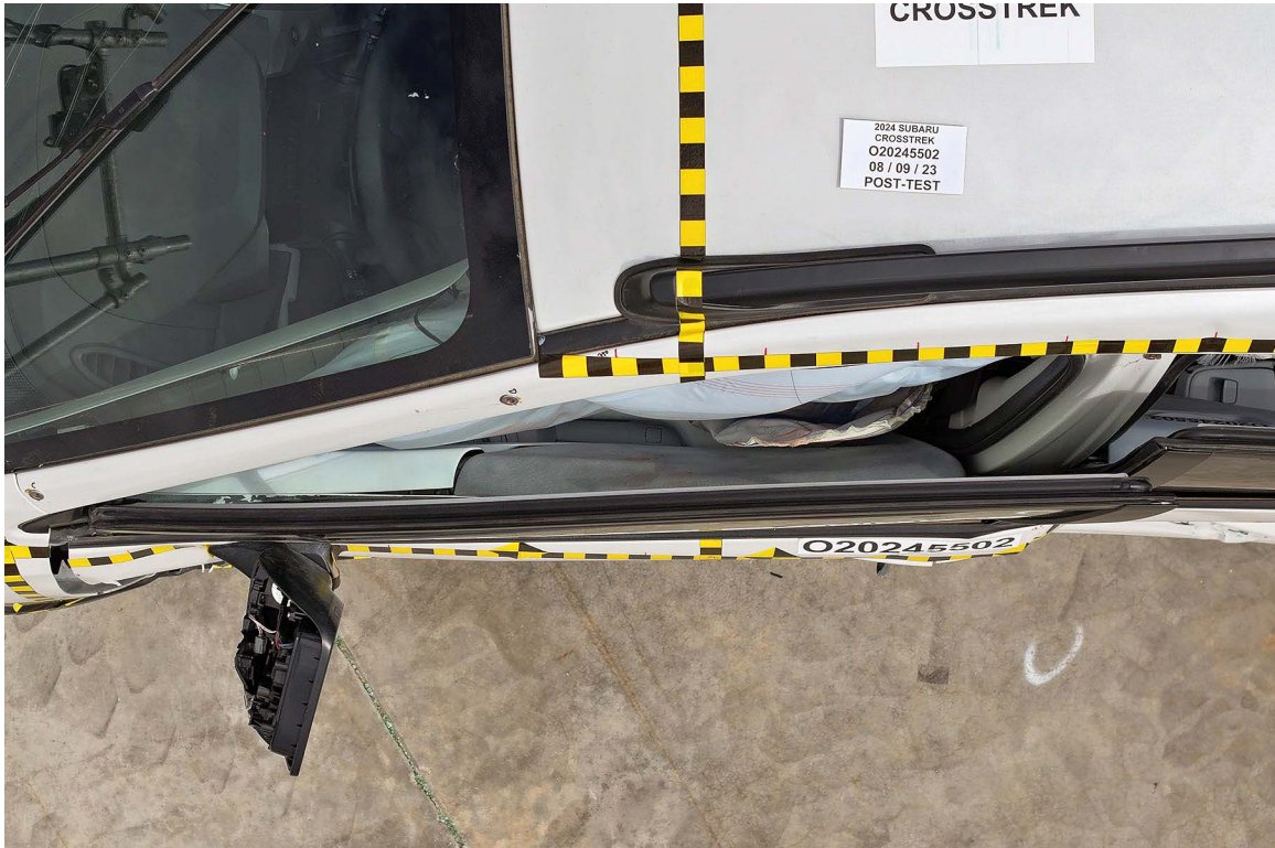
FIGURE 43. Post-Test Driver Dummy and Door Clearance View
