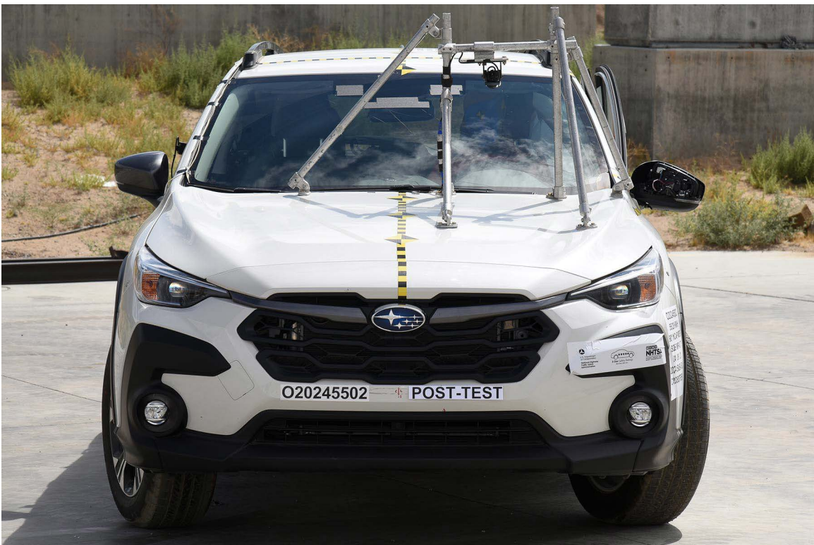
FIGURE 4. Post-Test Frontal View of Test Vehicle
