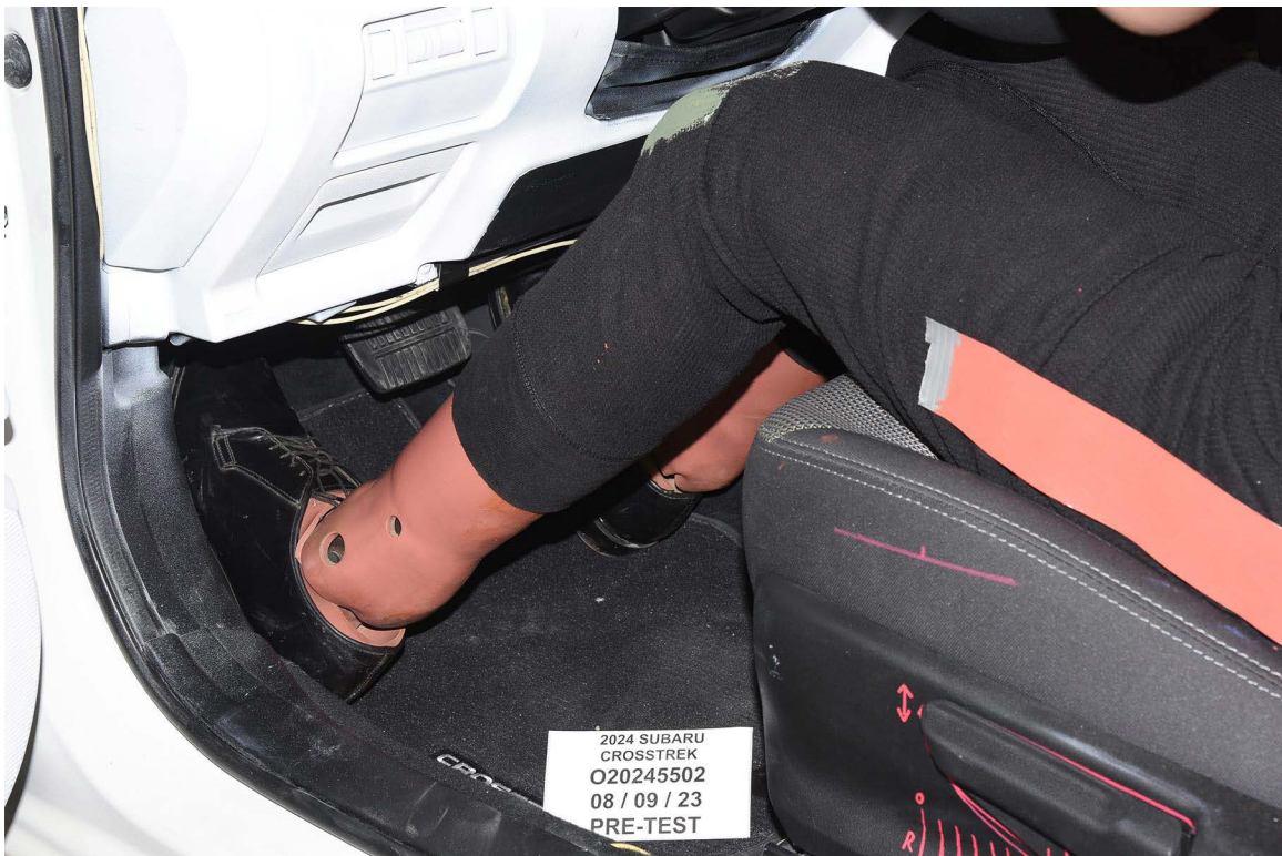
FIGURE 34. Pre-Test Placement of Driver Dummy's Feet
