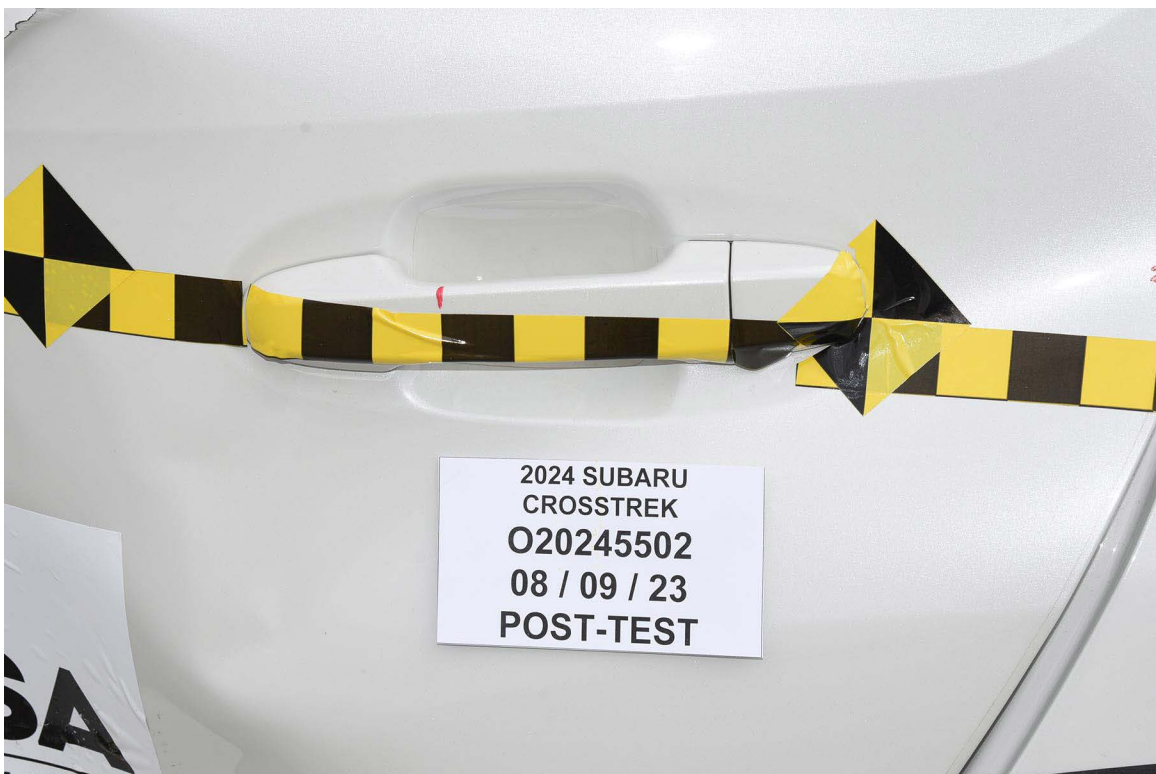
FIGURE 24. Post-Test Left Rear Door Latch Close-Up
