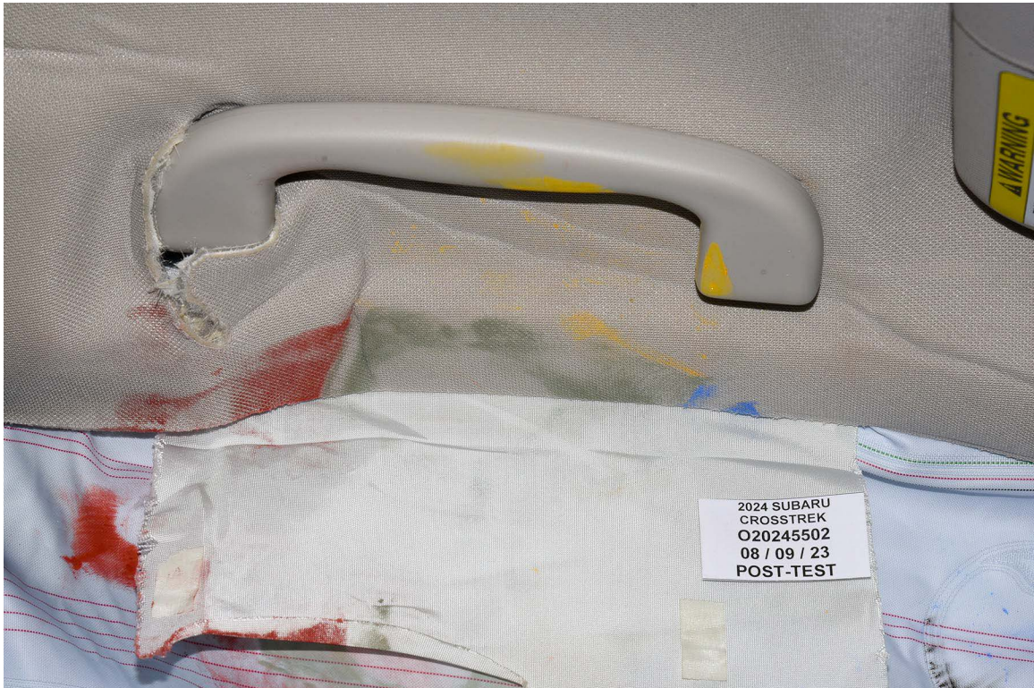
FIGURE 48a. Post-Test Driver Dummy Close-Up Head Contact with Vehicle Interior View
