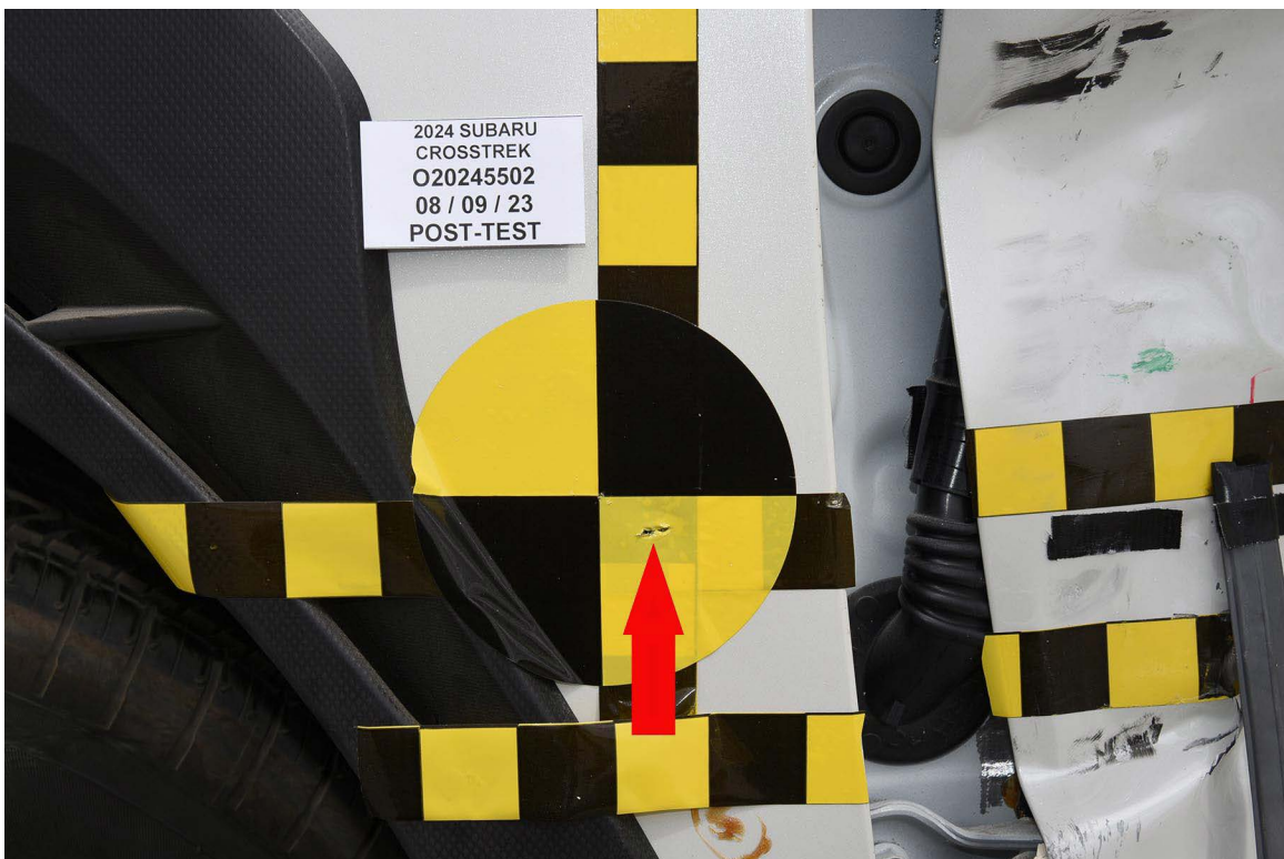
FIGURE 20. Post-Test Close-Up View of Impact Point Target
