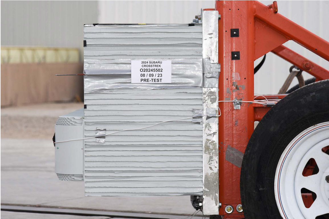
FIGURE 88. Pre-Test Left View of MDB Impactor Face
