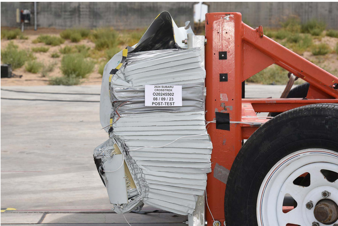
FIGURE 89. Post-Test Left View of MDB Impactor Face
