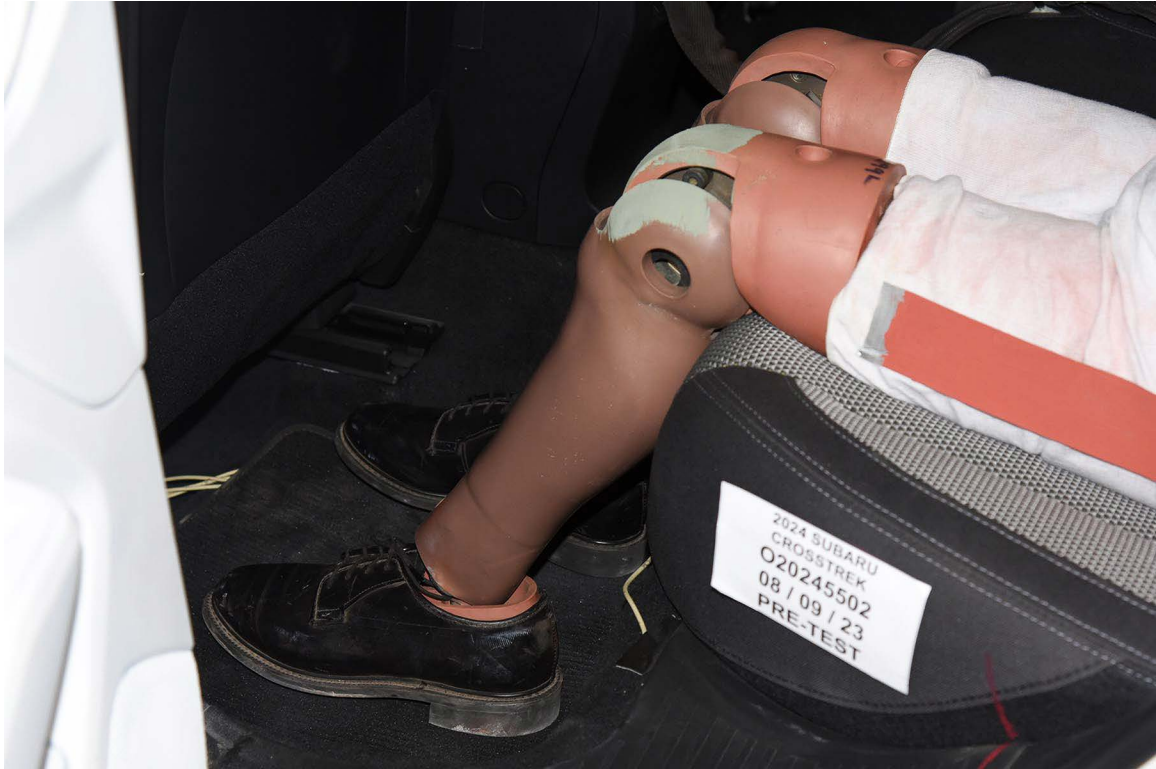
FIGURE 64. Pre-Test Placement of Rear Passenger Dummy's Feet
