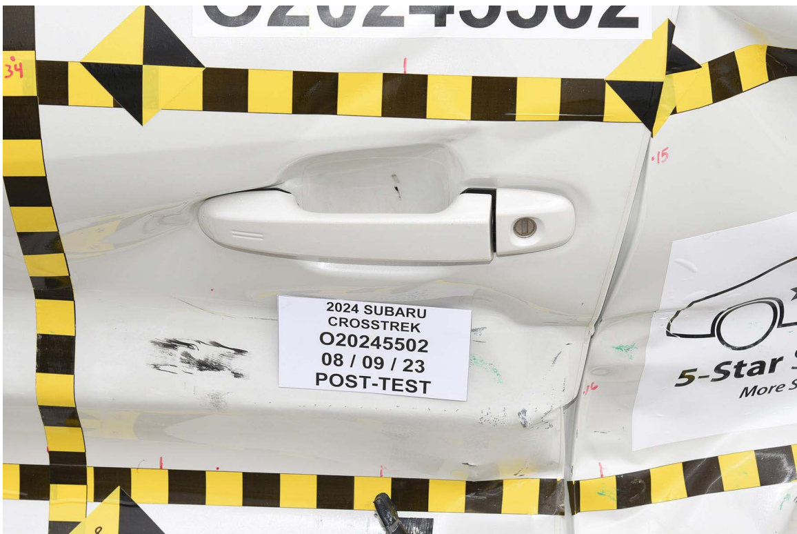
FIGURE 22. Post-Test Left Front Door Latch Close-Up
