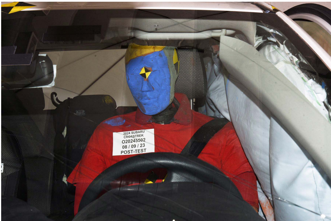
FIGURE 26. Post-Test Front Close-Up View of Driver Dummy
