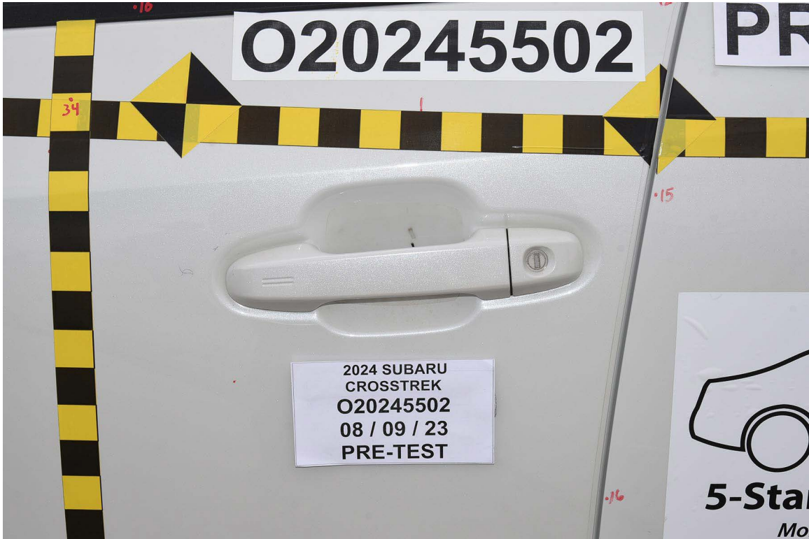
FIGURE 21. Pre-Test Left Front Door Latch Close-Up
