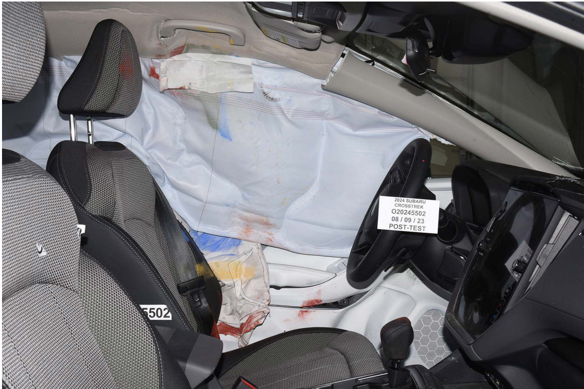
FIGURE 47. Post-Test Driver Inner Door Panel View Showing Driver Dummy Contact Locations
