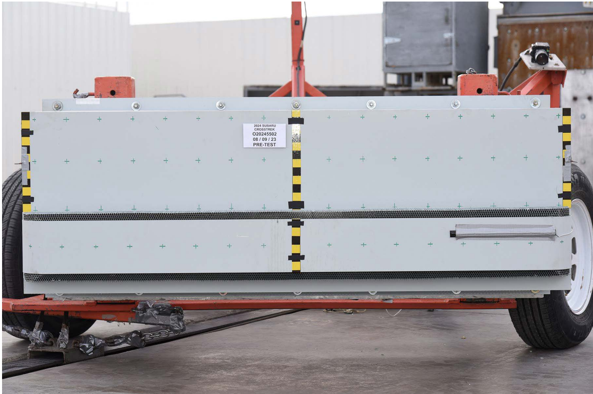
FIGURE 84. Pre-Test Front View of MDB Impactor Face
