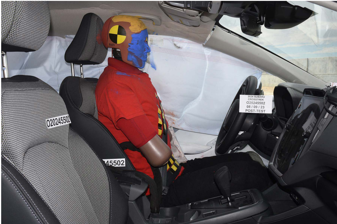
FIGURE 45. Post-Test Right Side View of Driver Dummy and Front Seat of Occupant Compartment
