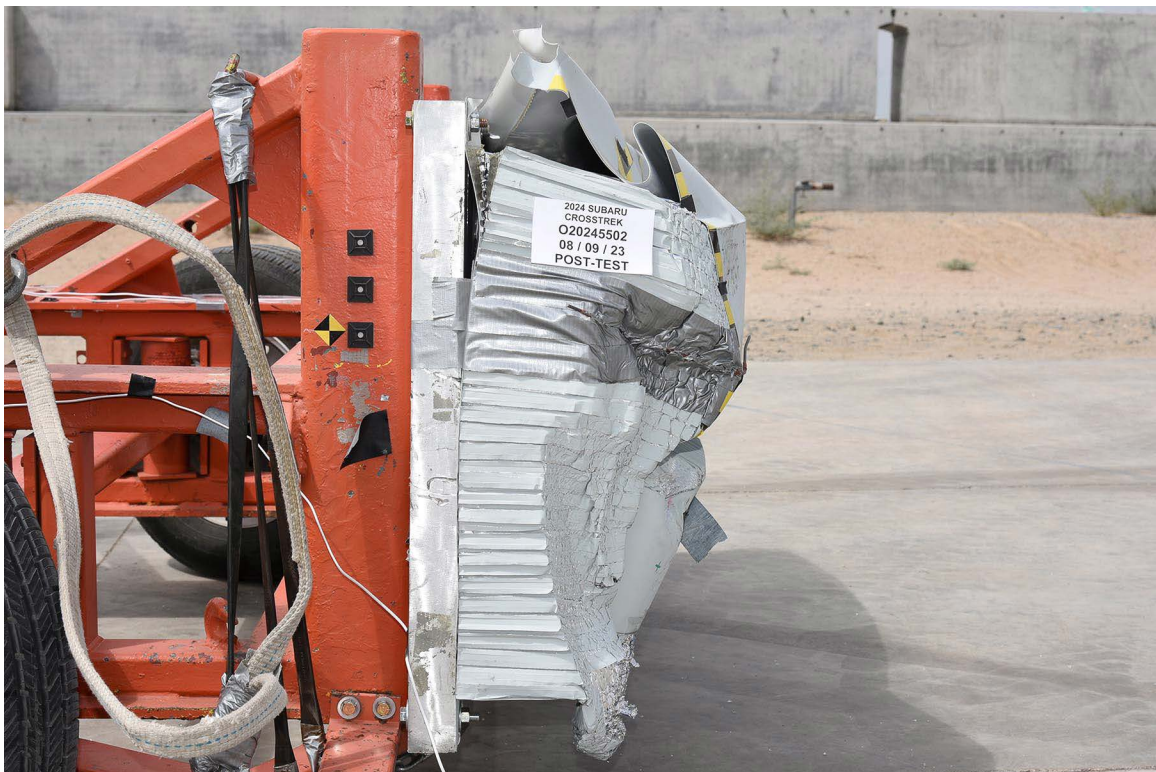
FIGURE 91. Post-Test Right View of MDB Impactor Face
