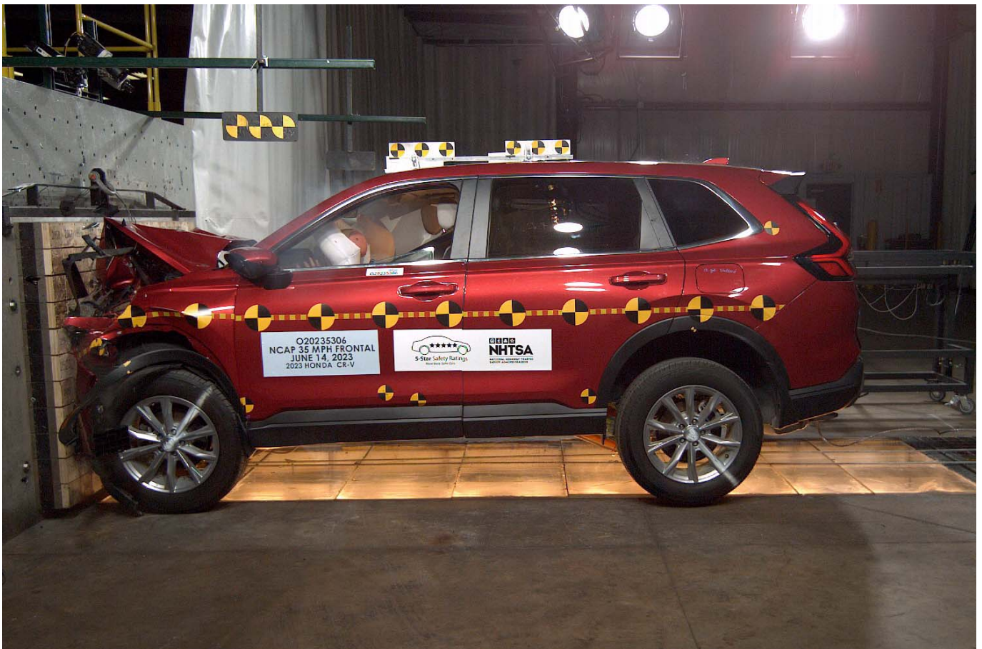
Photo No. 082 - 2023 Honda CR-V AWD EX 5-Door SUV Frontal Impact Event
