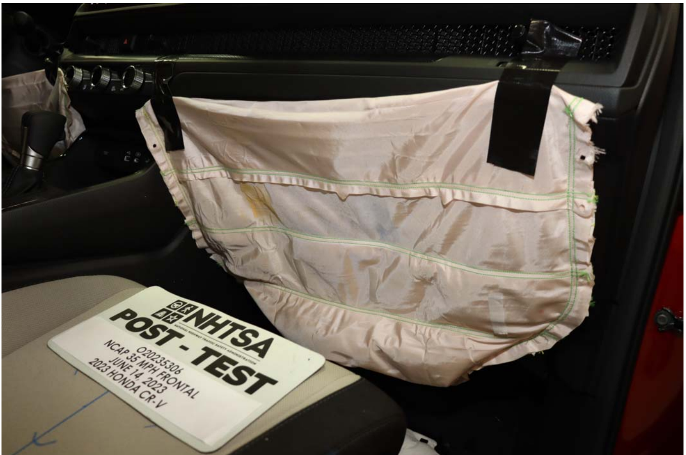
Photo No. 068 - Post-Test Passenger's Side Knee Bolster
