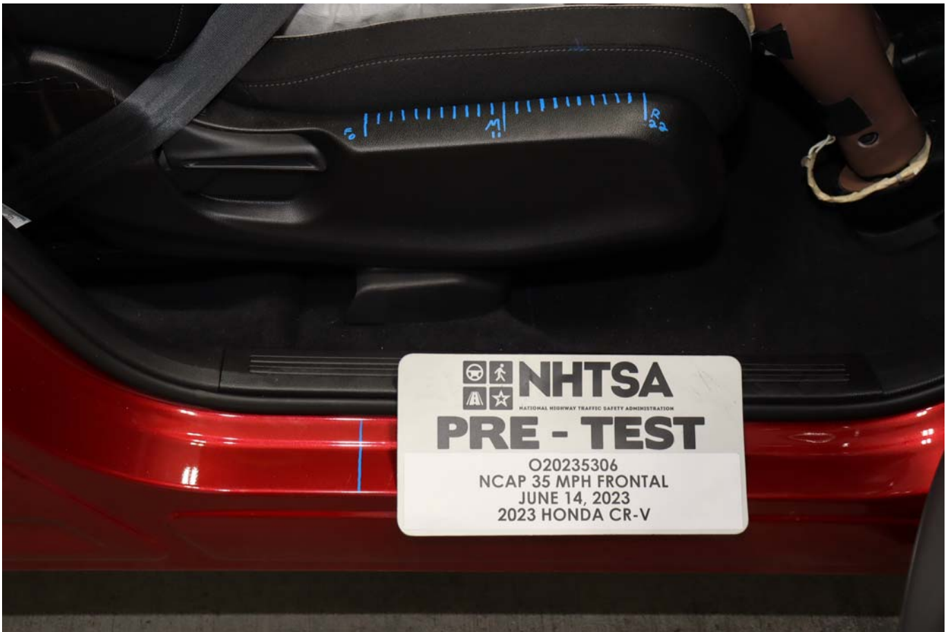
Photo No. 059 - Pre-Test Passenger's Seat Fore-Aft Markings
