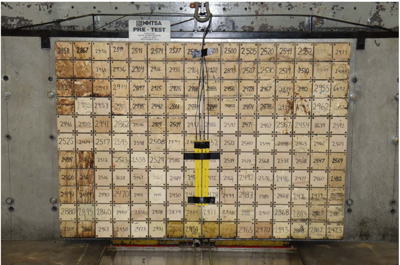
Photo No. 002 - Pre-Test Load Cell Wall
