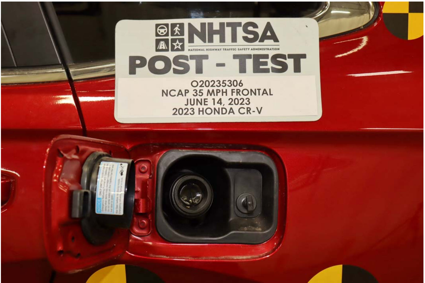
Photo No. 023 - Post-Test Fuel Filler Cap View
