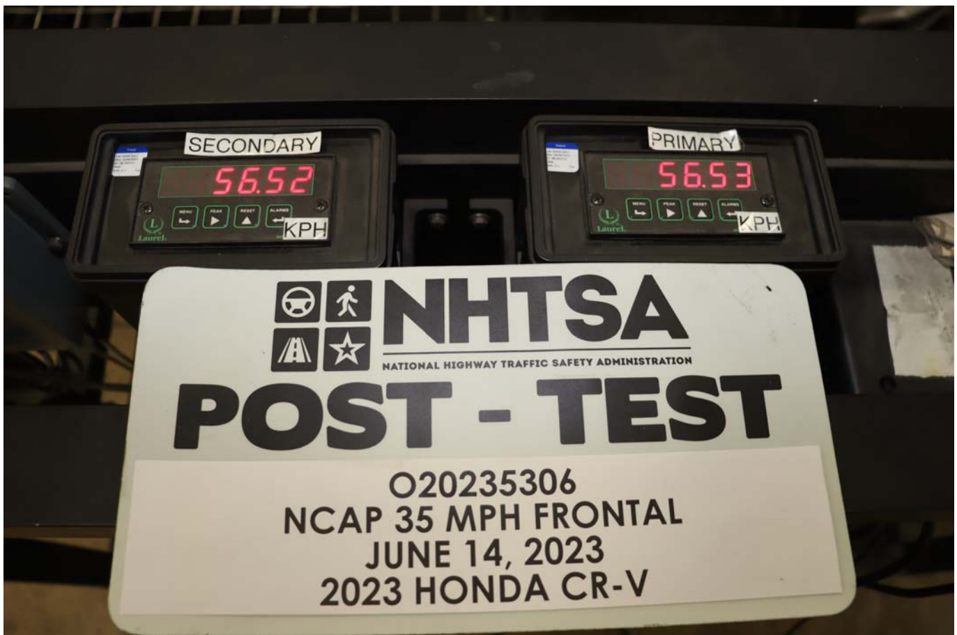
Photo No. 076 - Post-Test Speed Trap Read-Out
