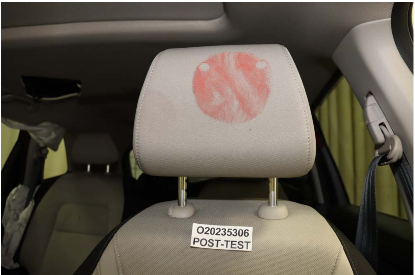
Photo No. 050 - Post-Test Driver Dummy Contact with Headrest
