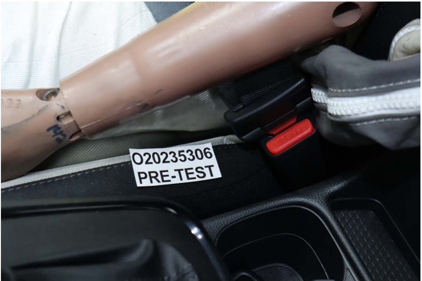
Photo No. 063 - Pre-Test View of Belt Buckle and Latch Plate for Passenger Dummy
