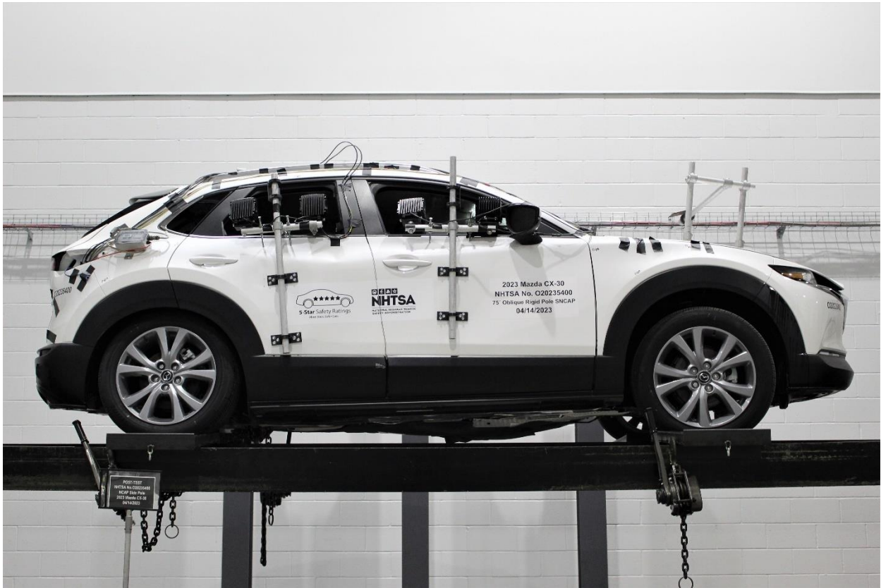
Figure A-69: FMVSS No. 301 Static Rollover 360 Degrees
