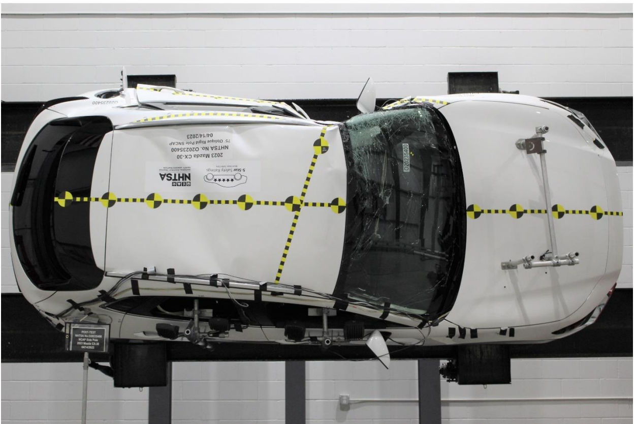
Figure A-68: FMVSS No. 301 Static Rollover 270 Degrees
