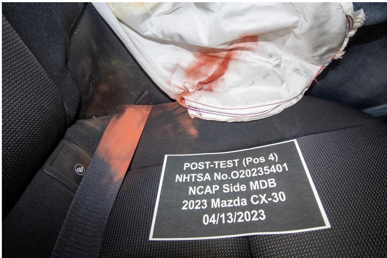
Figure A-80: Post-Test Rear Passenger Dummy Close-Up Pelvis Contact with Side Air bag View
