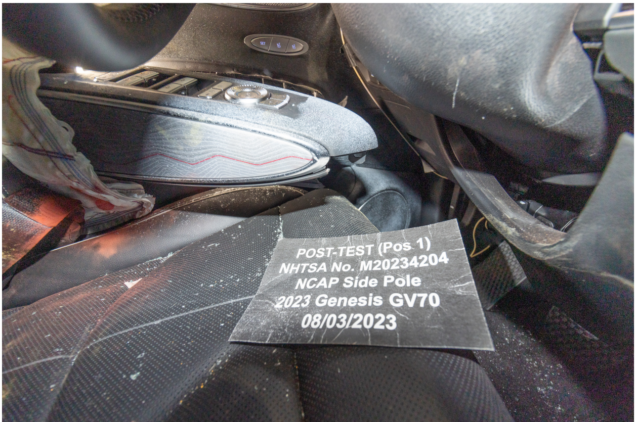
Figure A-52: Post-Test Dummy Close-Up Knee Contact with Vehicle Interior View
