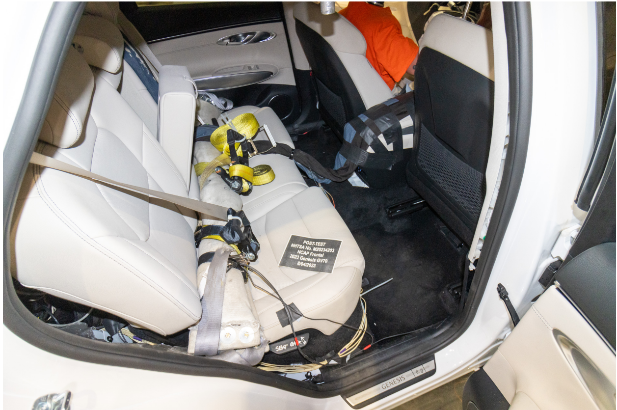
Figure A-29: Post-Test Dummy Cable Routing
