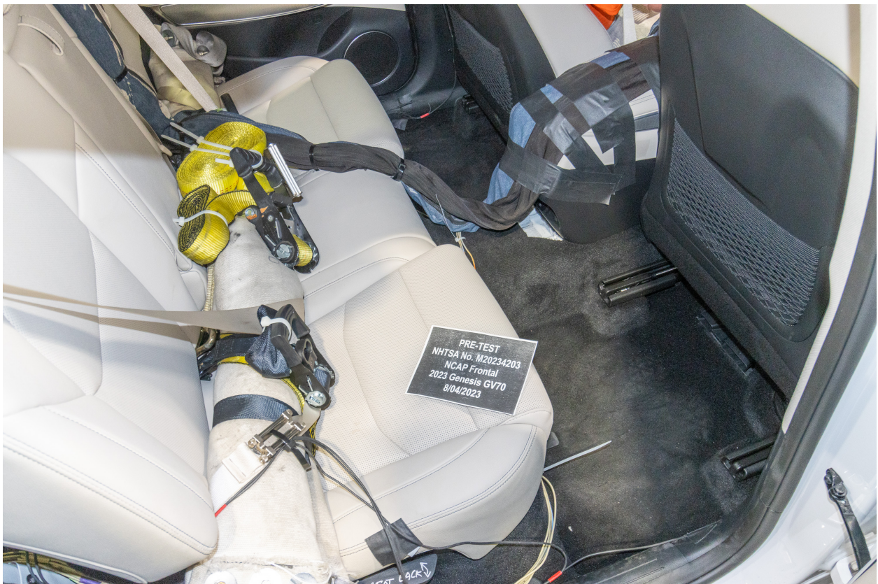
Figure A-28: Pre-Test Dummy Cable Routing
