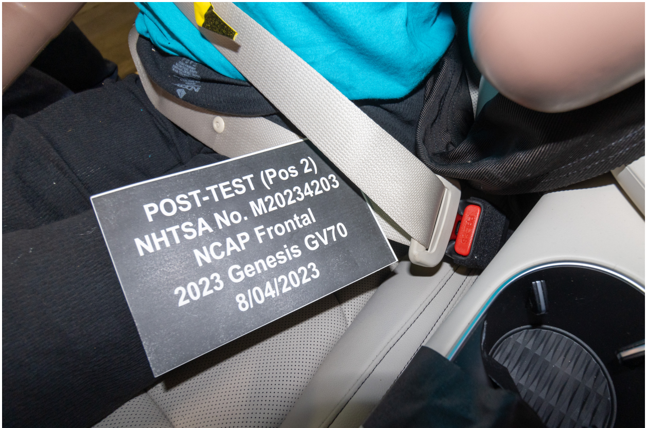
Figure A-64: Post-Test View of Belt Buckle and Latch Plate for Passenger Dummy
