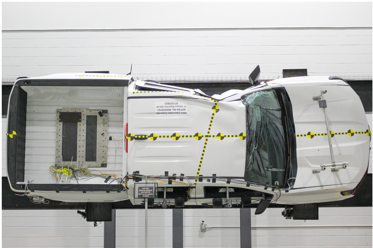
Figure A-68: FMVSS No. 301 Static Rollover 270 Degrees
