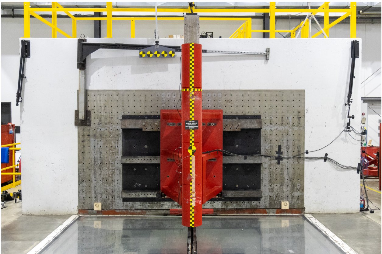
Figure A-60: Post-Test Pole Barrier Front View
