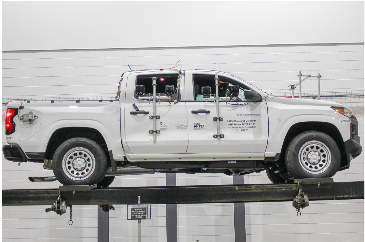
Figure A-65: FMVSS No. 301 Static Rollover 0 Degrees
