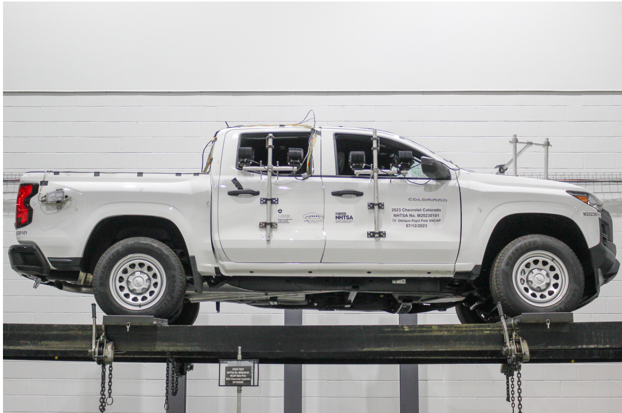
Figure A-69: FMVSS No. 301 Static Rollover 360 Degrees
