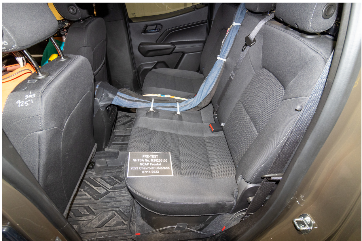
Figure A-28: Pre-Test Dummy Cable Routing
