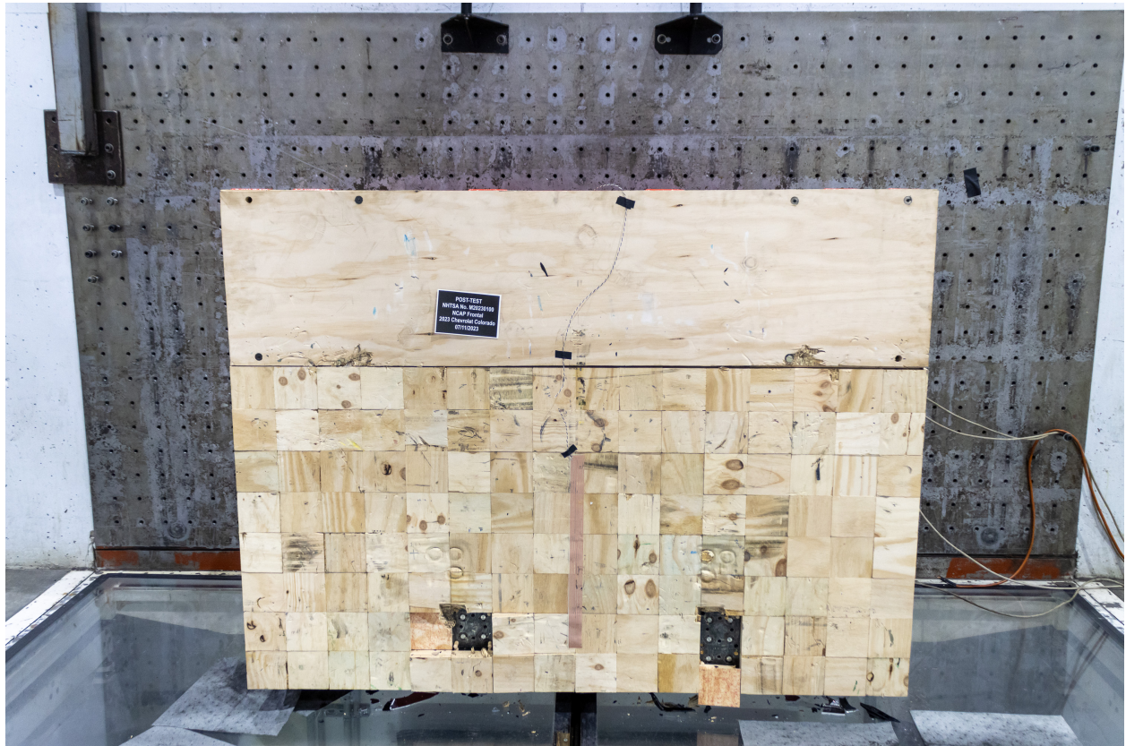
Figure A-3: Post-Test Load Cell Wall
