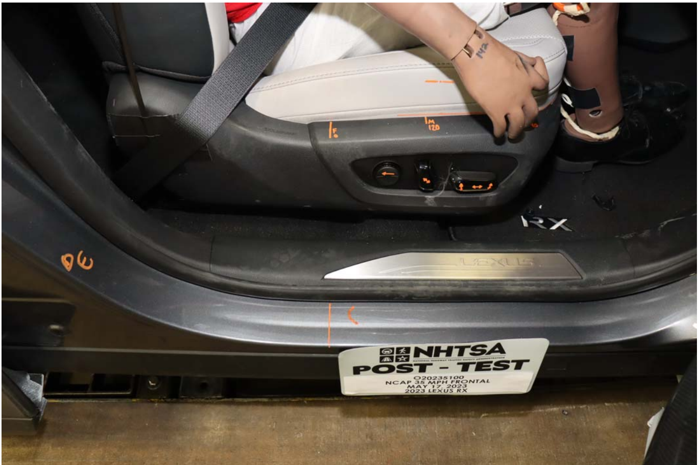
Photo No. 060 - Post-Test Passenger's Seat Fore-Aft Markings
