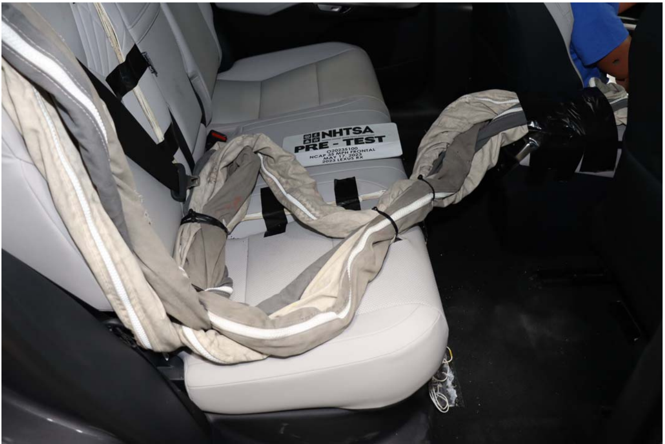
Photo No. 028 - Pre-Test Dummy Cable Routing
