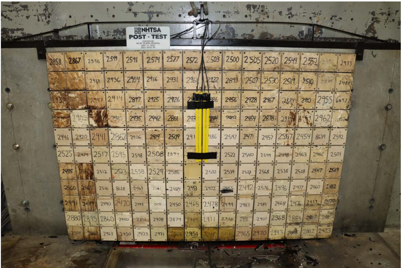
Photo No. 003 - Post-Test Load Cell Wall
