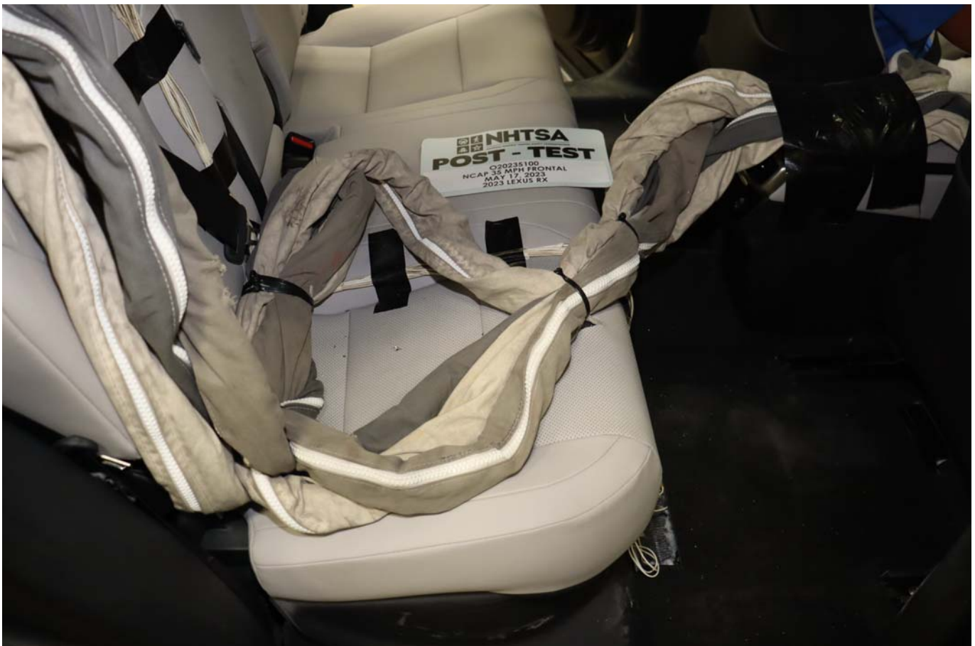
Photo No. 029 - Post-Test Dummy Cable Routing
