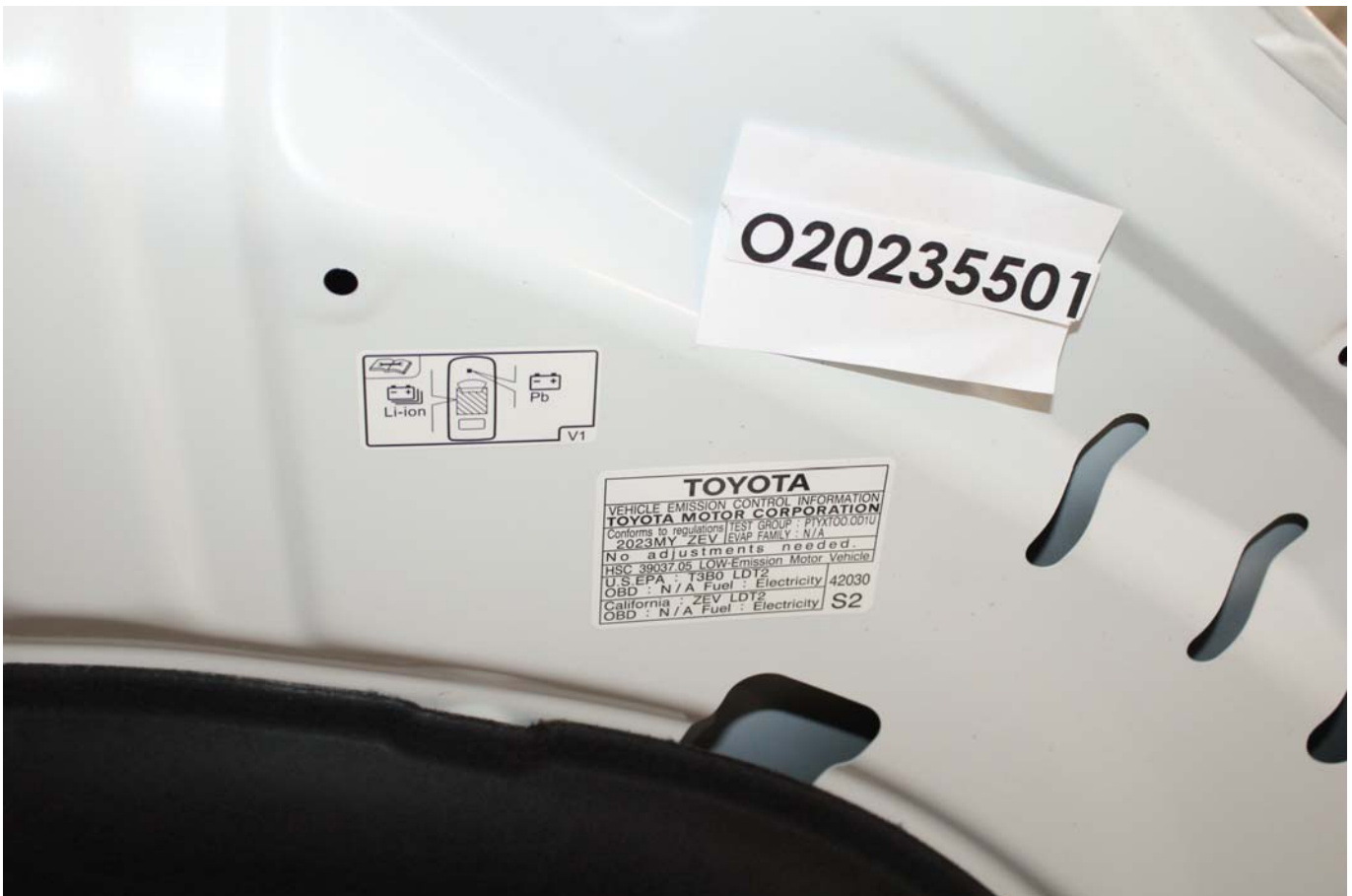
Photo No. 305-03 - First Responder Warning Label
