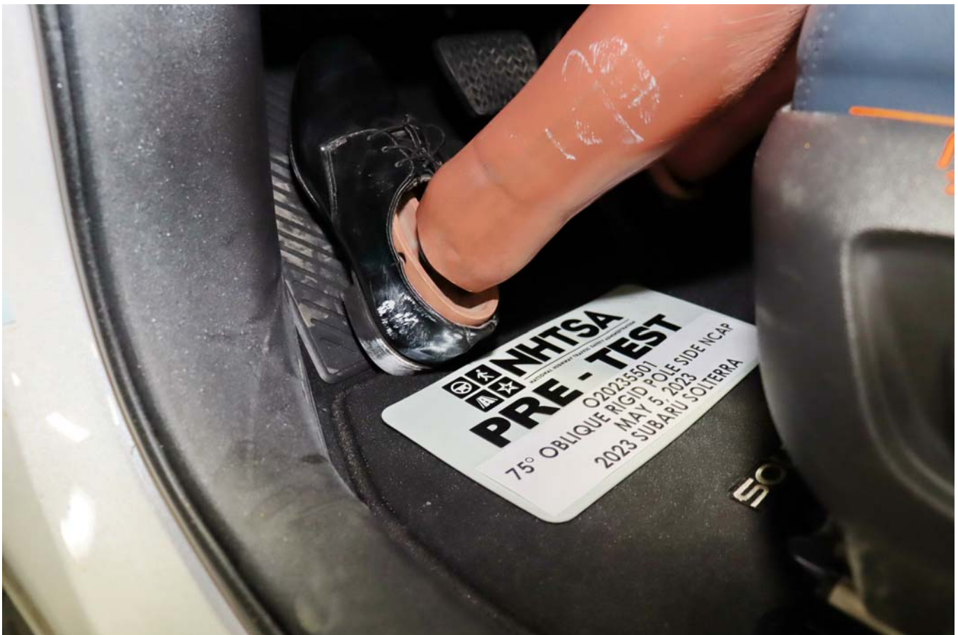
Photo No. 032 - Pre-Test Placement of Dummy's Feet
