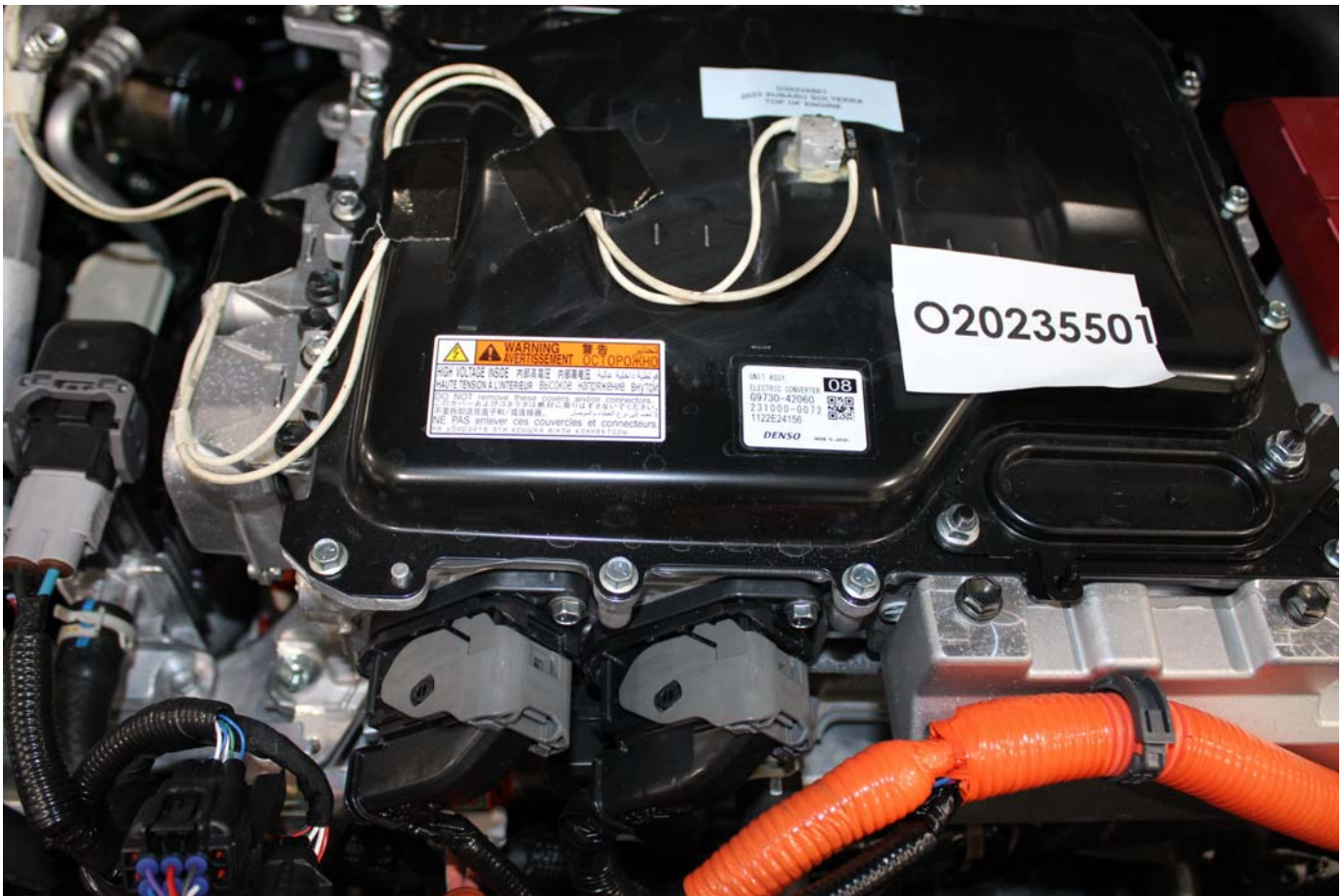
Photo No. 305-02 - Power Inverter Warning Label
