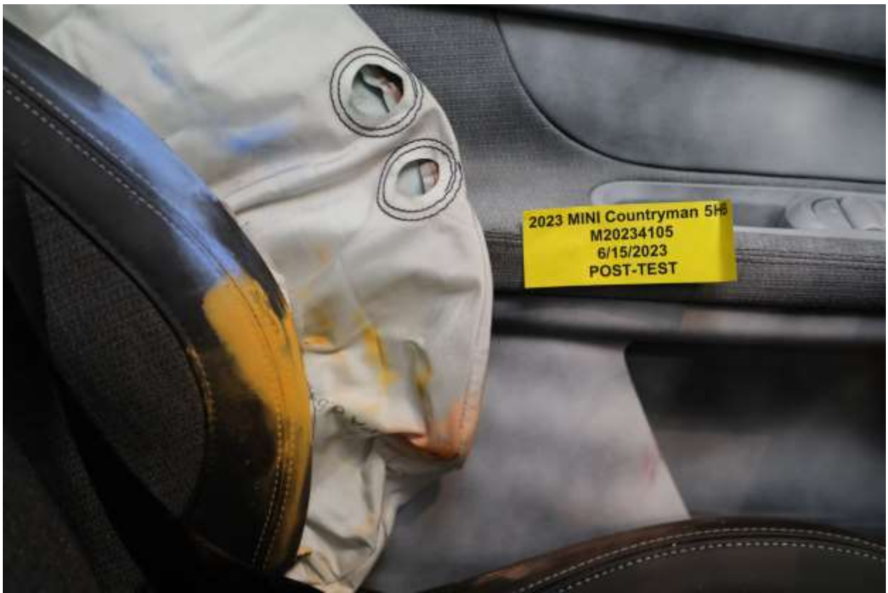
052 Post-Test Driver Dummy Close-Up Pelvis Contact View
