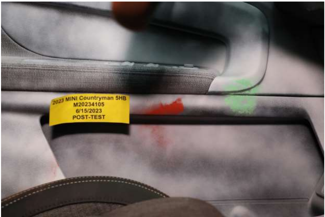
054 Post-Test Driver Dummy Close-Up Knee Contact View
