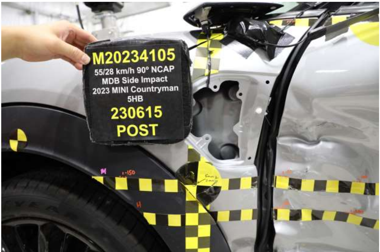
020 Post-Test Close-Up View of Impact Point Target
