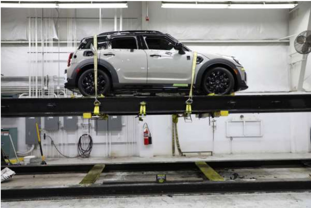
No. 069 FMVSS No. 301 Static Rollover 360 Degrees
