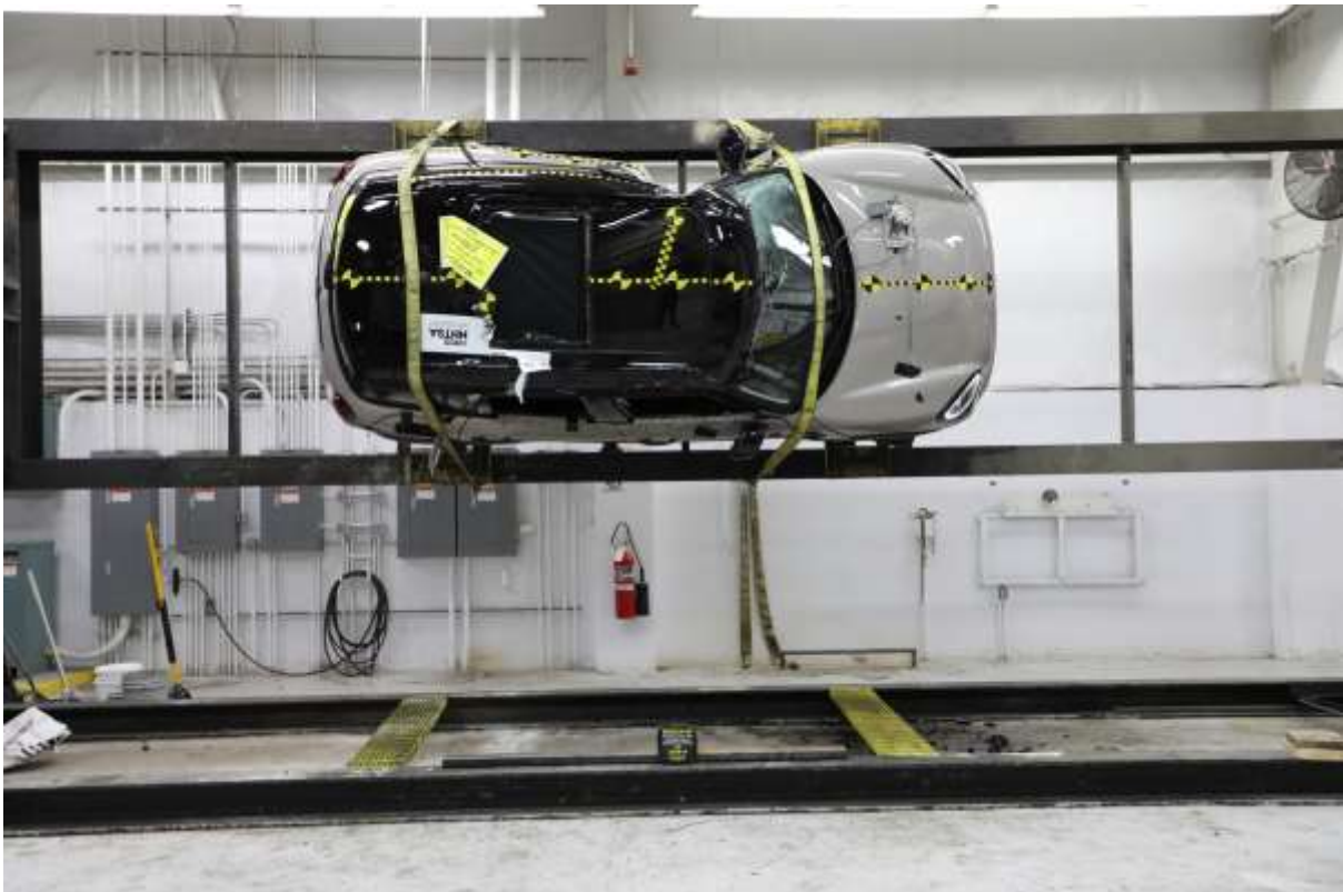
No. 066 FMVSS No. 301 Static Rollover 90 Degrees
