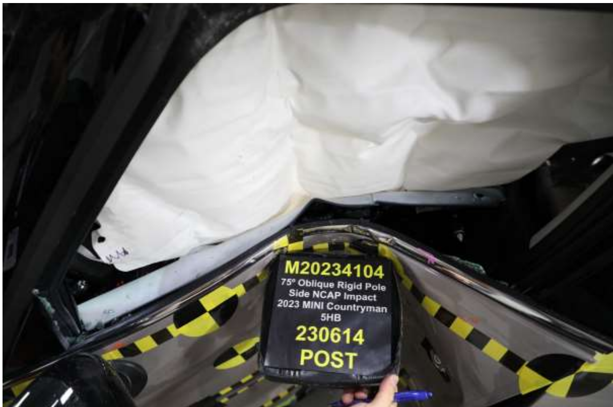
No. 041 Post-Test Dummy and Door Clearance View
