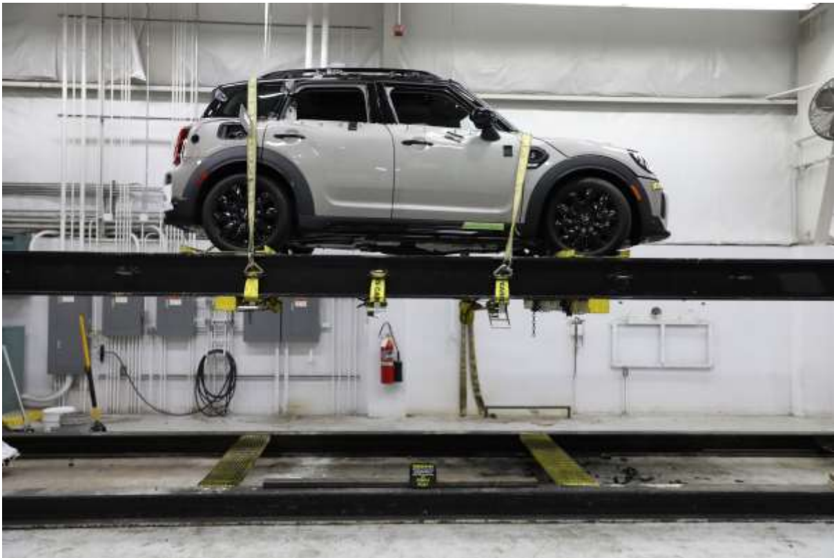
No. 065 FMVSS No. 301 Static Rollover 0 Degrees
