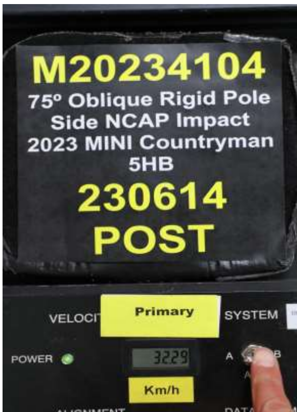
No. 064 Post-Test Primary and Redundant Speed Trap Read Out
