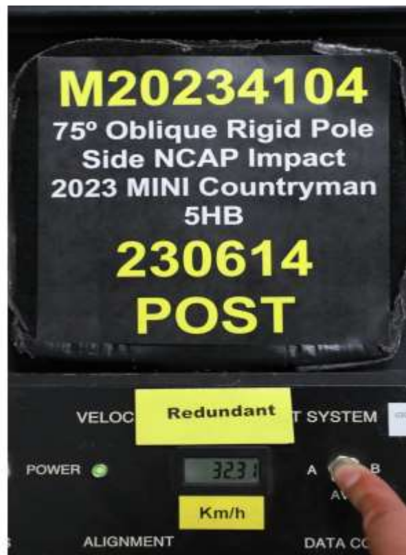
No. 064 Post-Test Primary and Redundant Speed Trap Read Out
