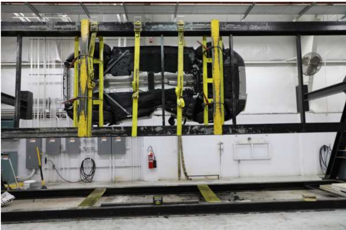
No. 068 FMVSS No. 301 Static Rollover 270 Degrees
