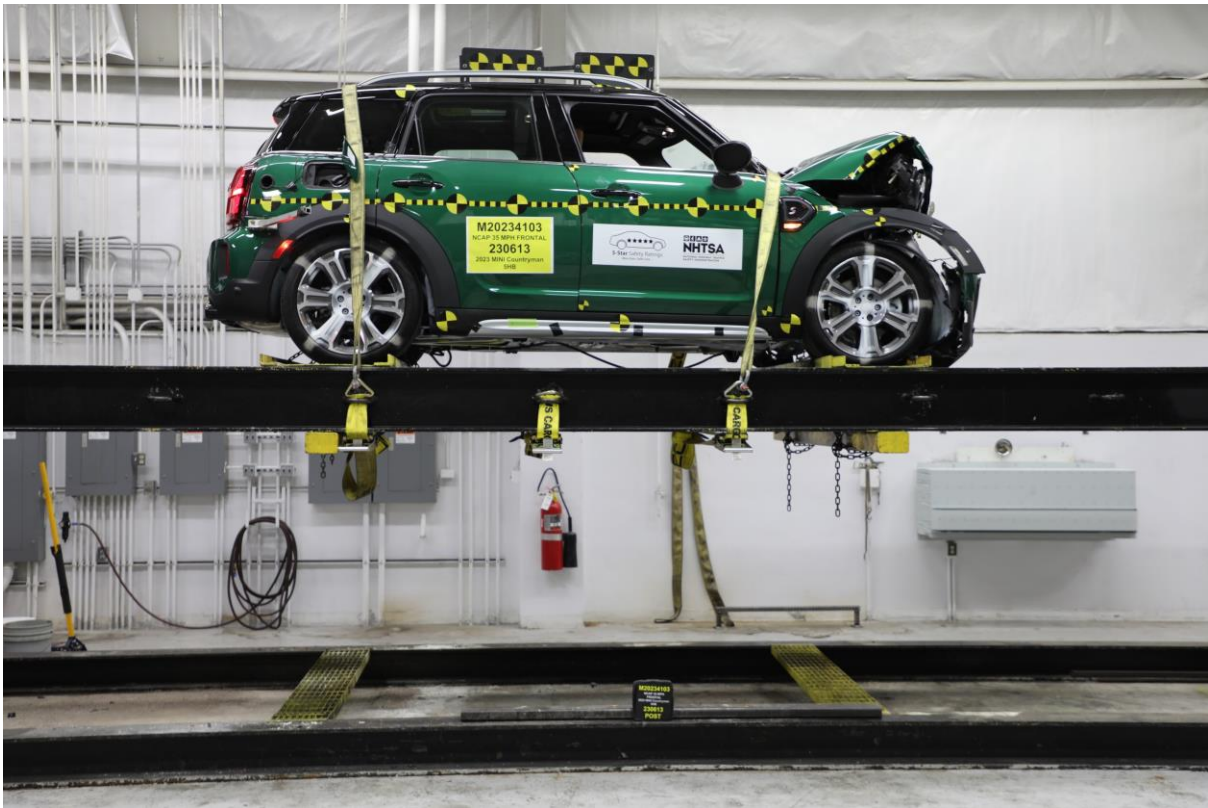
077 Vehicle at 0° on Static Rollover Device
