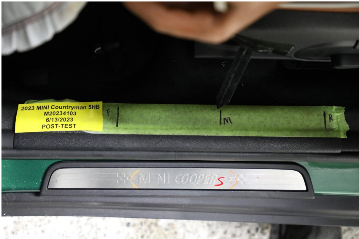
037 Post-Test Driver's Seat Fore-Aft Markings
