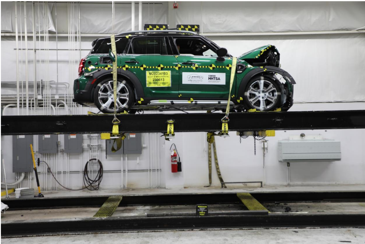
081 Vehicle at 360° on Static Rollover Device
