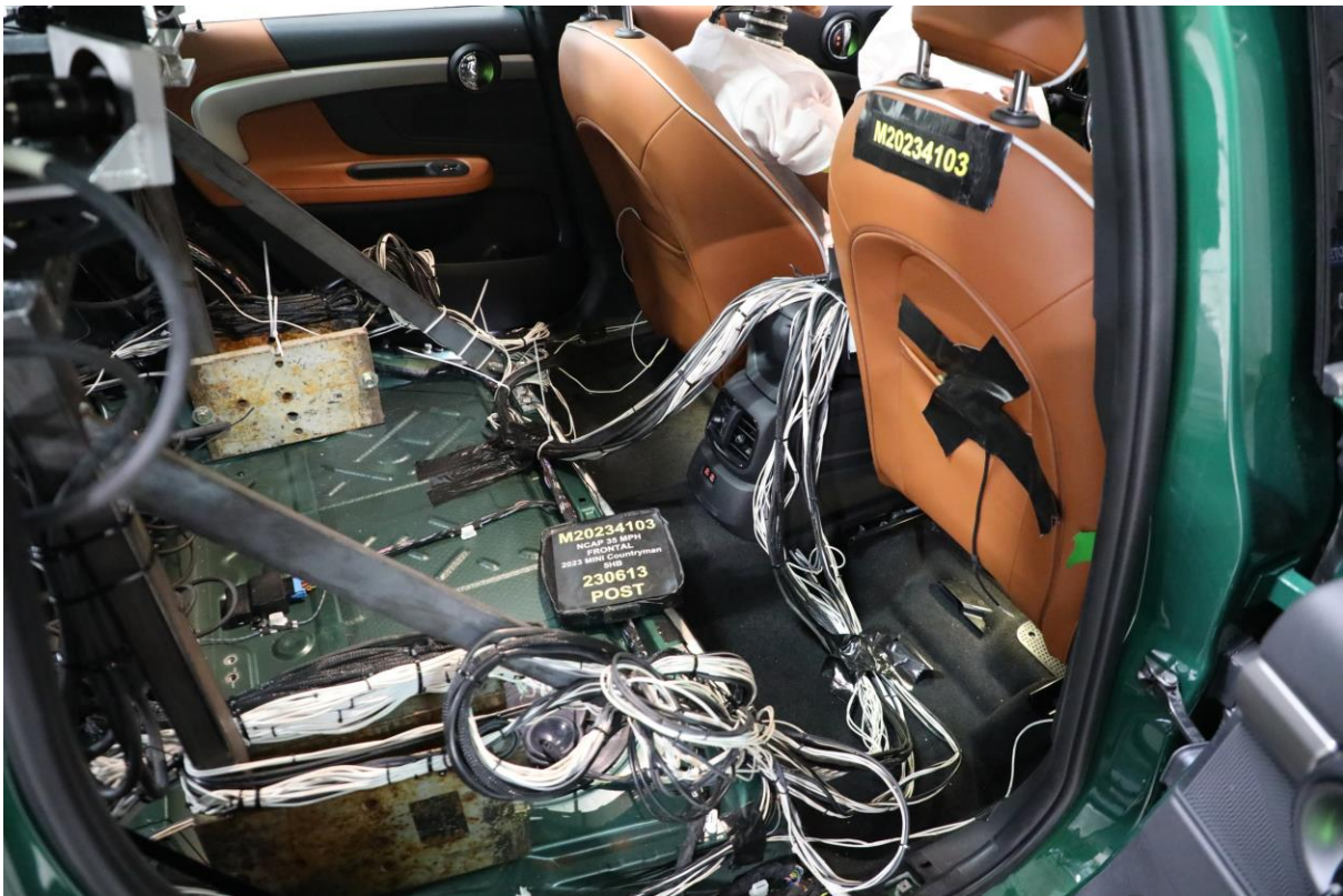
029 Post-Test Dummy Cable Routing
