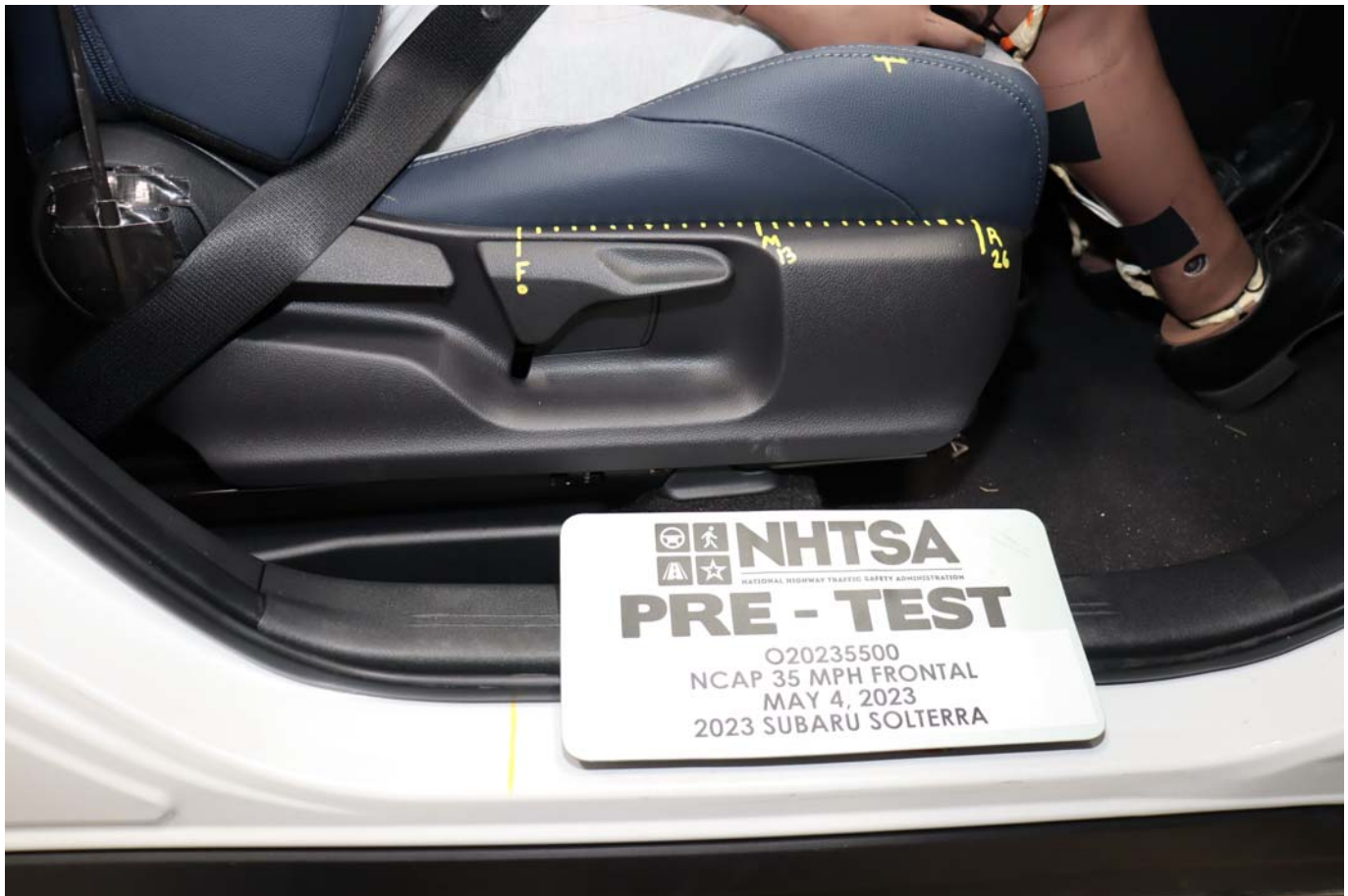
Photo No. 059 - Pre-Test Passenger's Seat Fore-Aft Markings
