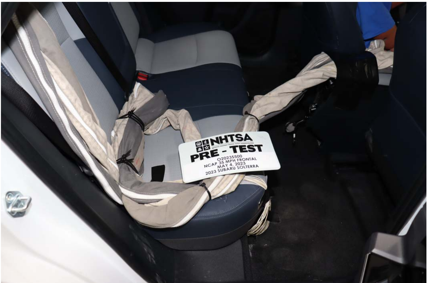
Photo No. 028 - Pre-Test Dummy Cable Routing
