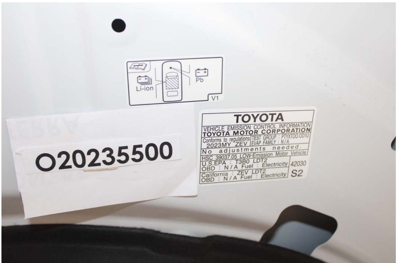
Photo No. 305-03 - First Responder Warning Label
