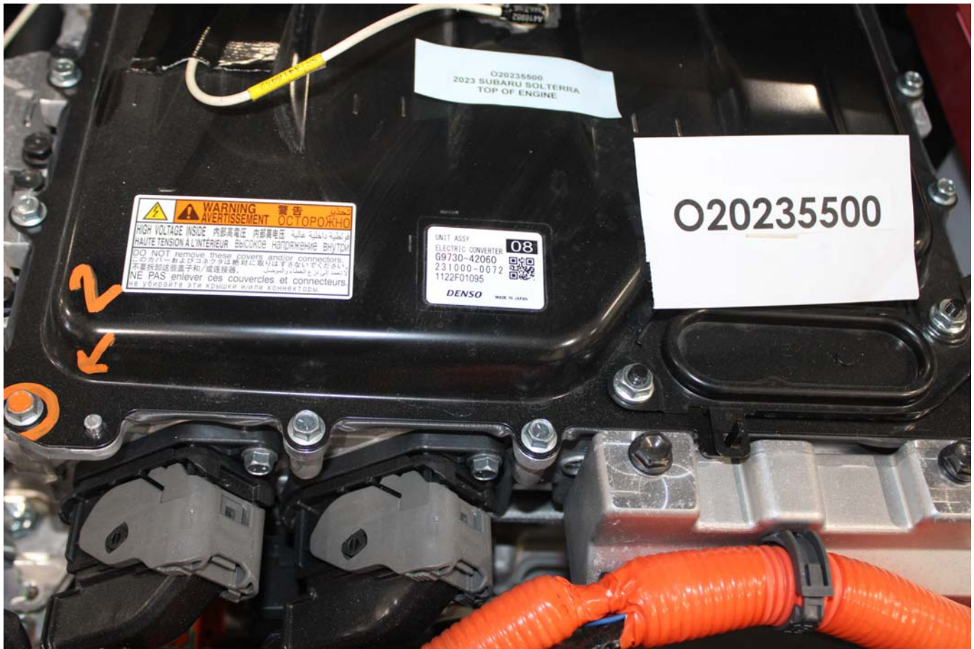
Photo No. 305-02 - Power Inverter Warning Label
