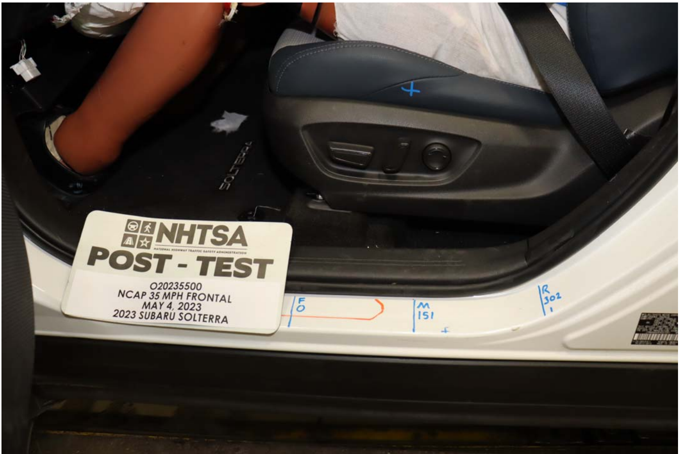
Photo No. 037 - Post-Test Driver's Seat Fore-Aft Markings
