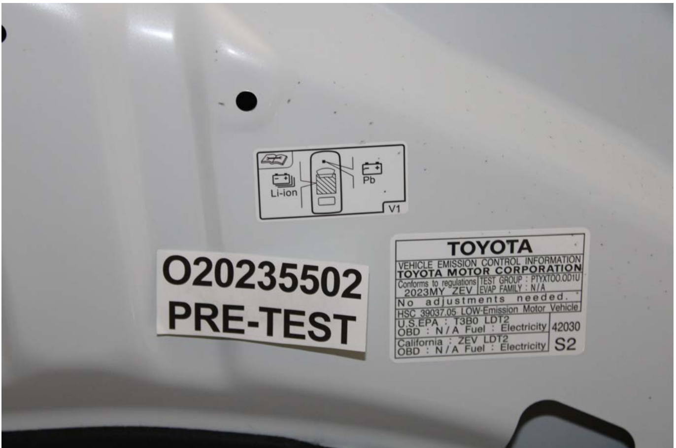
Photo No. 305-03 - First Responder Warning Label
