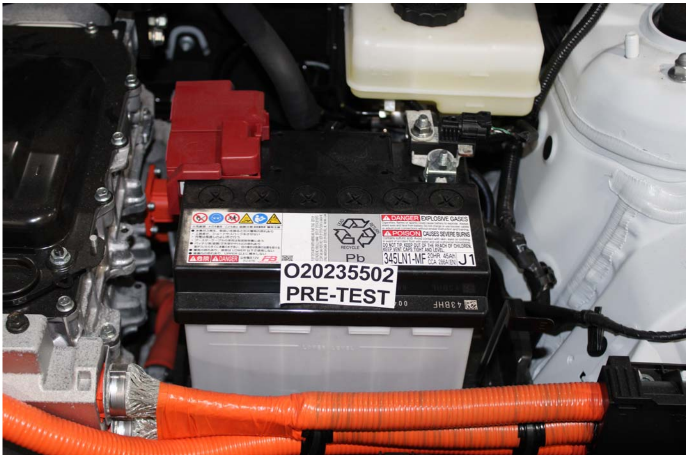
Photo No. 305-01 - Auxiliary Power Module Warning Label
