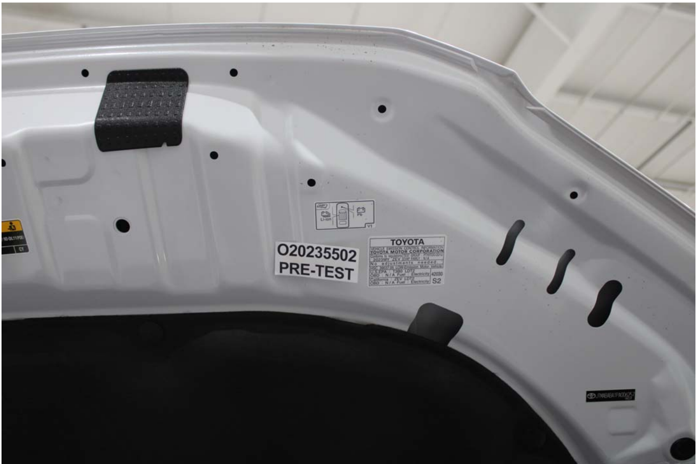
Photo No. 305-04 - First Responder Warning Location
