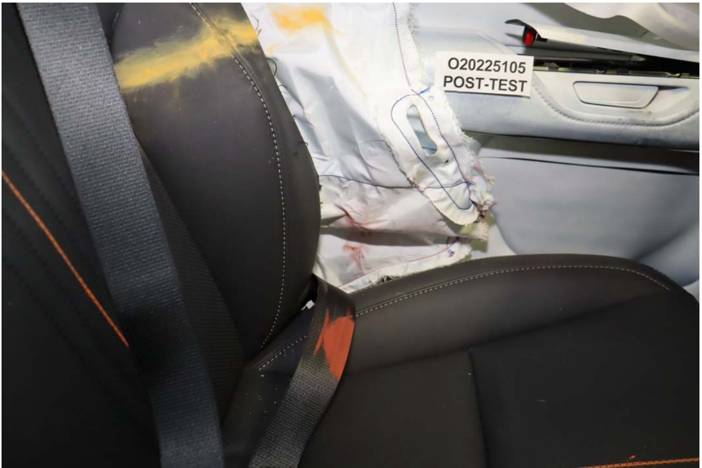
Photo No. 053 - Post-Test Driver Dummy Close-up Pelvis Contact with Side Airbag View
