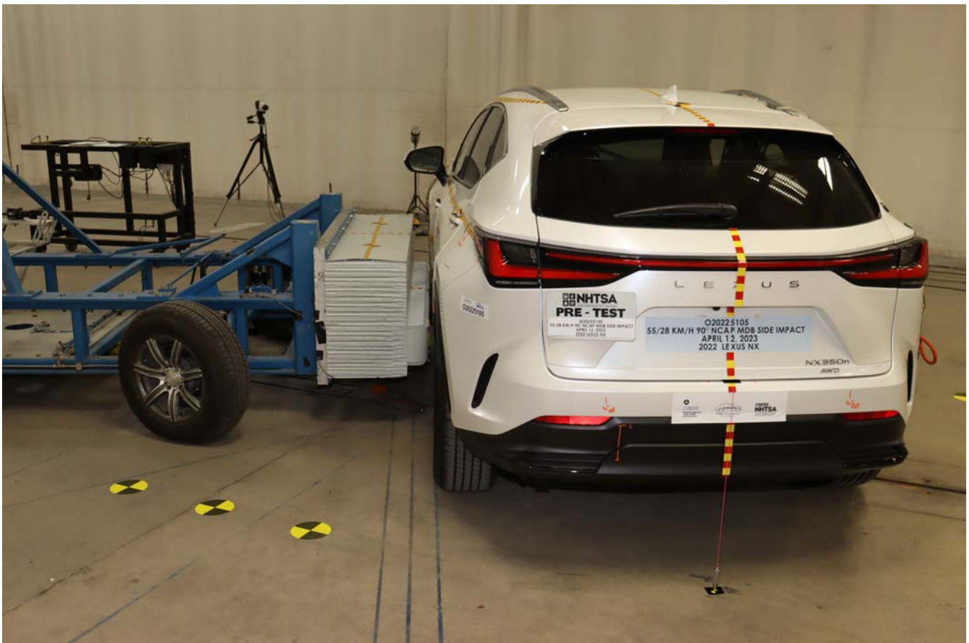
Photo No. 018 - Pre-Test Right Side View of MDB Positioned Against Side of Test Vehicle
