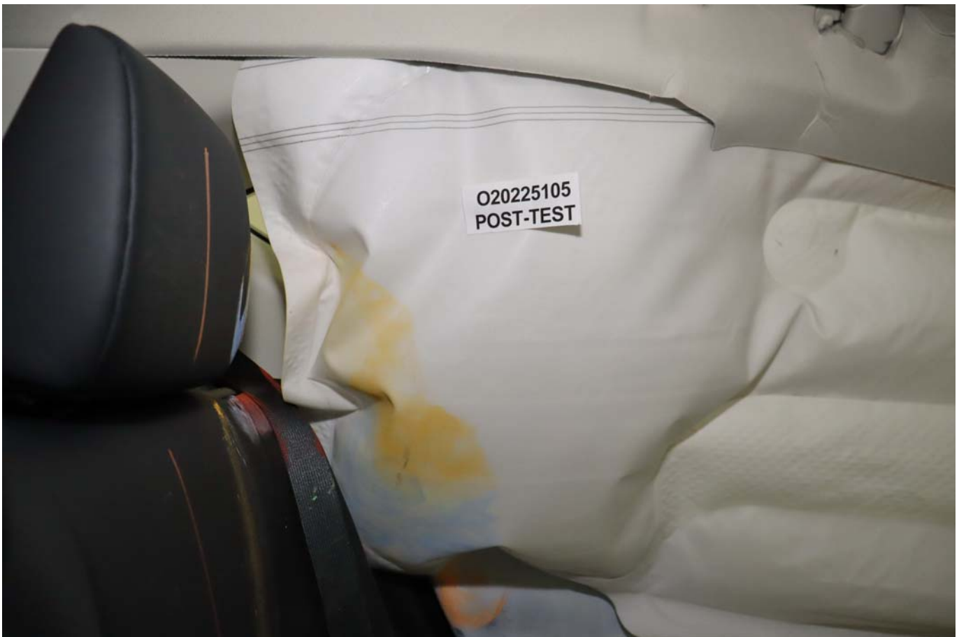
Photo No. 076 - Post-Test Rear Passenger Dummy Close-up Head Contact with Side Airbag View
