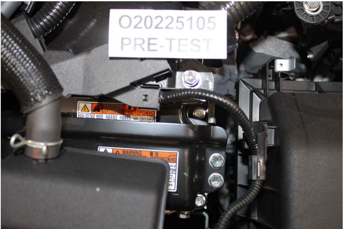
Photo No. 305-02 - Power Inverter Warning Label
