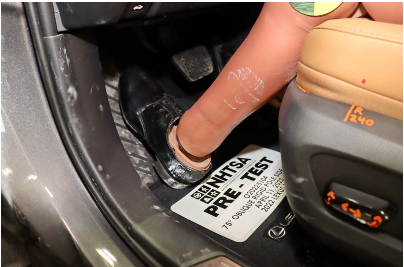
Photo No. 032 - Pre-Test Placement of Dummy's Feet
