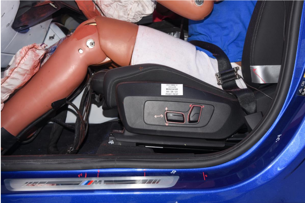
FIGURE 37. Post-Test Driver's Seat Fore-Aft Markings
