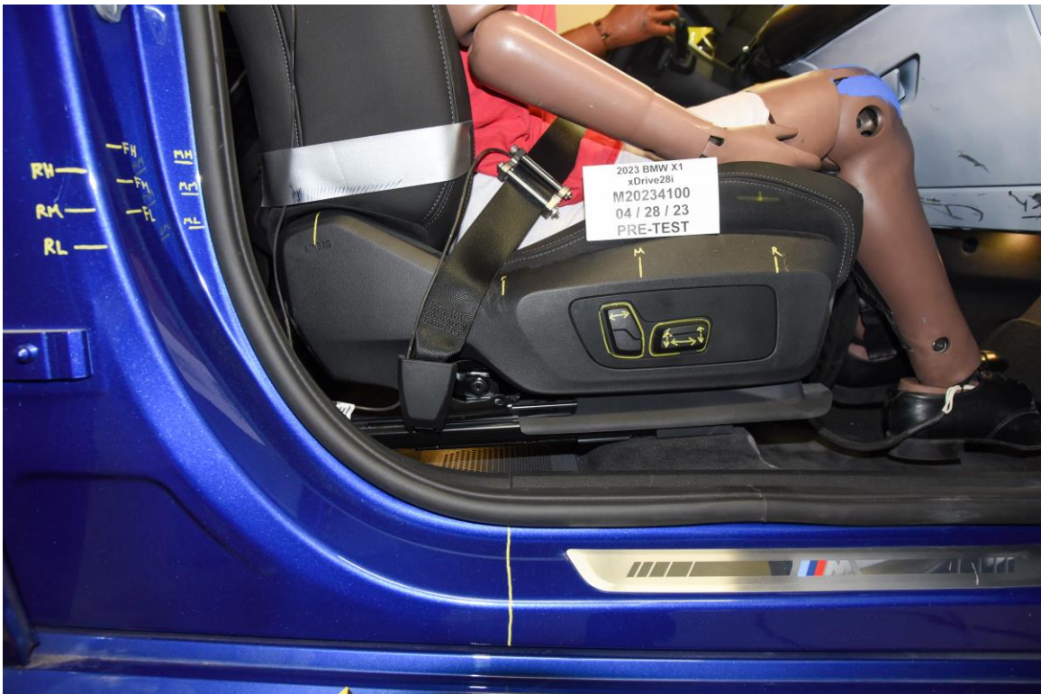
FIGURE 59. Pre-Test Passenger's Seat Fore-Aft Markings
