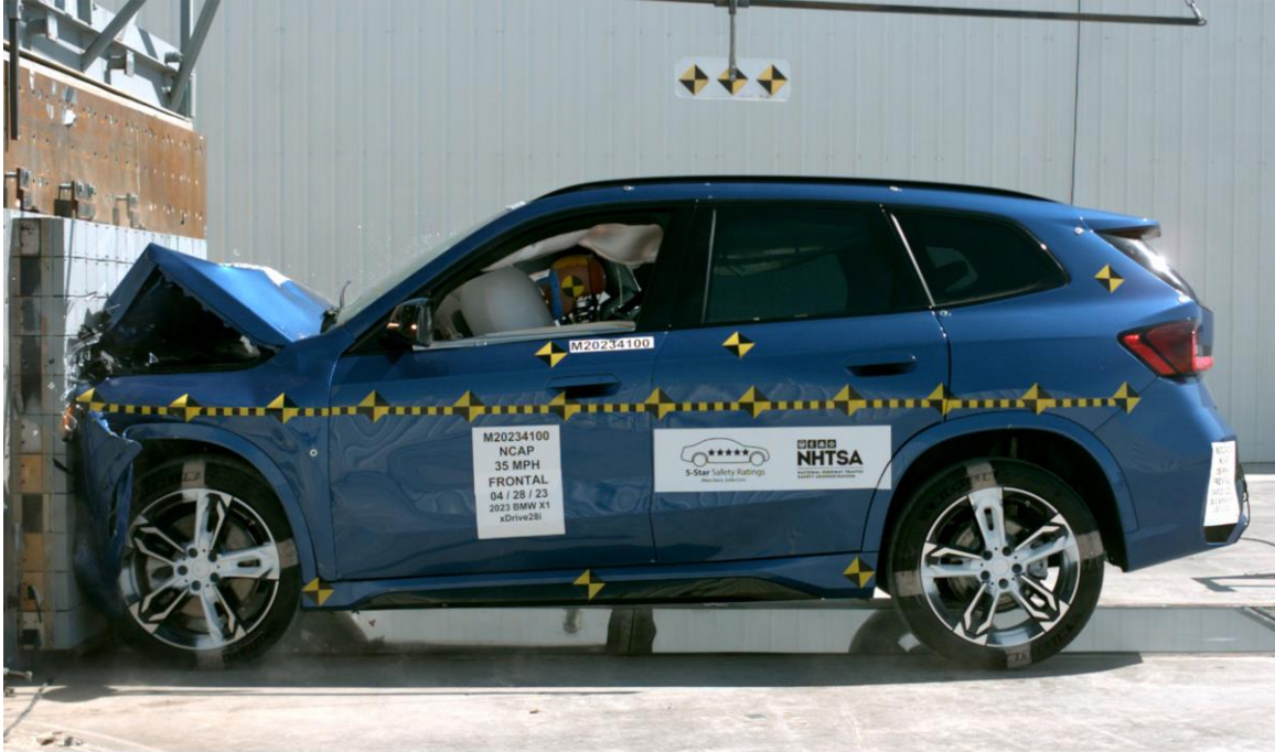
FIGURE 82. 2023 BMW X1 xDrive28i 5-Door SUV Impact Event
