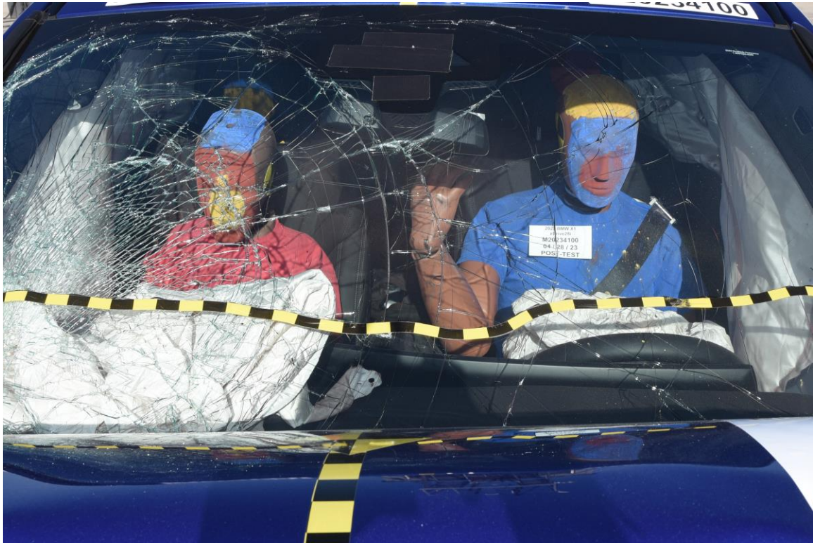
FIGURE 19. Post-Test Windshield View
