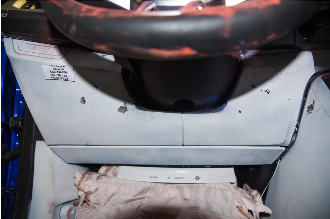
FIGURE 45. Post-Test Driver's Side Knee Bolster
