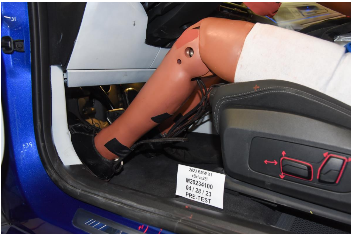
FIGURE 42. Pre-Test Driver Dummy Feet
