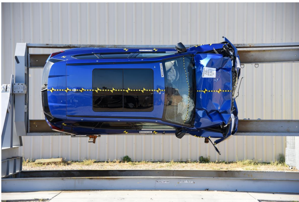
FIGURE 78. Vehicle at 90° on Static Rollover Device
