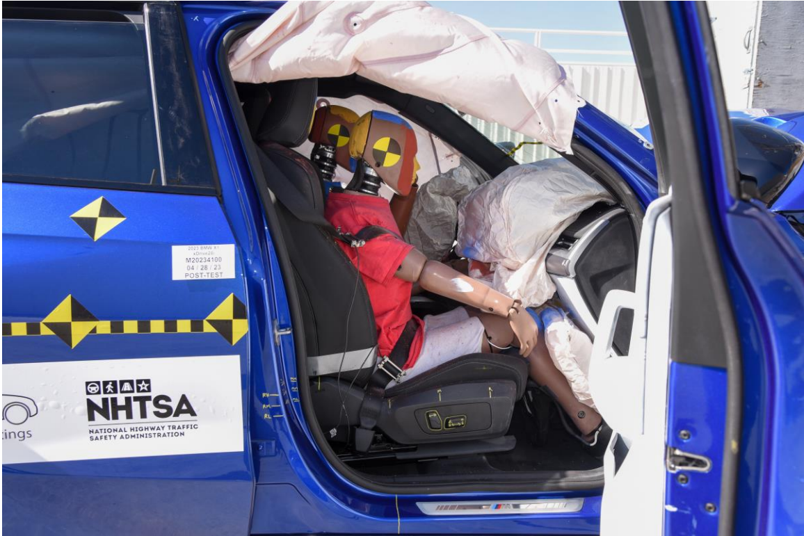
FIGURE 58. Post-Test Passenger Dummy and Vehicle Interior View
