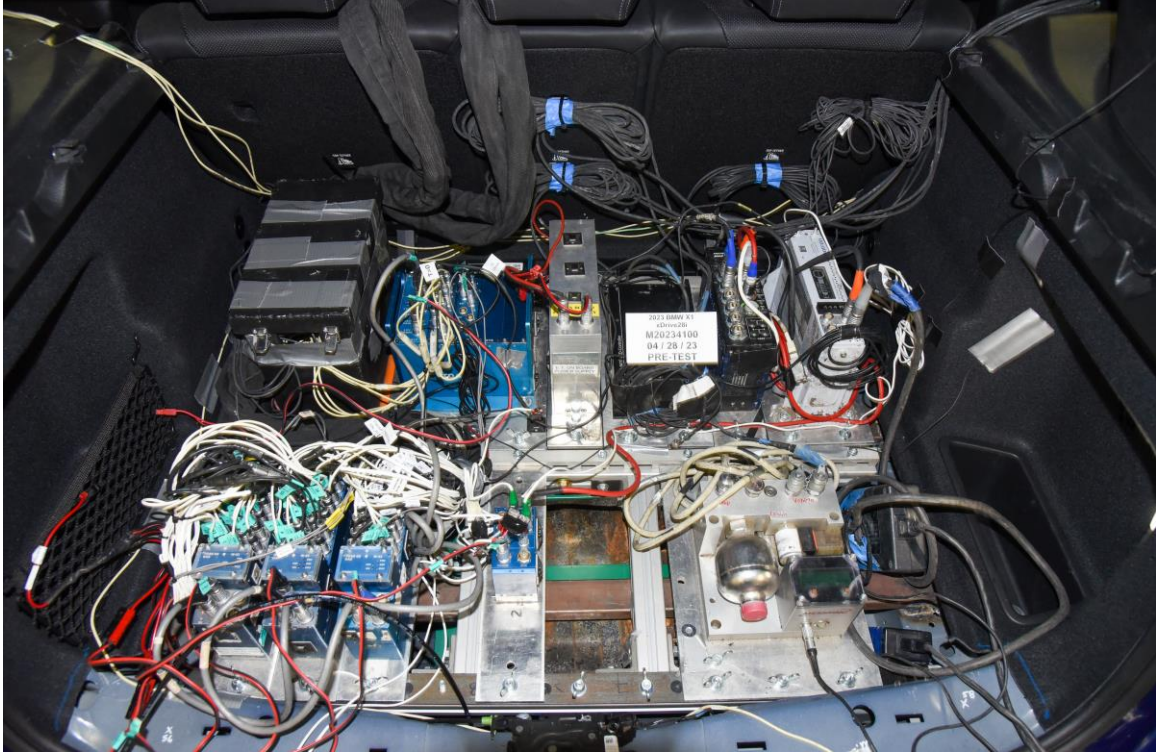
FIGURE 74. Photograph of Ballast Installed in Vehicle
