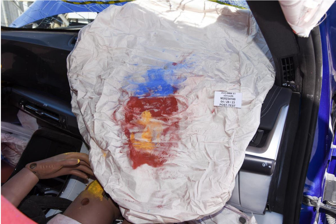
FIGURE 72. Post-Test Passenger Dummy Contact with Airbag
