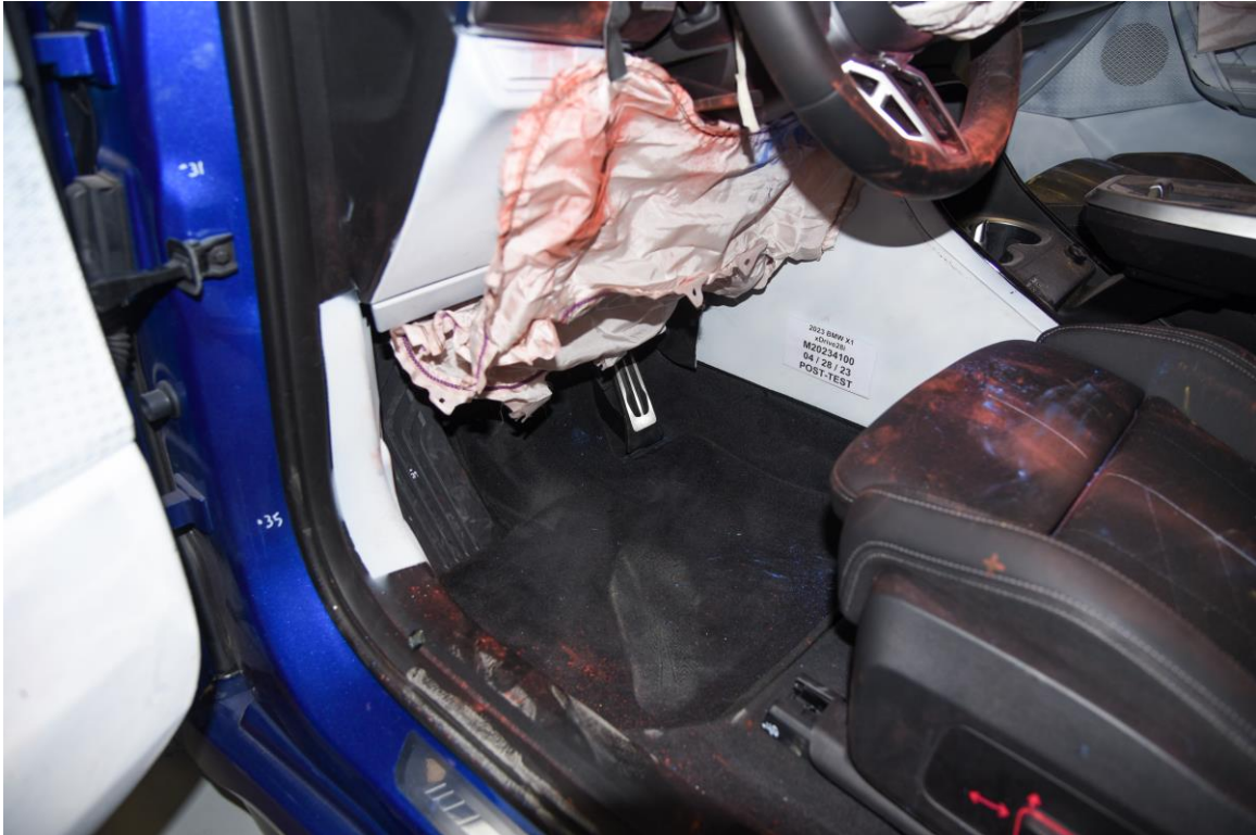
FIGURE 47. Post-Test Driver's Side Floorpan
