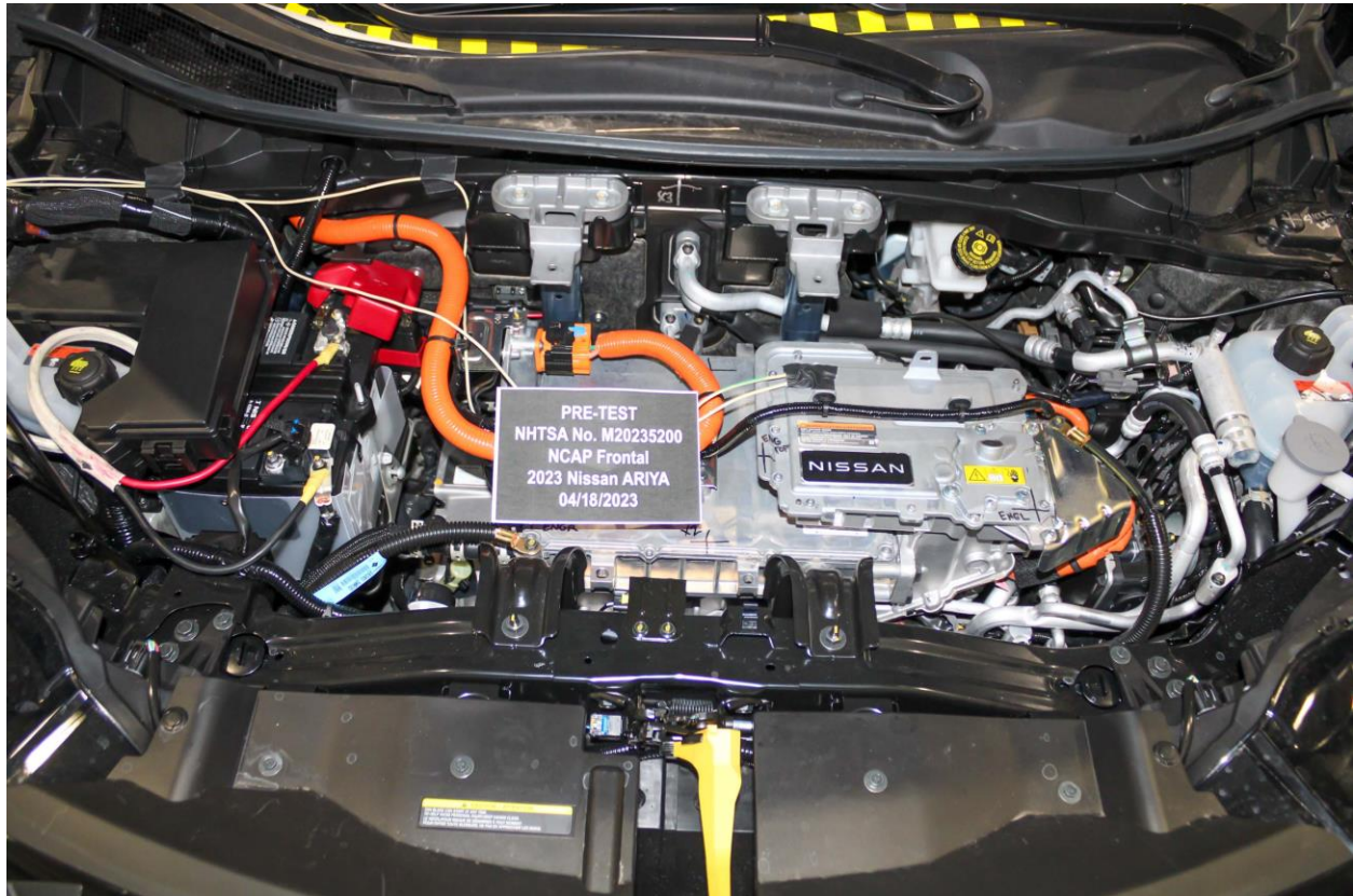
Figure 305-16: Pre-Impact View of Electric Propulsion Drive
