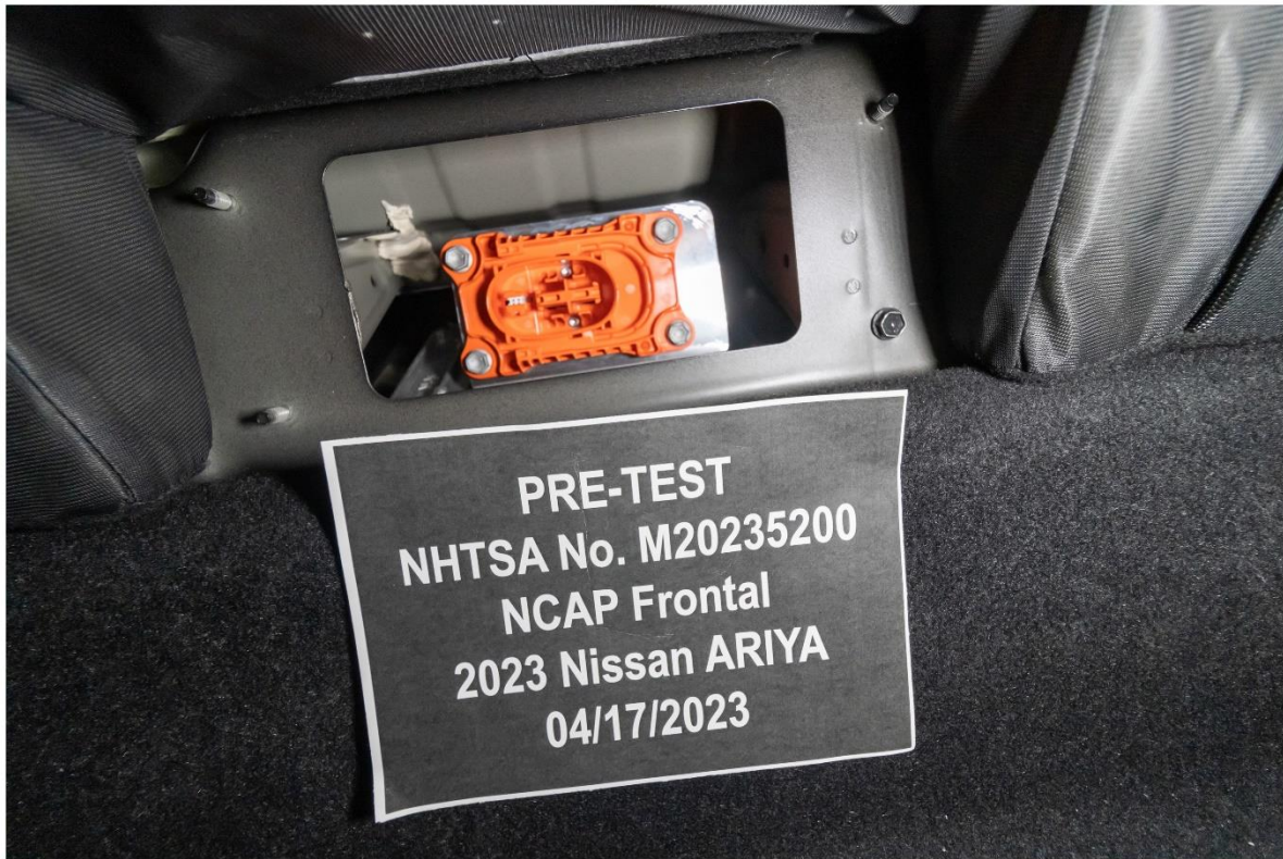
Figure 305-8: Manual High Voltage Service Disconnect Removed Location
