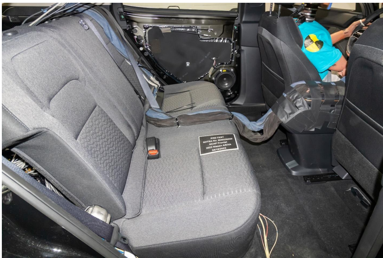
Figure A-28: Pre-Test Dummy Cable Routing
