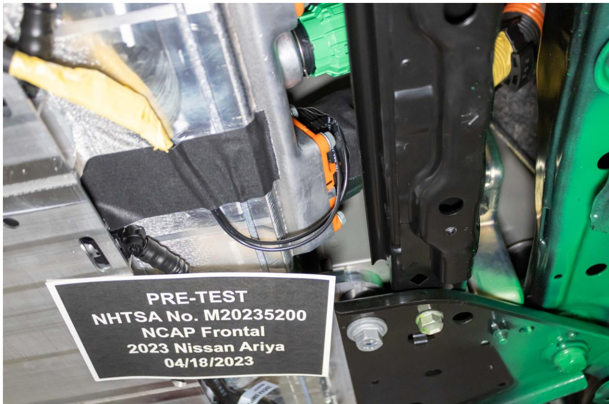
Figure 305-22: Pre-Impact View of High Voltage Leads Attached
