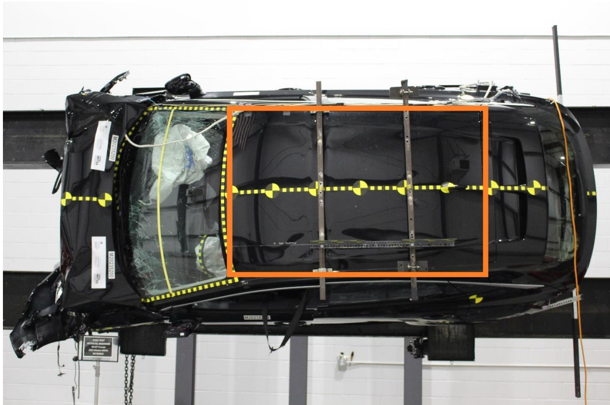
Figure 305-30: FMVSS No. 305 Static Rollover 270 Degrees
