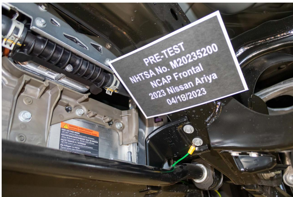
Figure 305-21: Pre-Impact View of Ground Lead Attached
