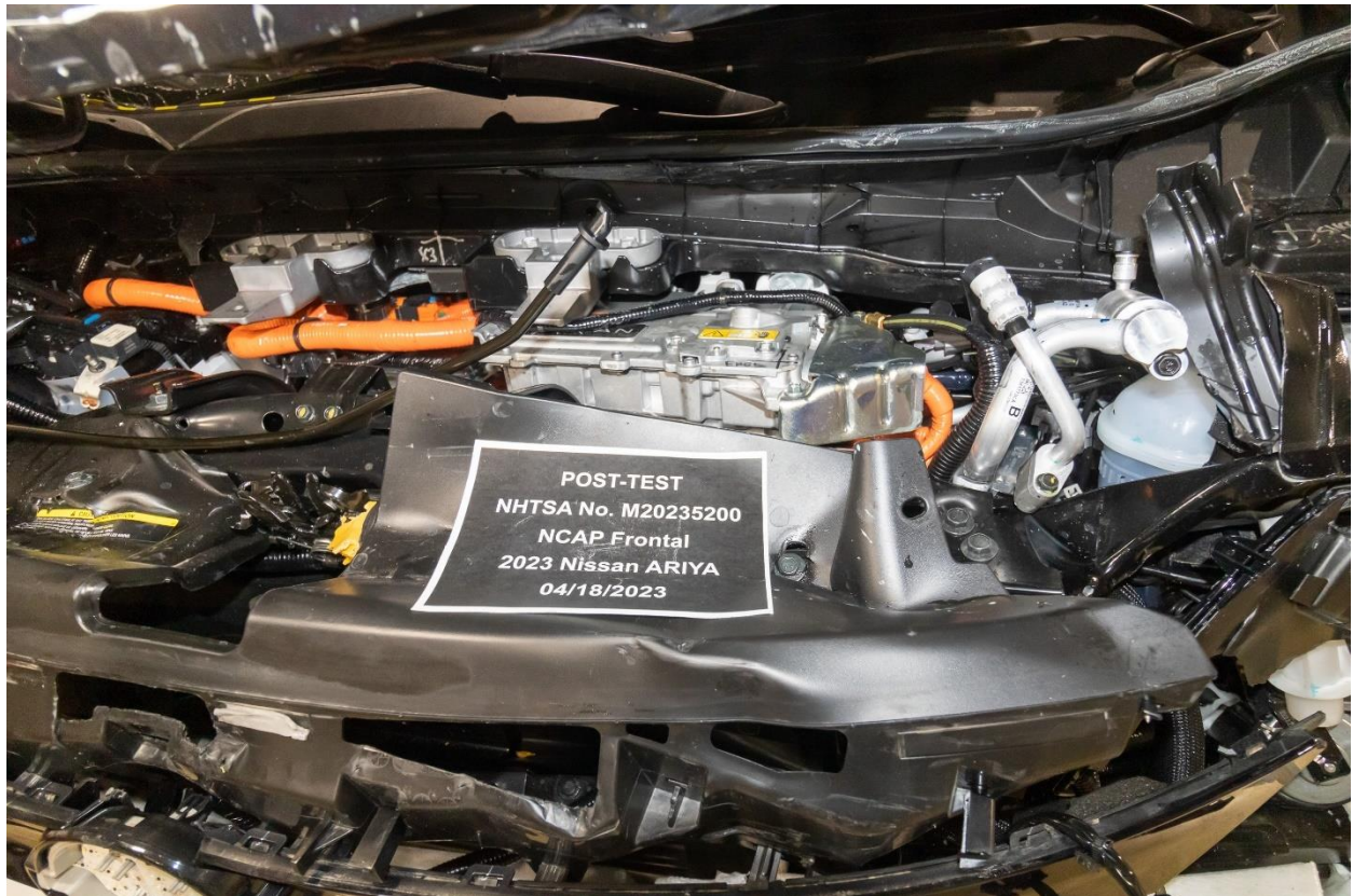
Figure 305-17: Post-Impact View of Electric Propulsion Drive
