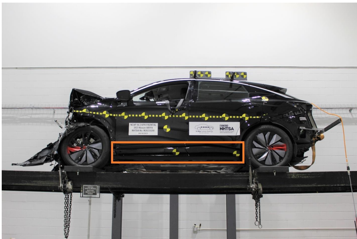
Figure 305-30: FMVSS No. 305 Static Rollover 270 Degrees
