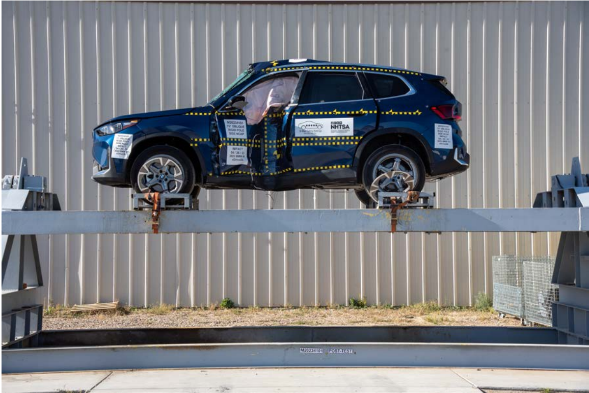
FIGURE 69. FMVSS No. 301 Static Rollover 360 Degrees
