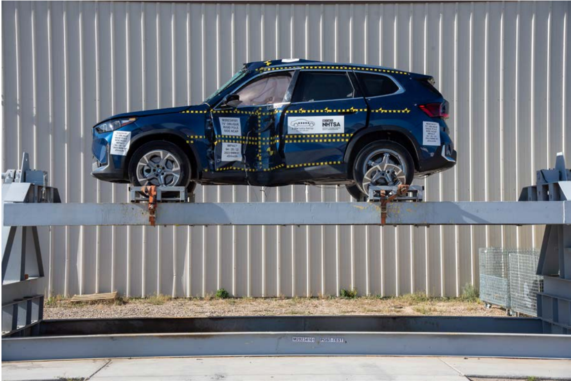
FIGURE 65. FMVSS No. 301 Static Rollover 0 Degrees
