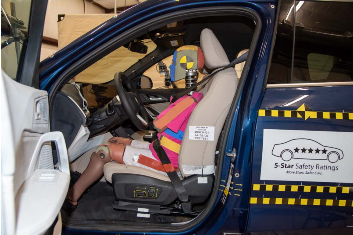
FIGURE 23. Pre-Test Left Side View of Dummy Showing Belt and Chalking
