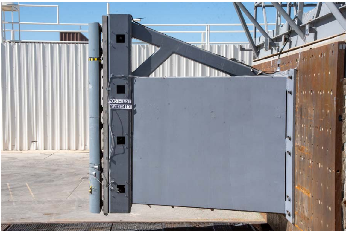
FIGURE 62. Post-Test Pole Barrier Side View
