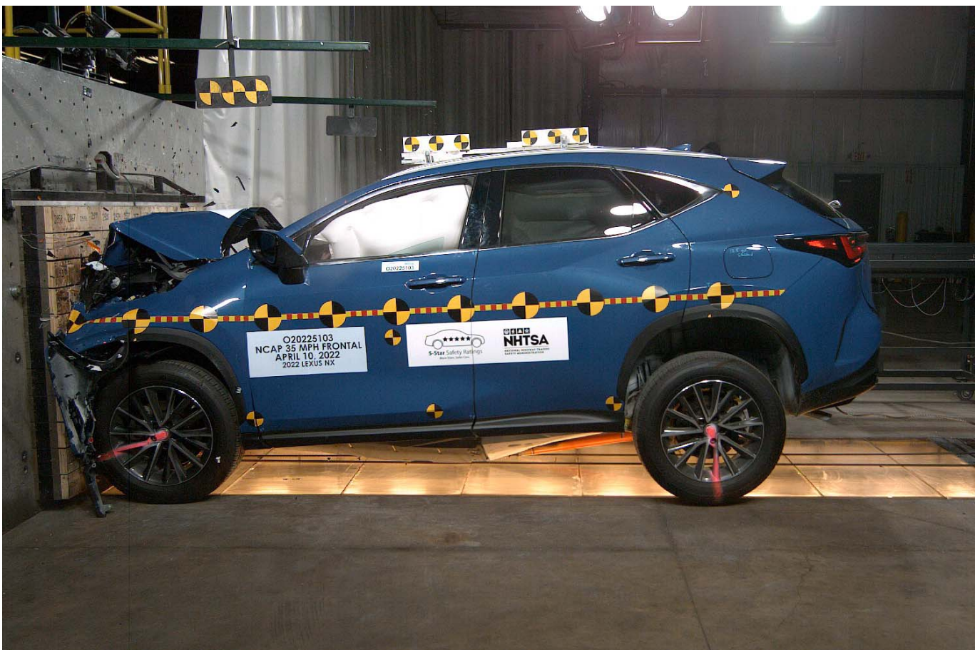
Photo No. 082 - 2022 Lexus NX 250 AWD 5-Door SUV Frontal Impact Event
