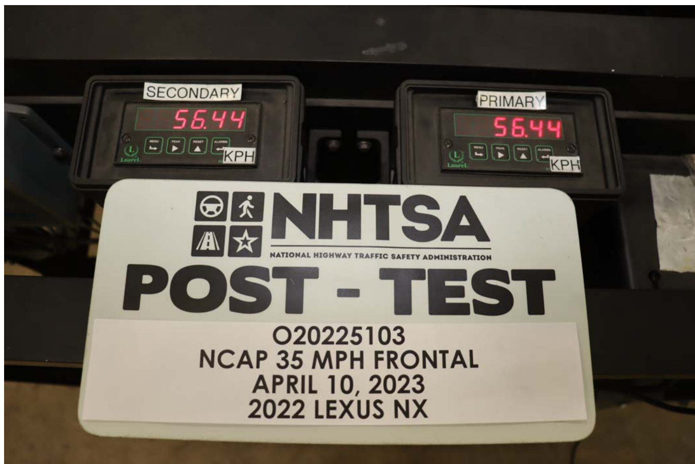
Photo No. 076 - Post-Test Speed Trap Read-Out
