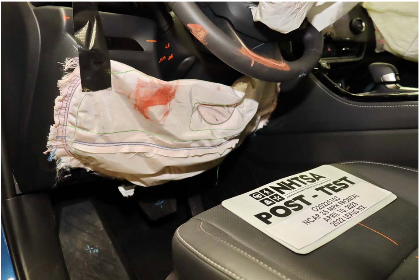
Photo No. 045 - Post-Test Driver's Side Knee Bolster
