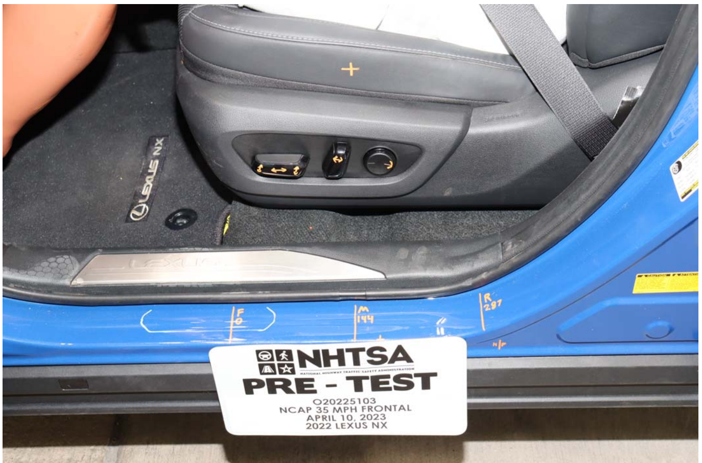
Photo No. 036 - Pre-Test Driver's Seat Fore-Aft Markings
