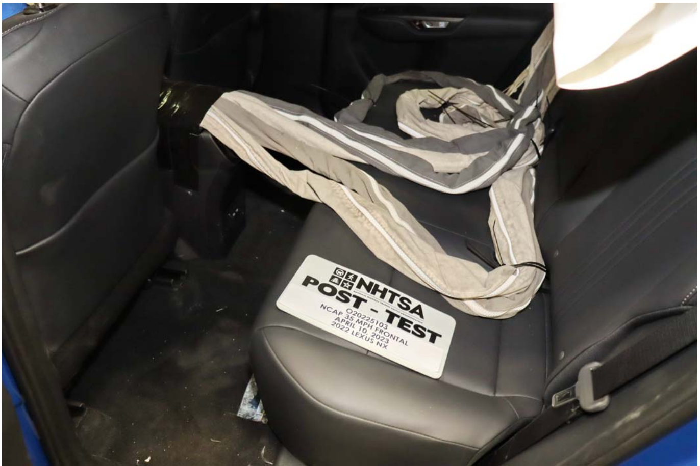
Photo No. 029 - Post-Test Dummy Cable Routing
