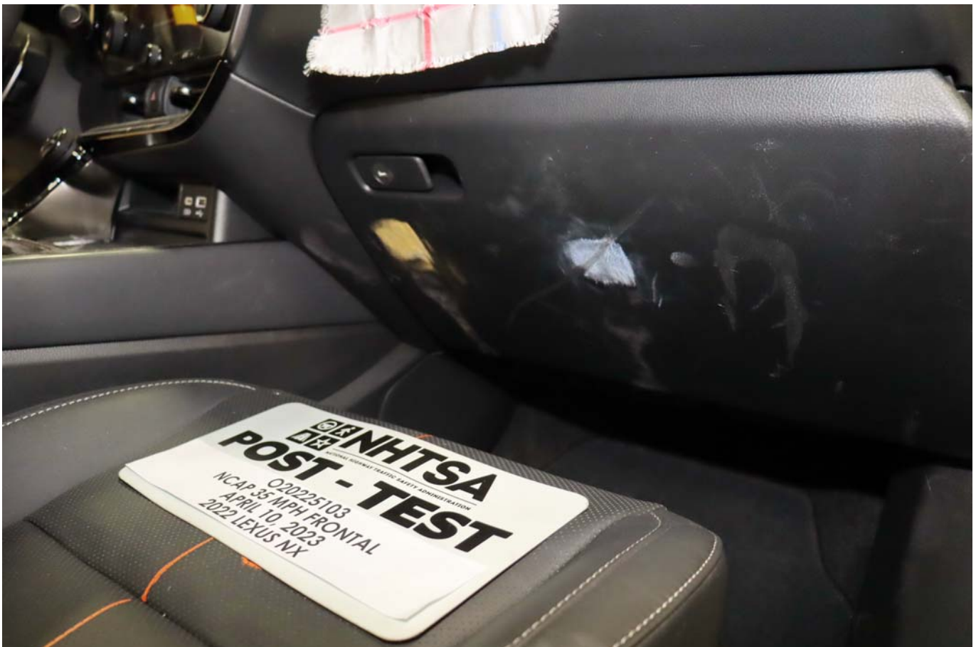
Photo No. 068 - Post-Test Passenger's Side Knee Bolster
