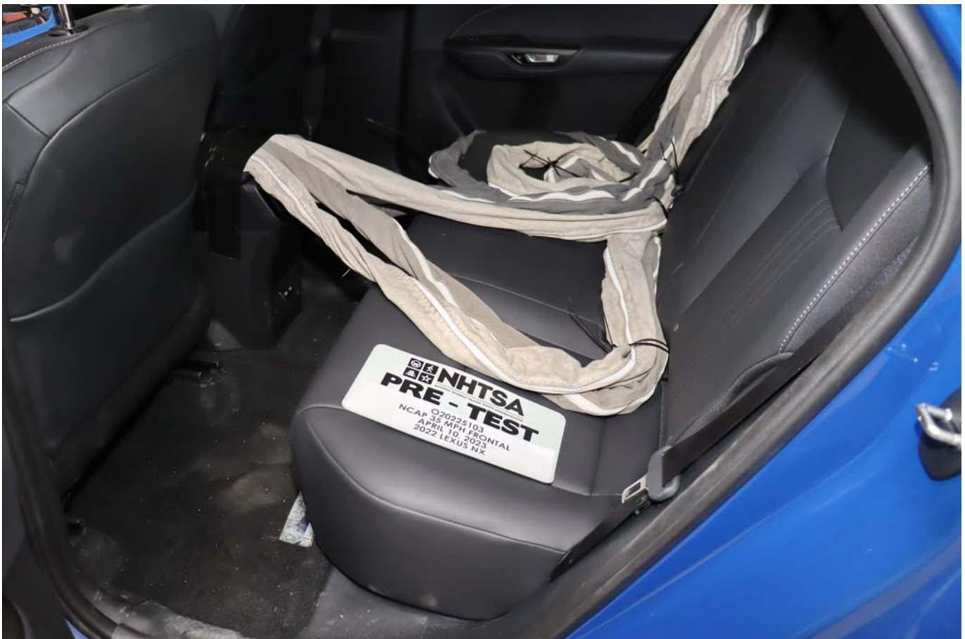
Photo No. 028 - Pre-Test Dummy Cable Routing
