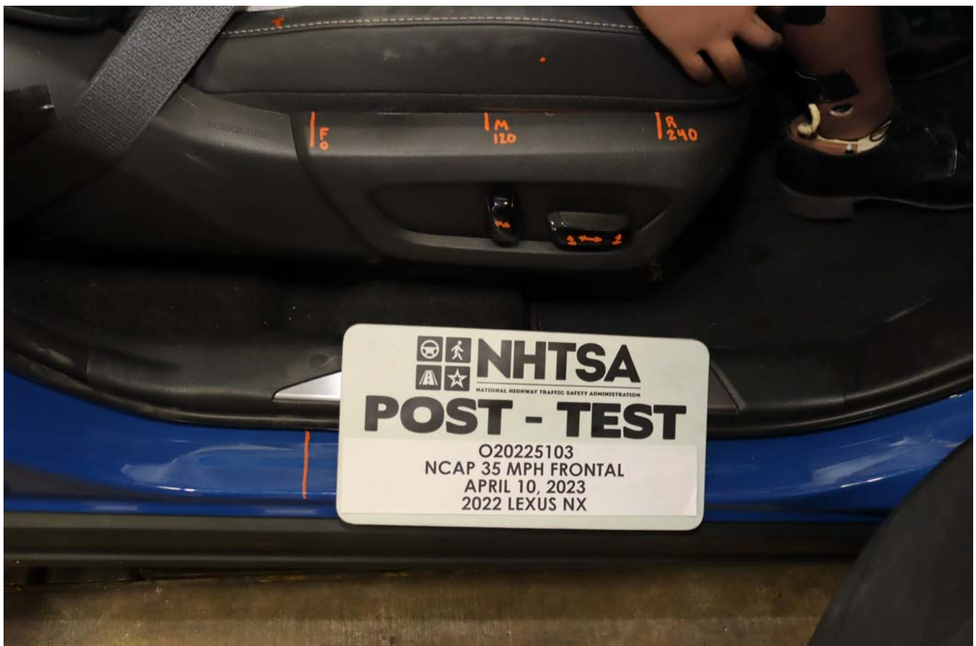
Photo No. 060 - Post-Test Passenger's Seat Fore-Aft Markings
