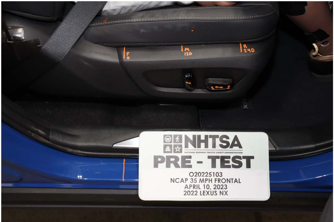
Photo No. 059 - Pre-Test Passenger's Seat Fore-Aft Markings
