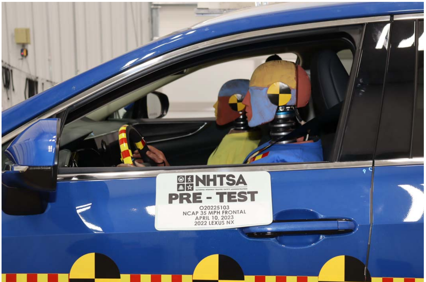
Photo No. 032 - Pre-Test Driver Dummy Window View
