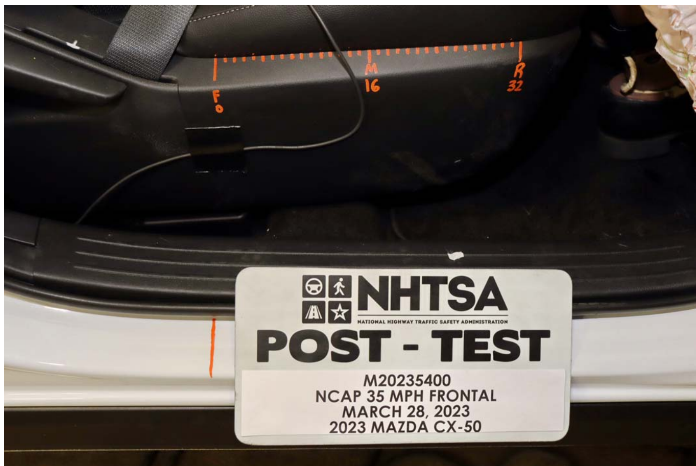
Photo No. 060 - Post-Test Passenger's Seat Fore-Aft Markings
