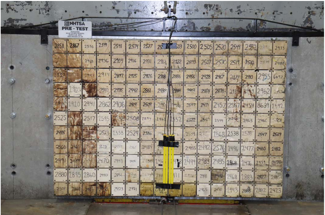
Photo No. 002 - Pre-Test Load Cell Wall
