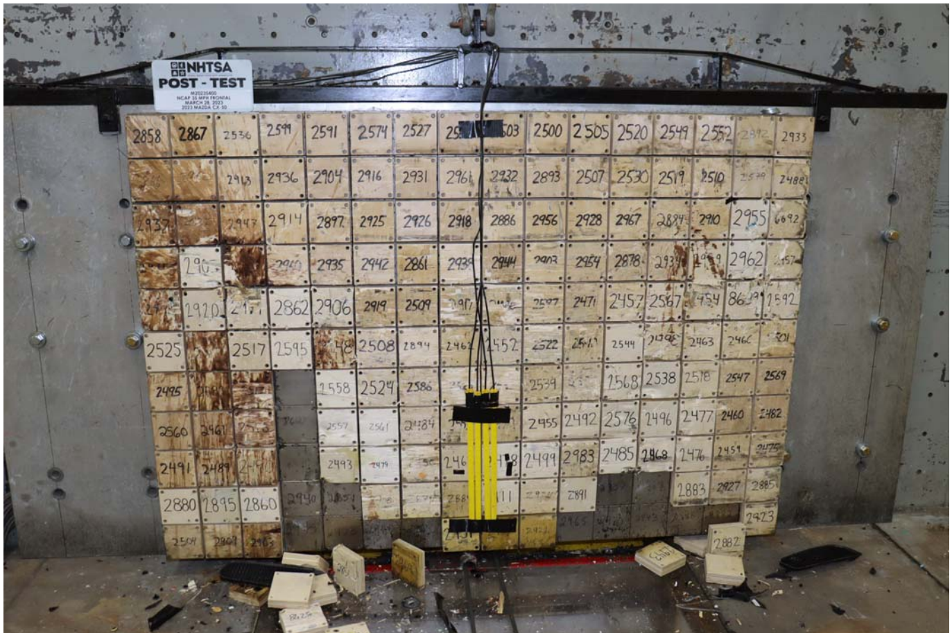
Photo No. 003 - Post-Test Load Cell Wall
