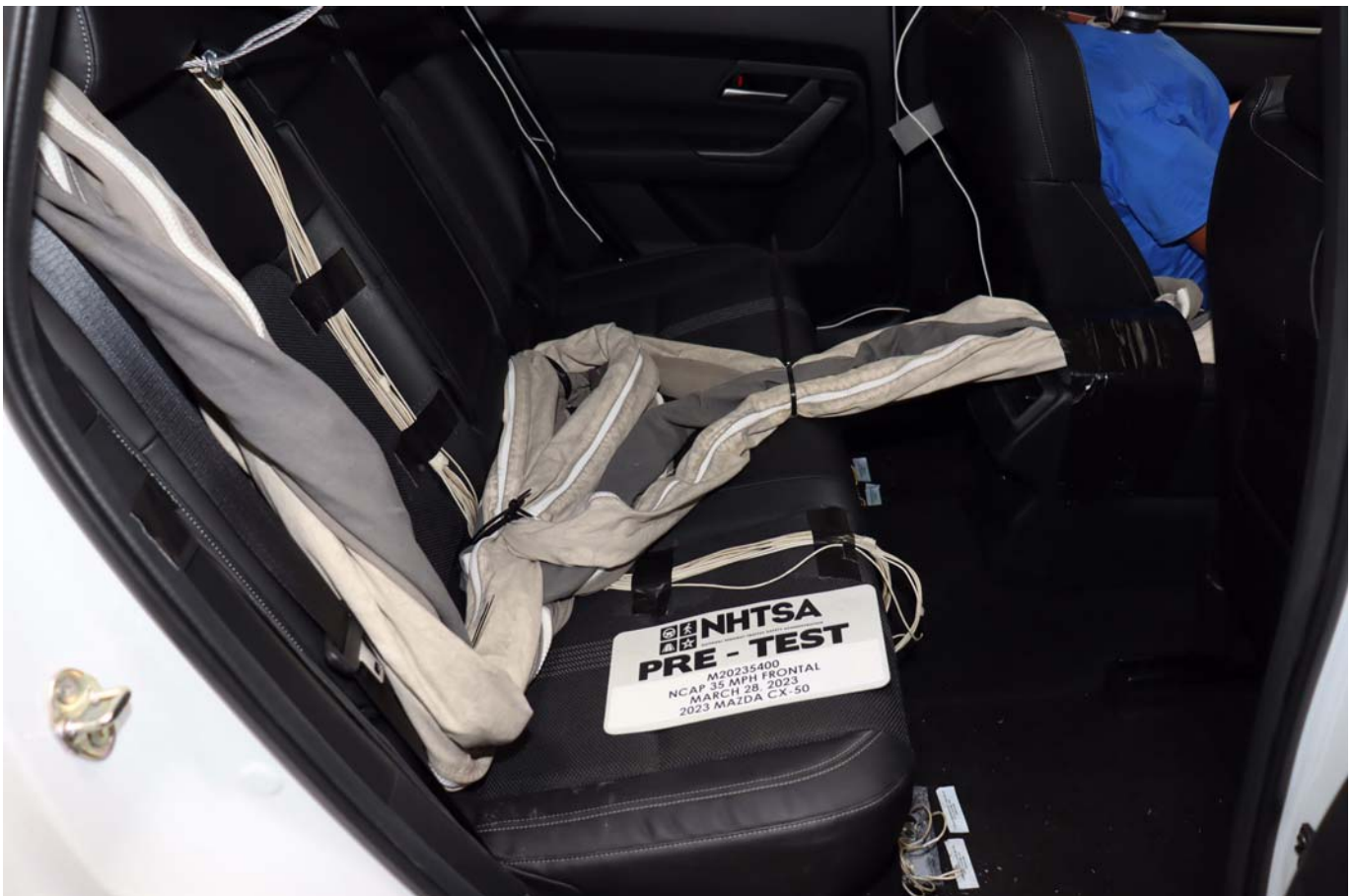
Photo No. 028 - Pre-Test Dummy Cable Routing
