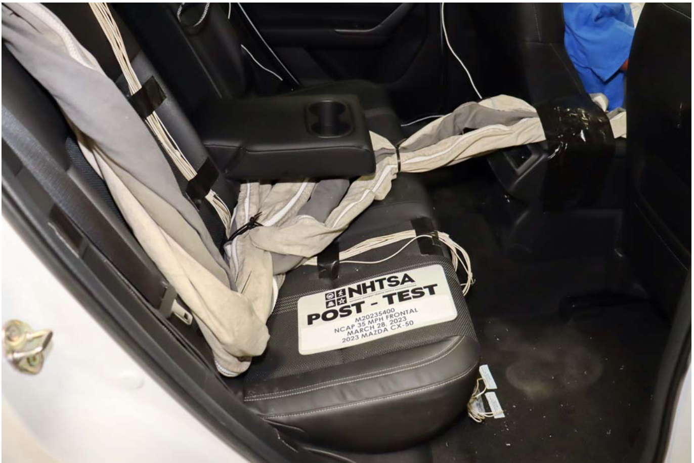
Photo No. 029 - Post-Test Dummy Cable Routing
