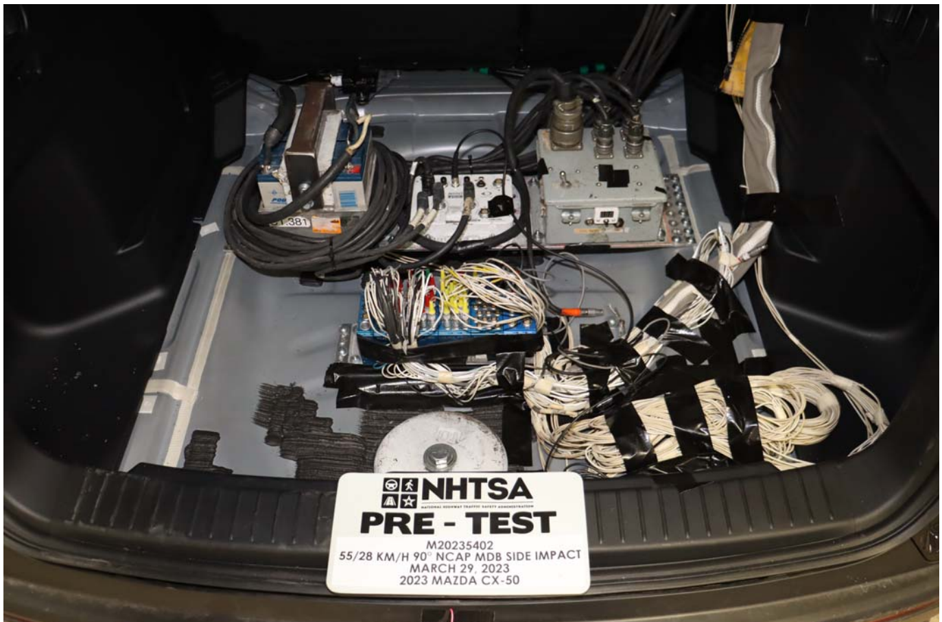
Photo No. 094 - Pre-Test Ballast View
