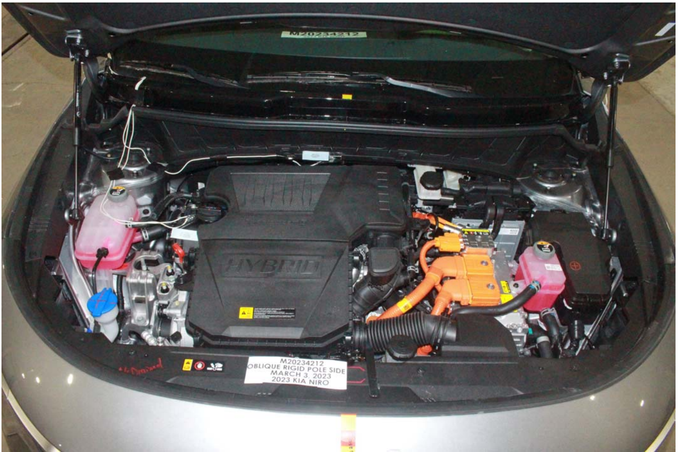
Photo No. 305-20 - Pre-Impact View of Other Visible Electric Propulsion Components
