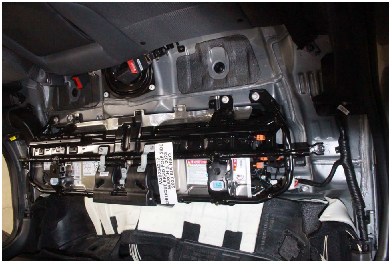
Photo No. 305-09 - Pre-Impact View of Propulsion Battery
