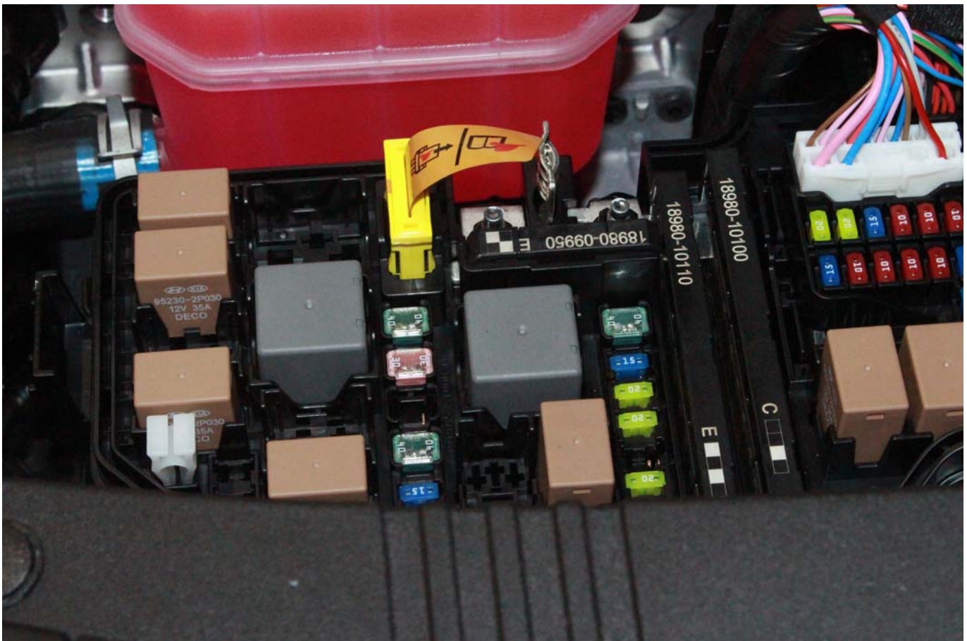
Photo No. 305-03 - First Responder Warning Label
