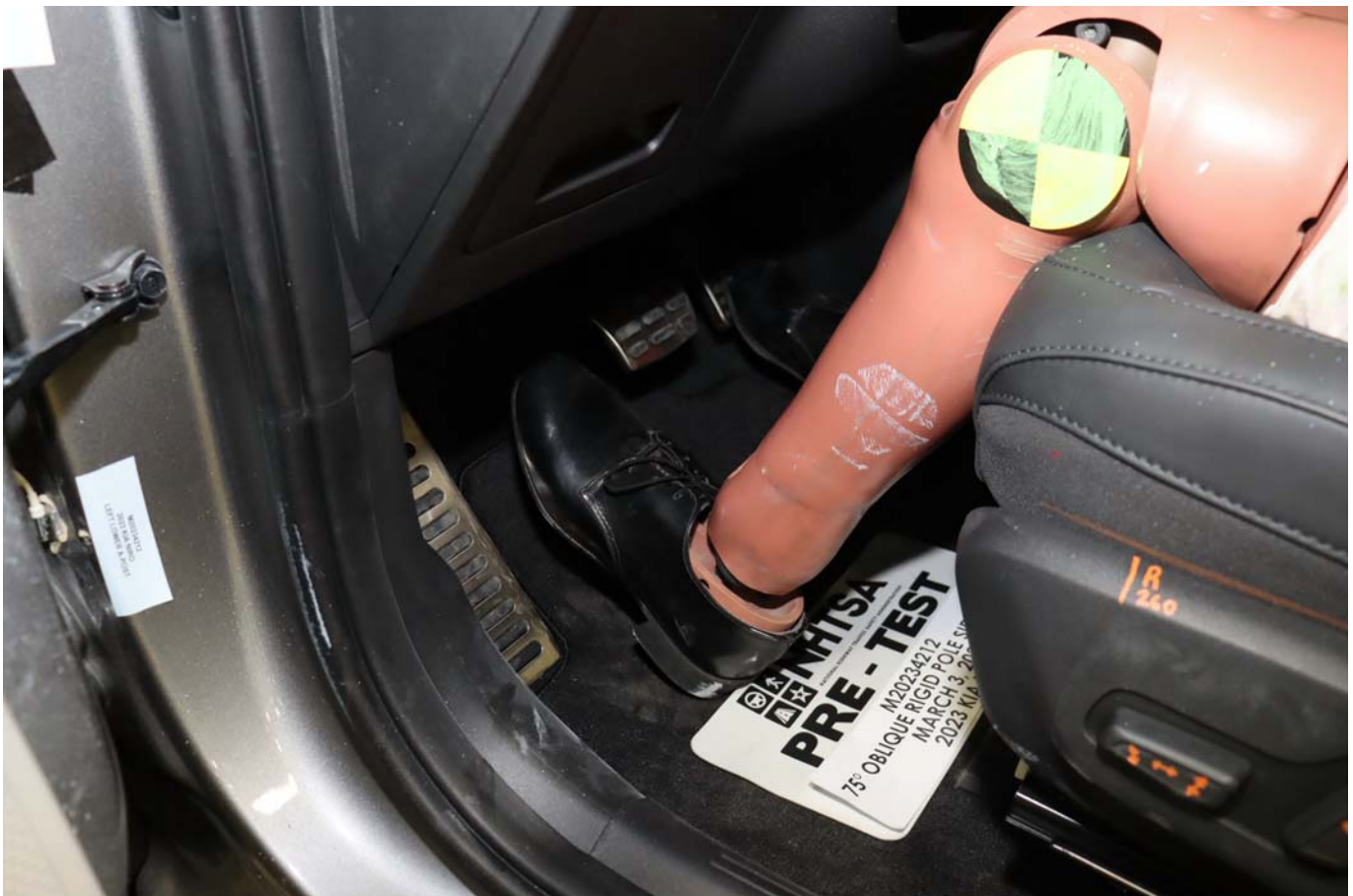
Photo No. 032 - Pre-Test Placement of Dummy's Feet
