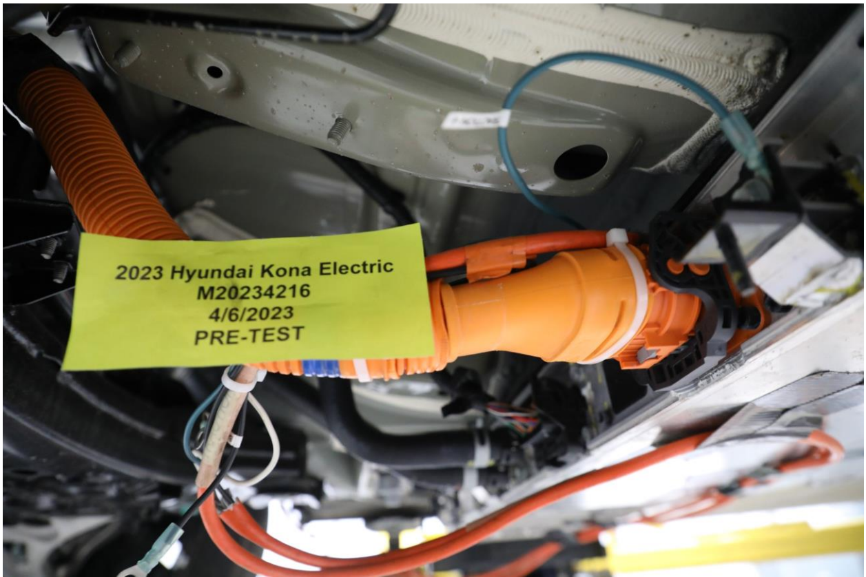
305-22 Pre-Impact View of High Voltage Leads Attached
