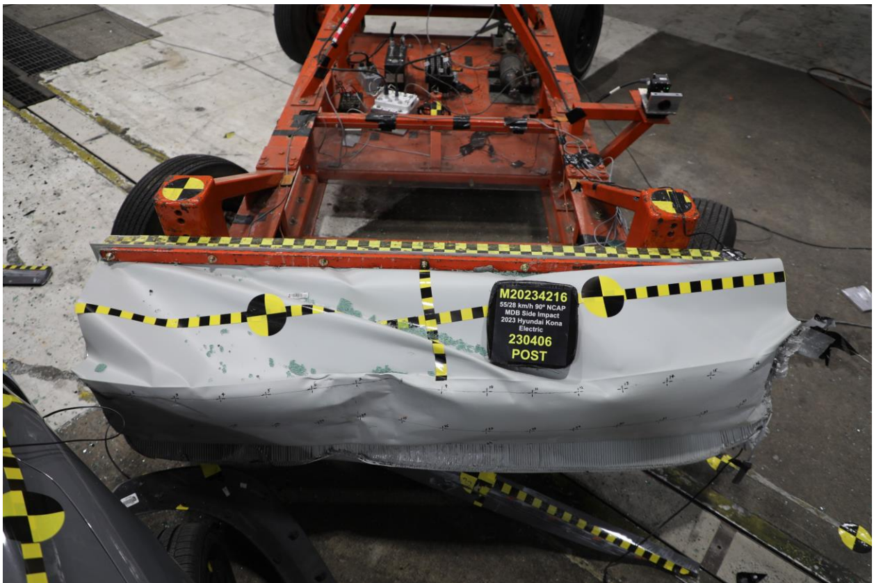
087 Post-Test Top View of MDB Impactor Face
