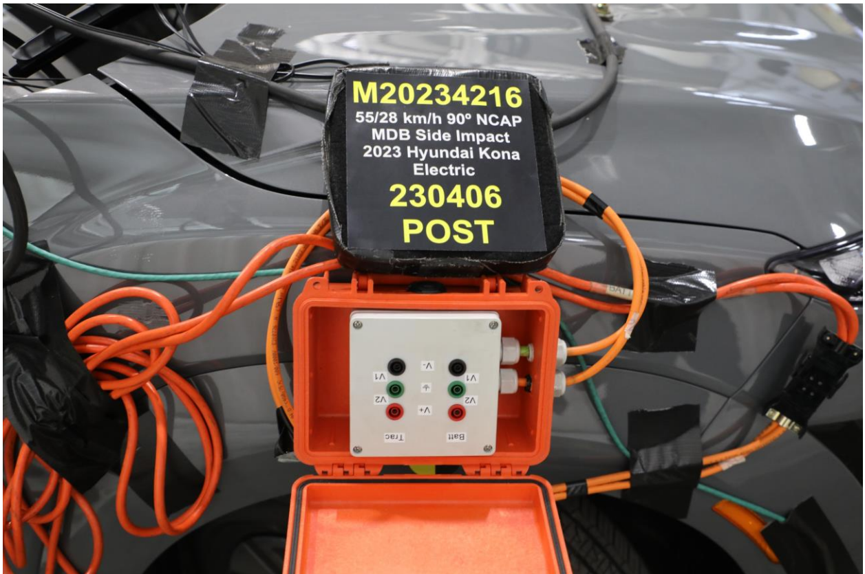
305-25 Post-Impact View of Installed Test Interface Port
