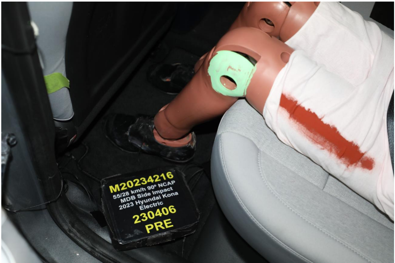
064 Pre-Test Placement of Rear Passenger Dummy's Feet
