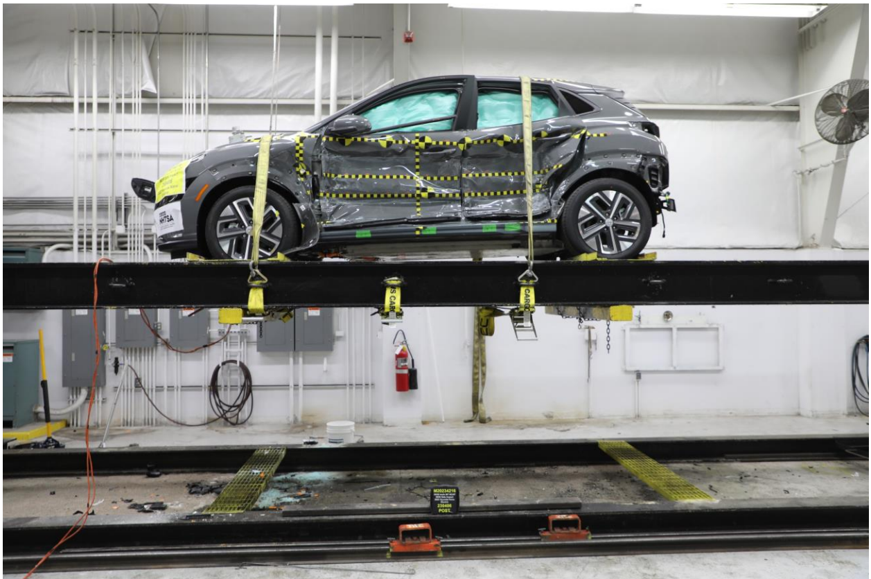
096 FMVSS No. 301 Static Rollover 0 Degrees
