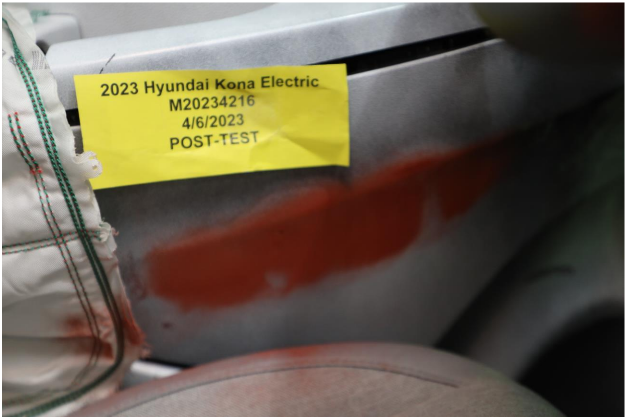
052 Post-Test Driver Dummy Close-Up Pelvis Contact View
