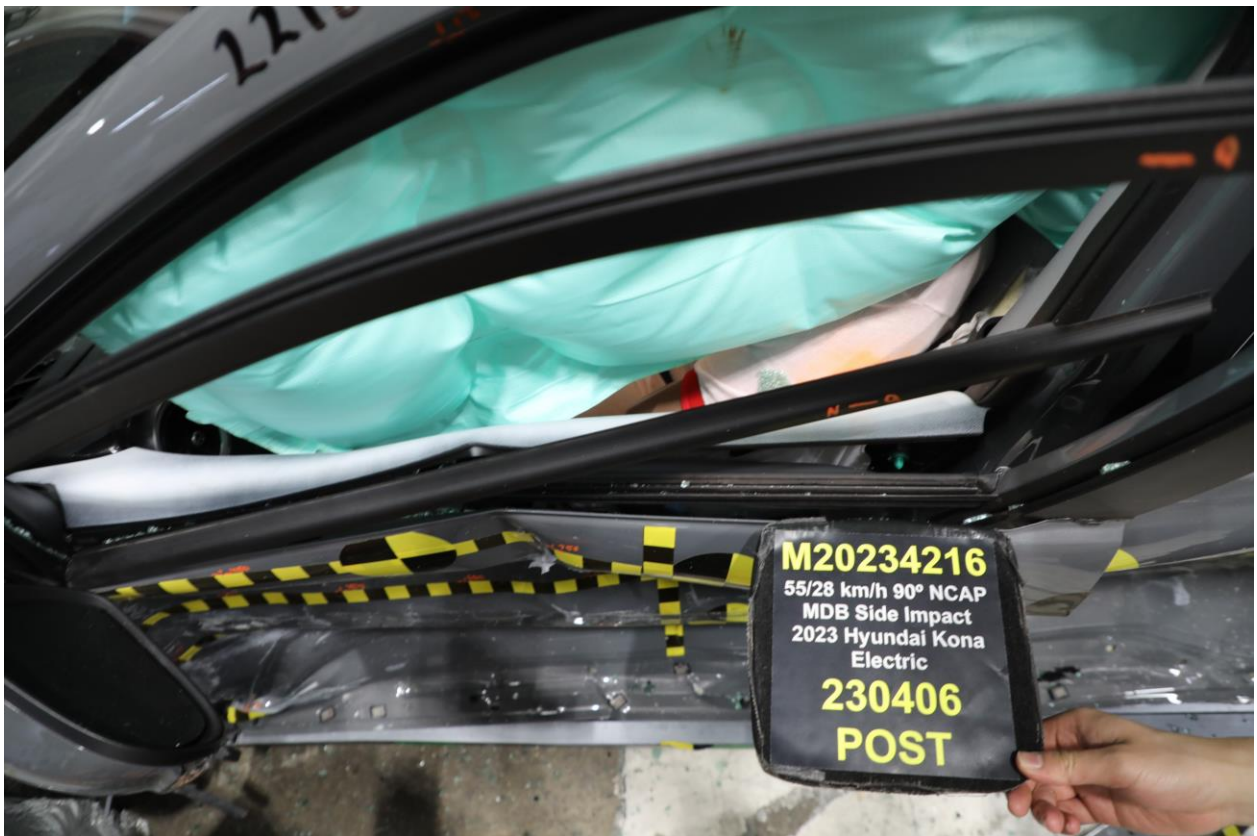
043 Post-Test Driver Dummy and Door Clearance View
