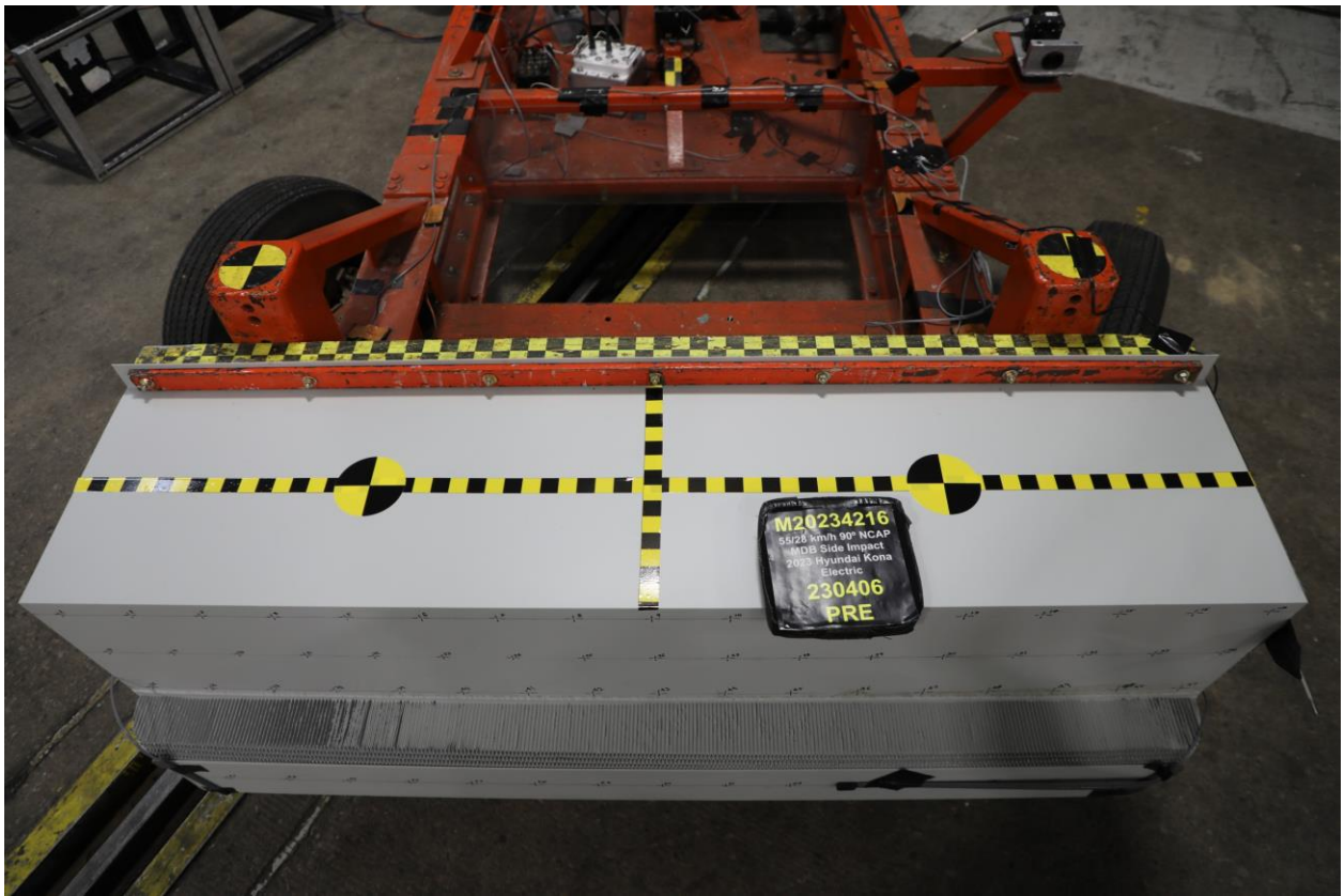
086 Pre-Test Top View of MDB Impactor Face
