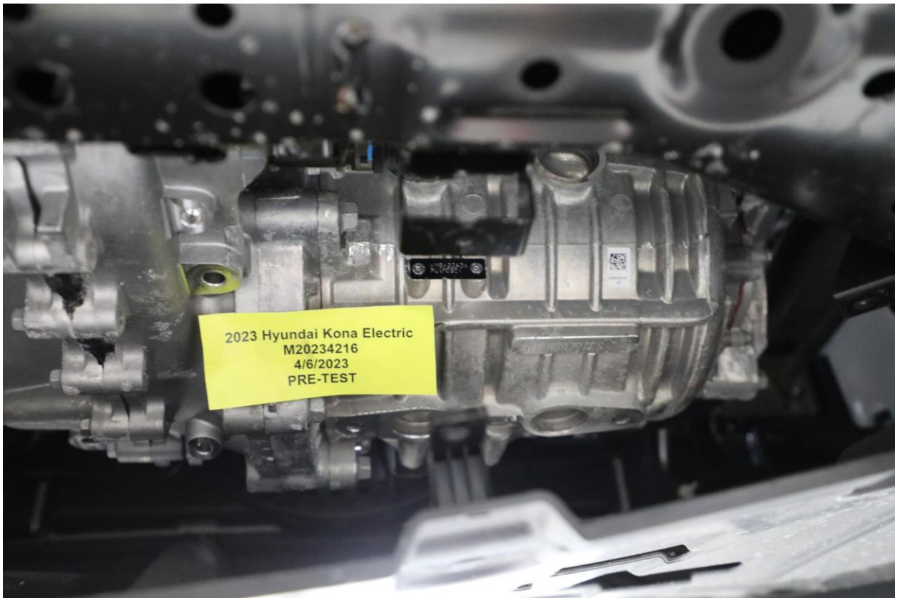
305-16 Pre-Impact View of Electric Propulsion Drive
