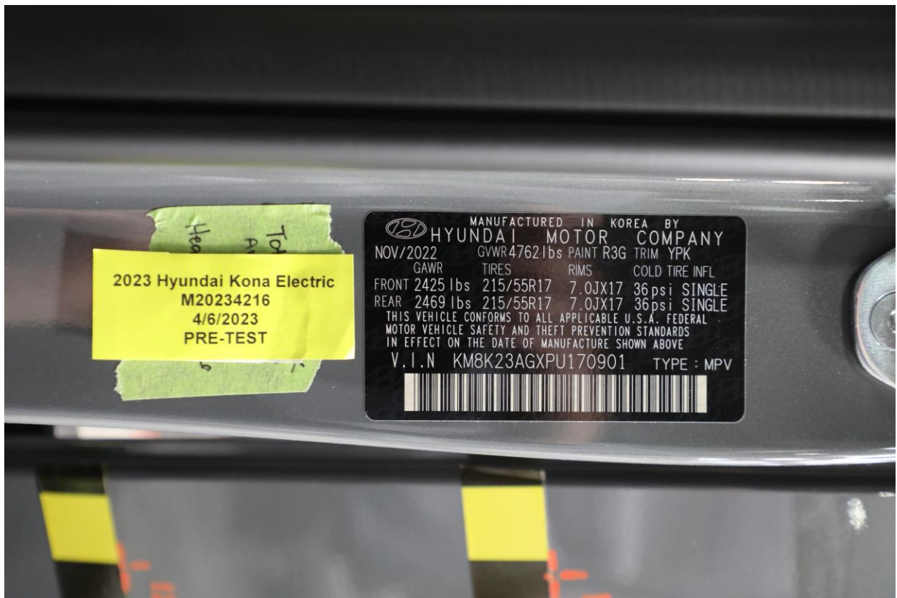
092 Close-Up View of Vehicle's Certification Label
