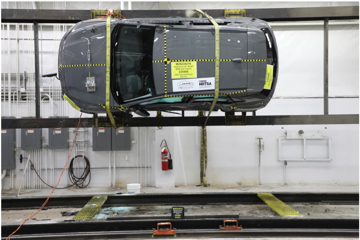
305-28 FMVSS No. 305 Static Rollover at 90°
