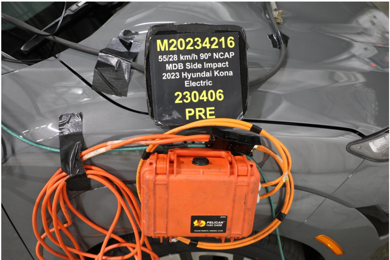
305-24 Pre-Impact View of Installed Test Interface Port
