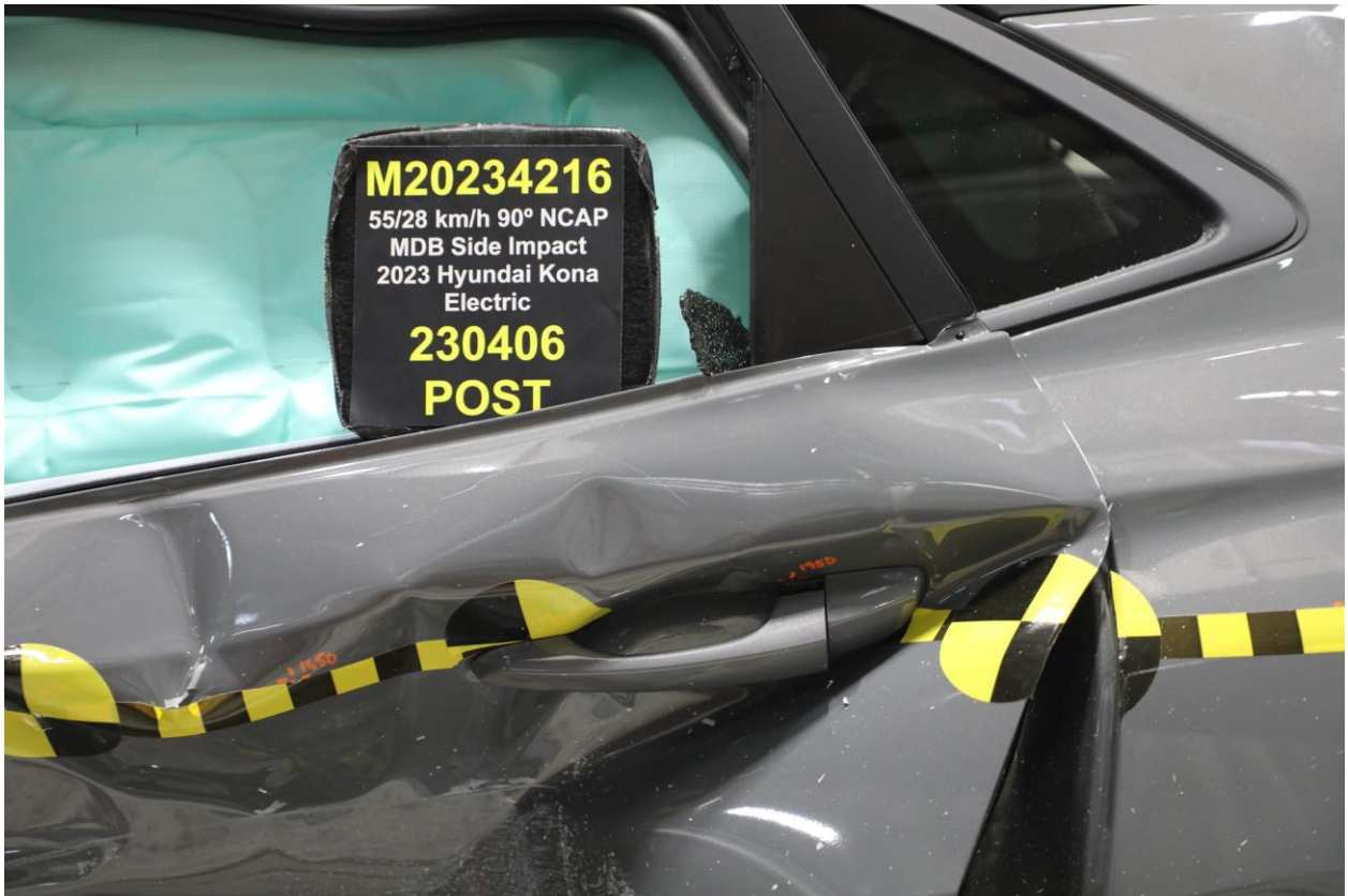
024 Post-Test Left Rear Door Latch Close-Up
