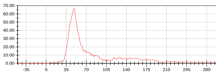
Passenger Lower Spine T12 Resultant Acceleration (g) vs. Time [ms]
