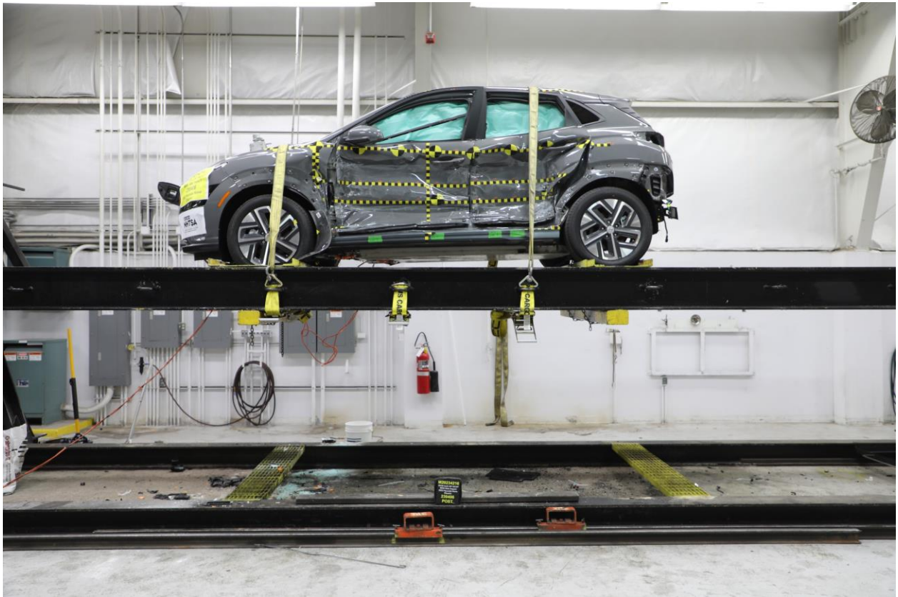
100 FMVSS No. 301 Static Rollover 360 Degrees
