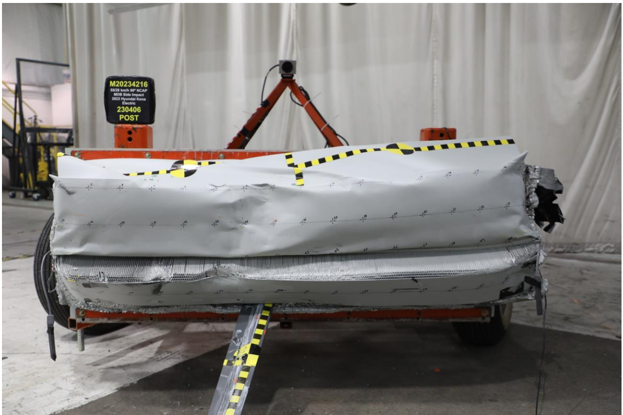
085 Post-Test Front View of MDB Impactor Face
