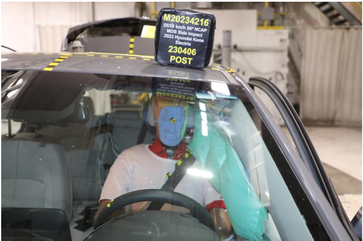
026 Post-Test Front Close-Up View of Driver Dummy
