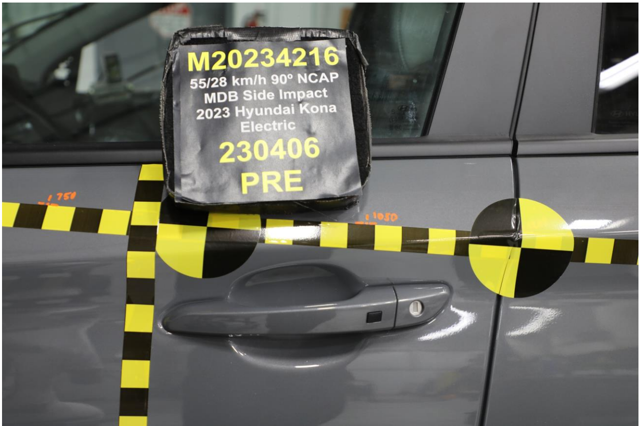
021 Pre-Test Left Front Door Latch Close-Up
