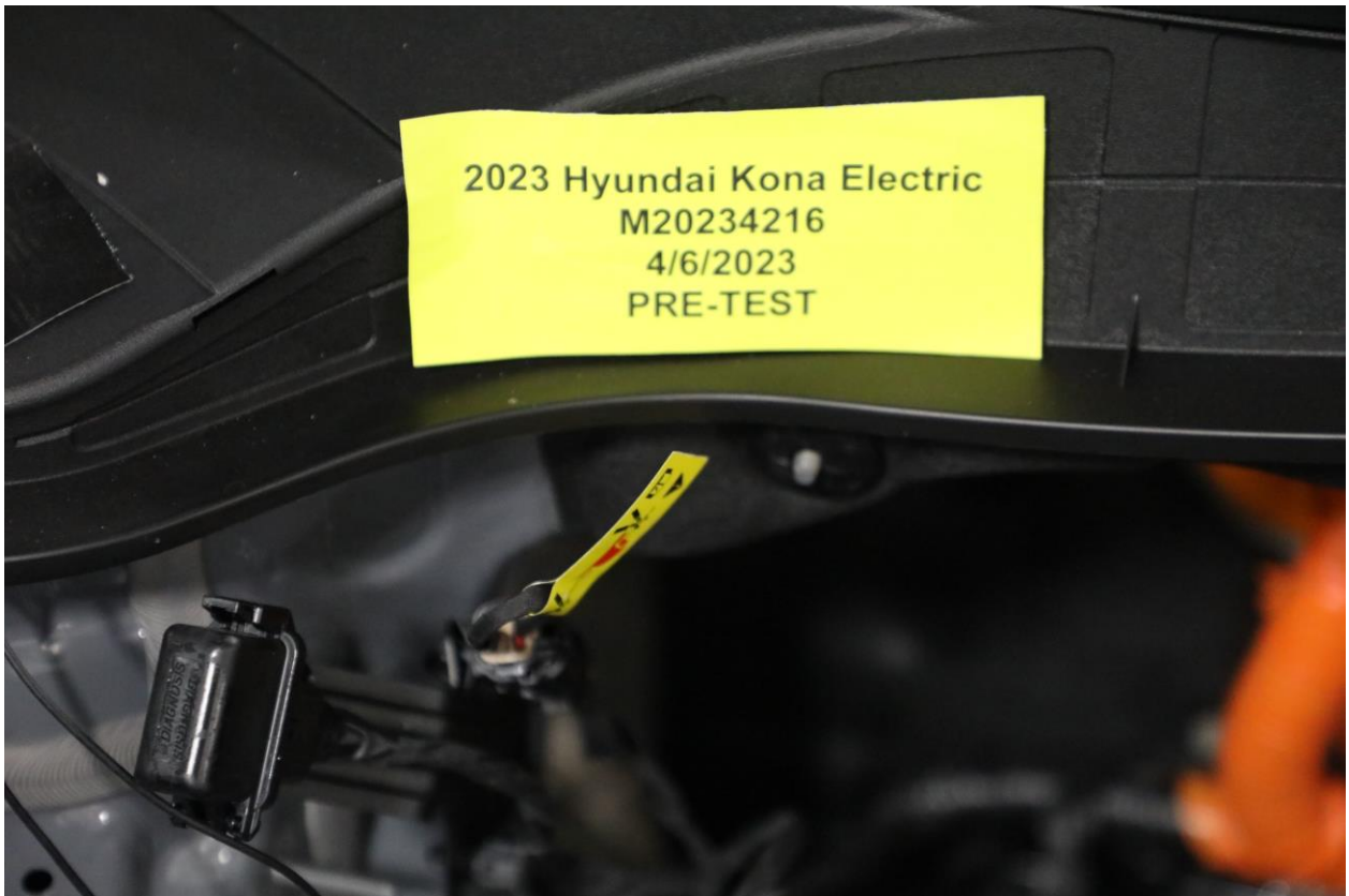
305-06 Manual High Voltage Service Disconnect in Place
