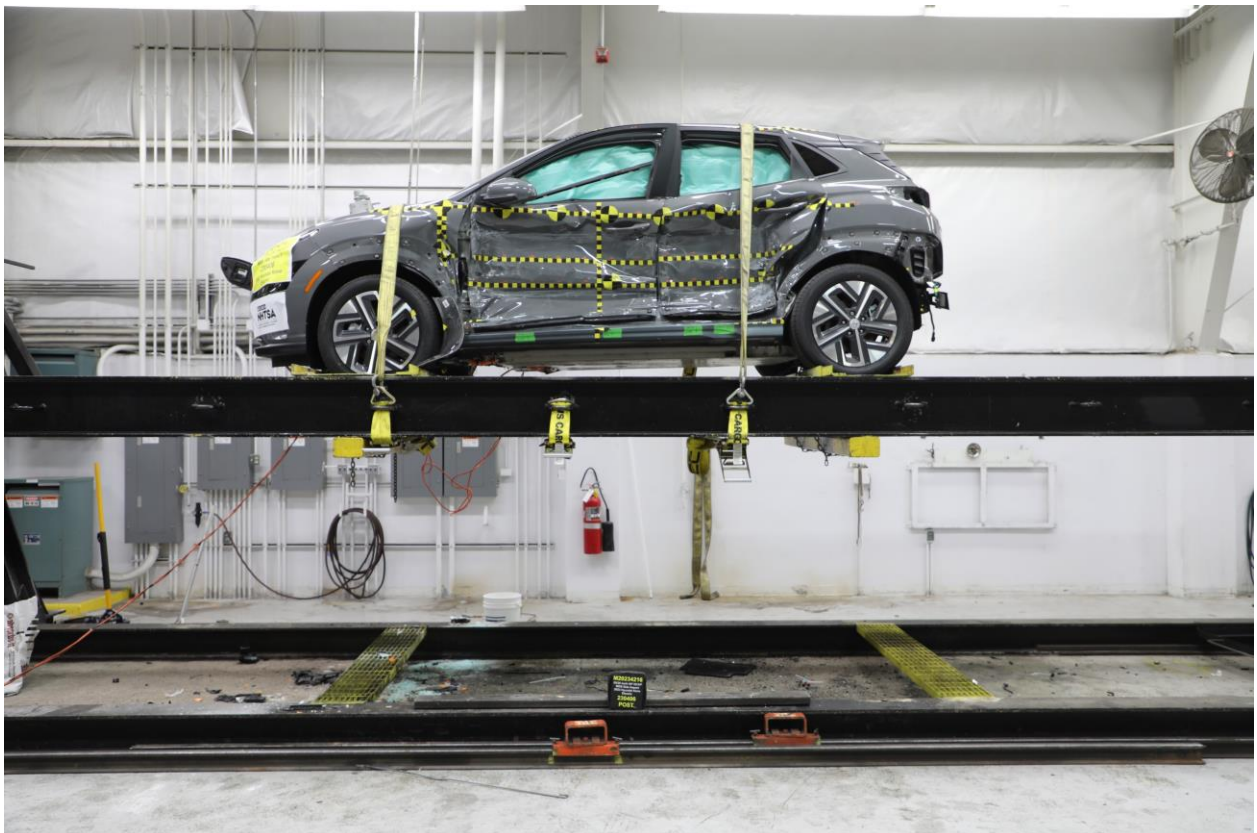
305-31 FMVSS No. 305 Static Rollover at 360°
