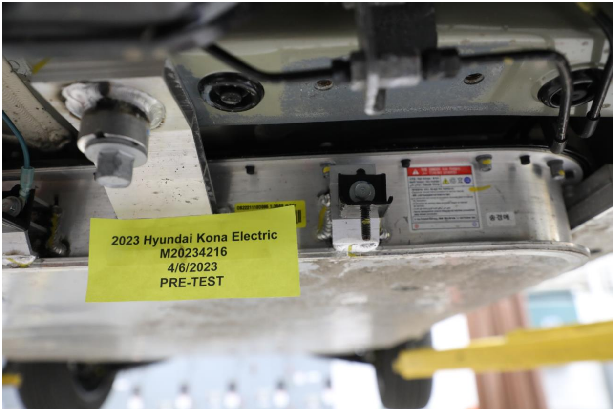
305-14 Pre-Impact View of Propulsion Battery Module(s)
