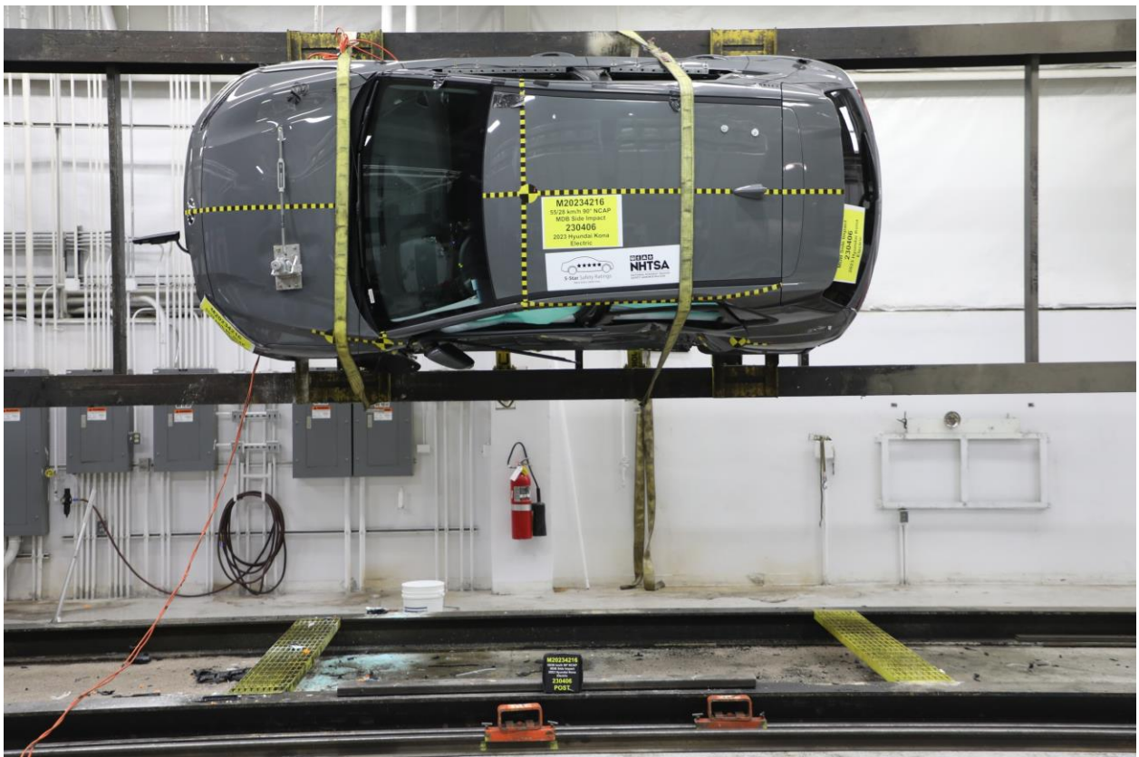
097 FMVSS No. 301 Static Rollover 90 Degrees
