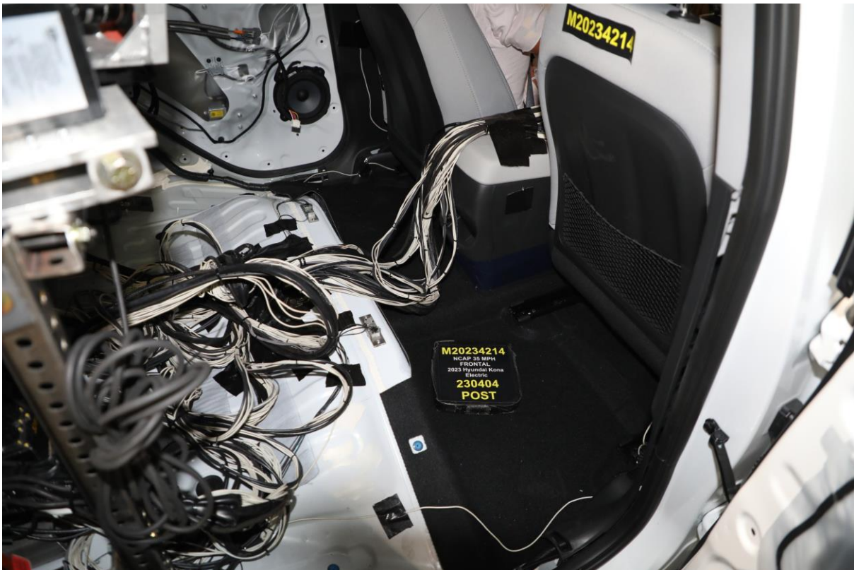
029 Post-Test Dummy Cable Routing
