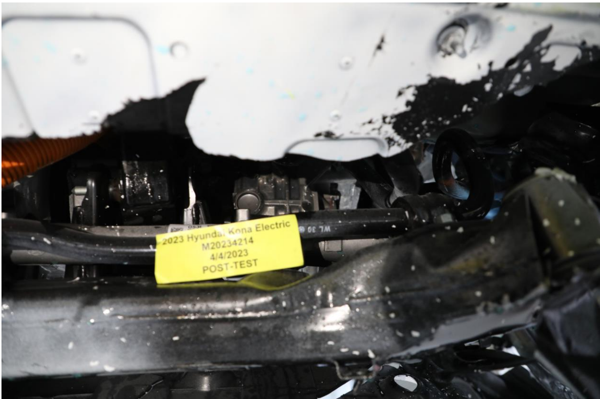
305-17 Post-Impact View of Electric Propulsion Drive
