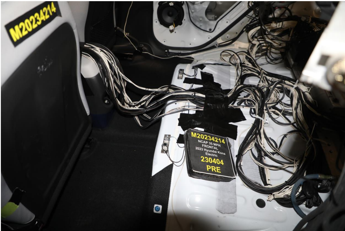
028 Pre-Test Dummy Cable Routing
