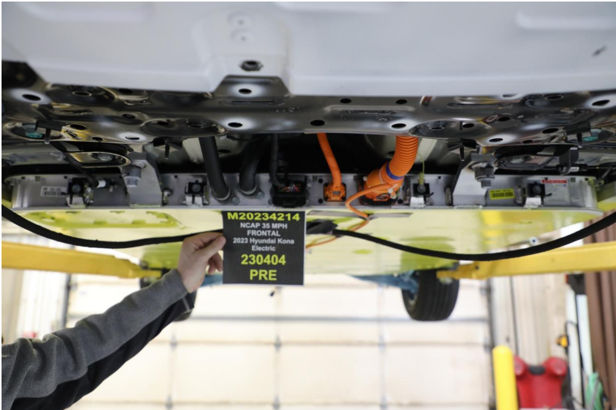
305-09 Pre-Impact View of Propulsion Battery
