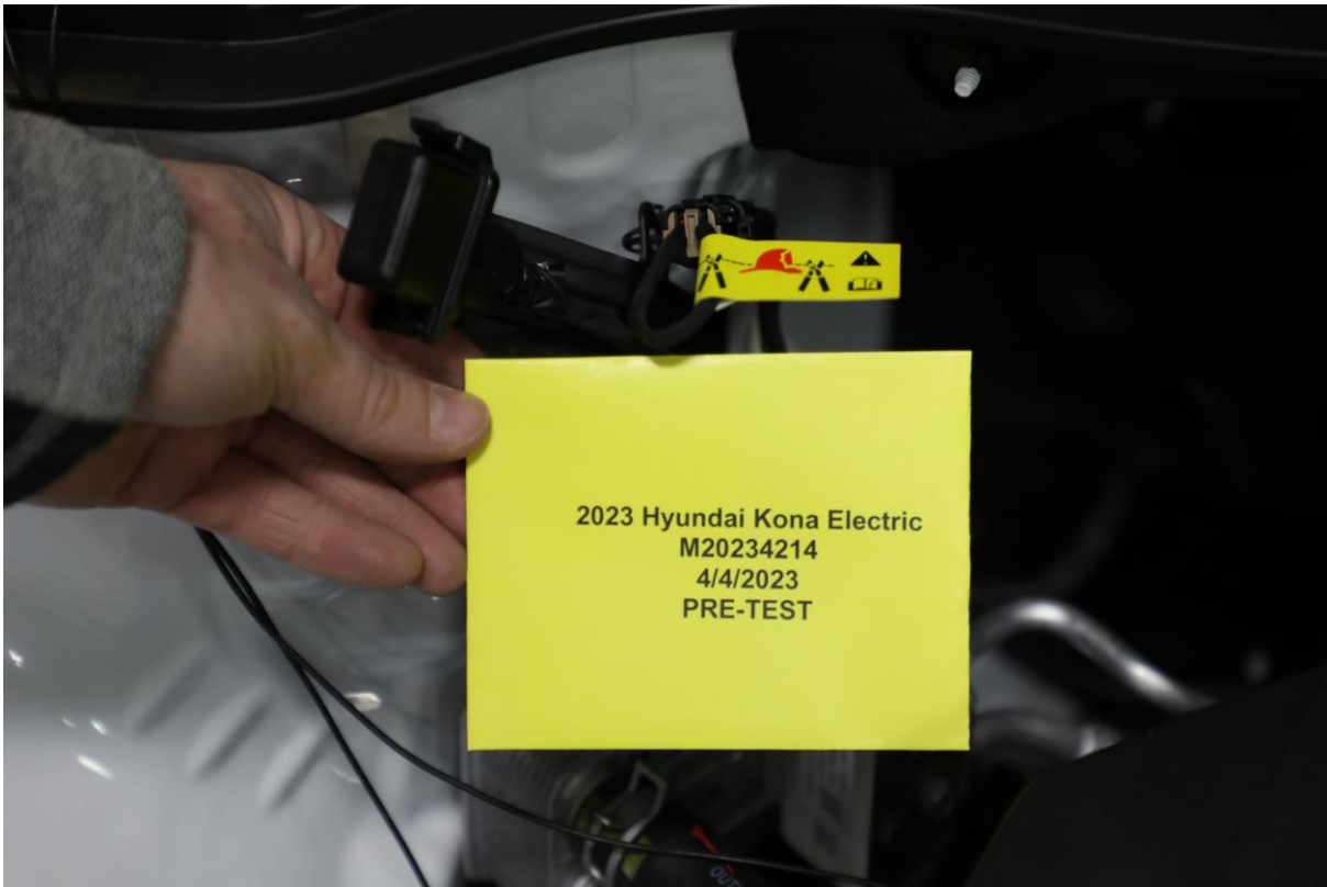
305-06 Manual High Voltage Service Disconnect in Place
