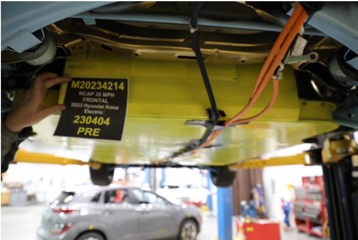
305-12 Pre-Impact View of Battery Box(s) or Container(s) Which Holds Individual Battery Modules
