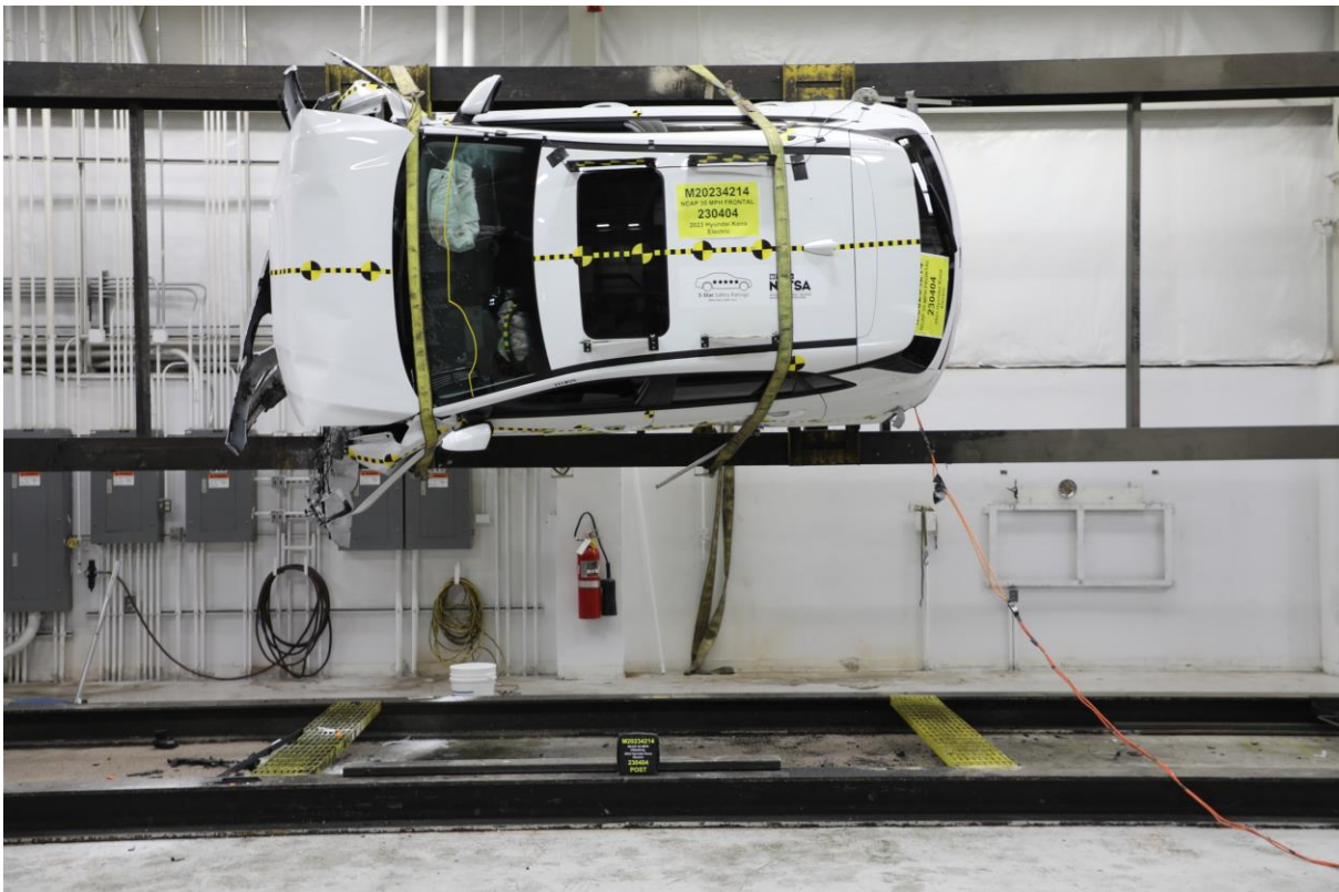
078 Vehicle at 90° on Static Rollover Device
