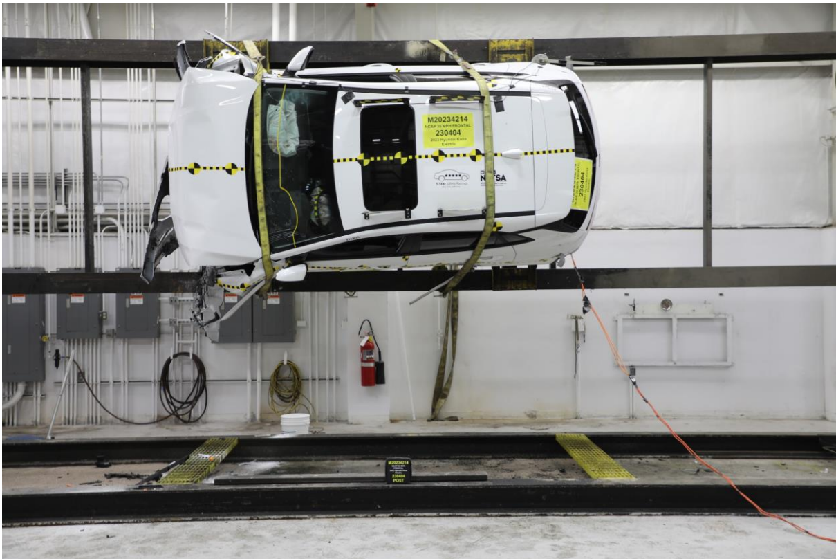
305-28 FMVSS No. 305 Static Rollover at 90°
