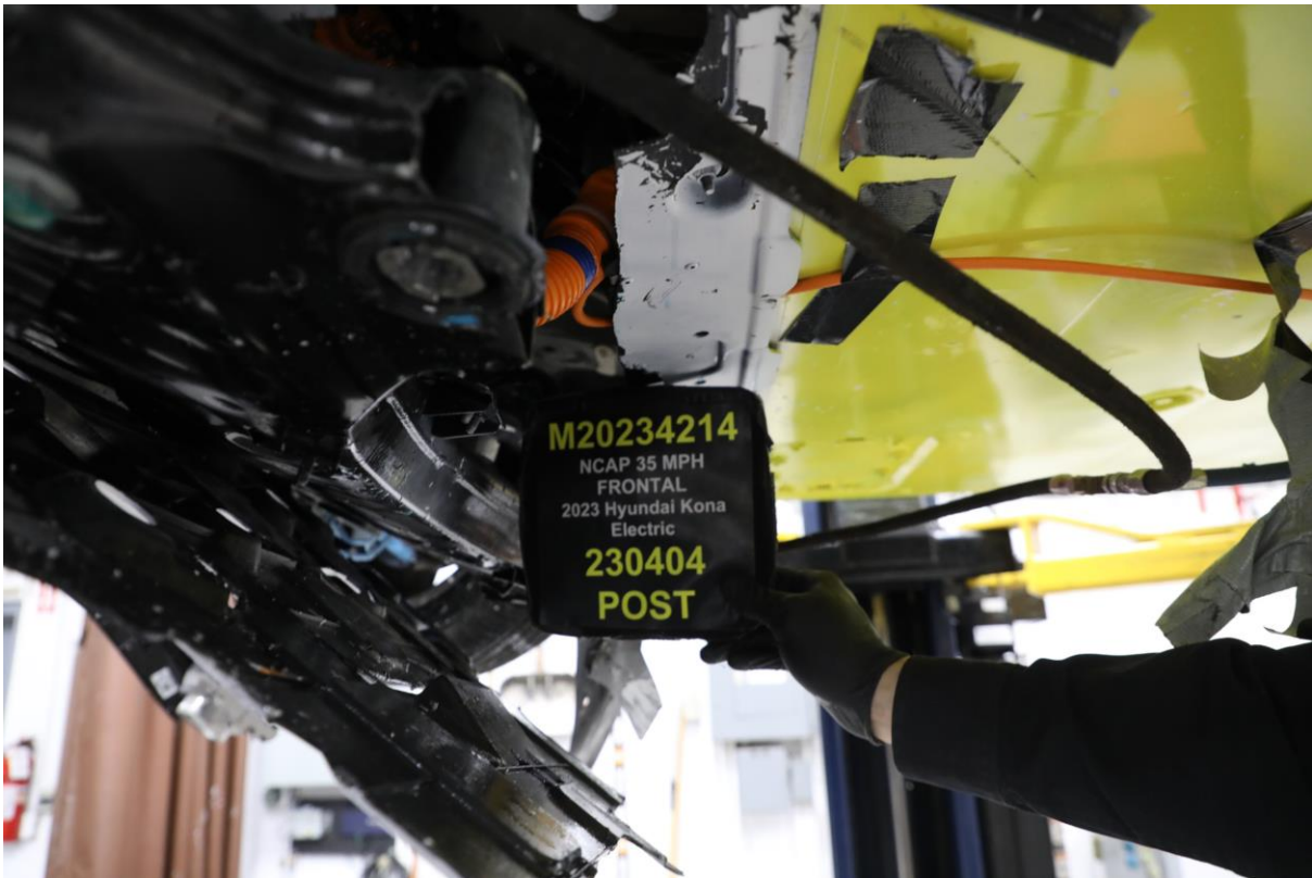
305-10 Post-Impact Front View of Propulsion Battery
