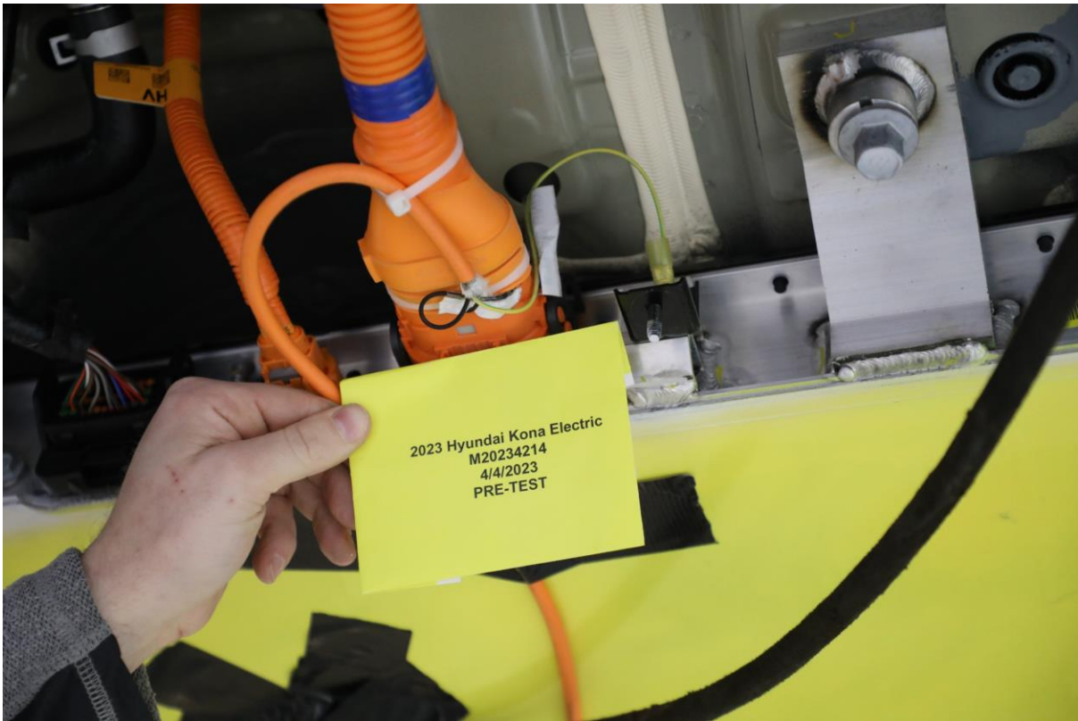
305-18 Pre-Impact View of High Voltage Interconnect(s)
