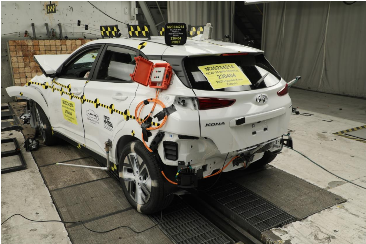
305-25 Post-Impact View of Installed Test Interface Port
