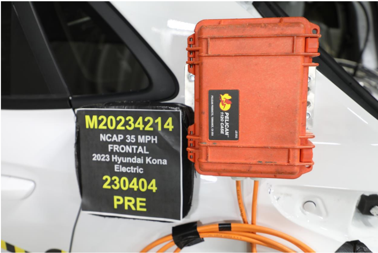
305-24 Pre-Impact View of Installed Test Interface Port
