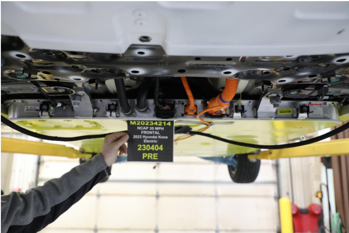
305-14 Pre-Impact View of Propulsion Battery Module(s)
