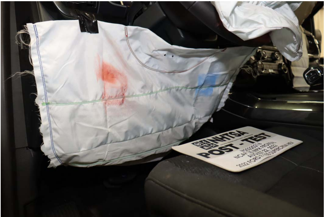
Photo No. 045 - Post-Test Driver's Side Knee Bolster
