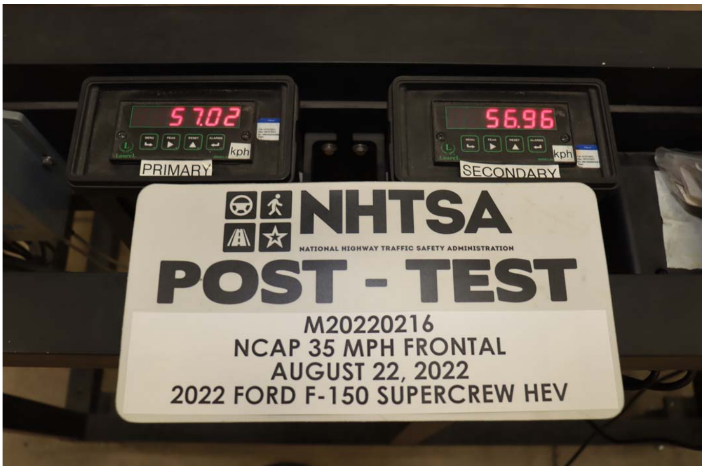
Photo No. 076 - Post-Test Speed Trap Read-Out
