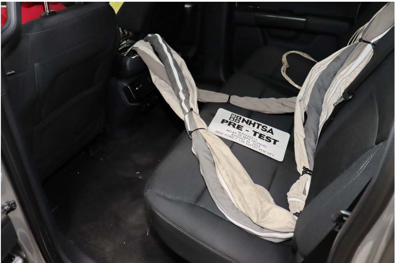
Photo No. 028 - Pre-Test Dummy Cable Routing
