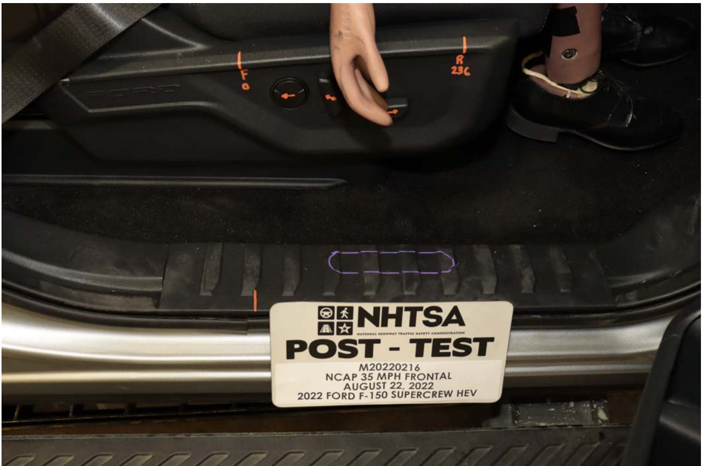
Photo No. 060 - Post-Test Passenger's Seat Fore-Aft Markings
