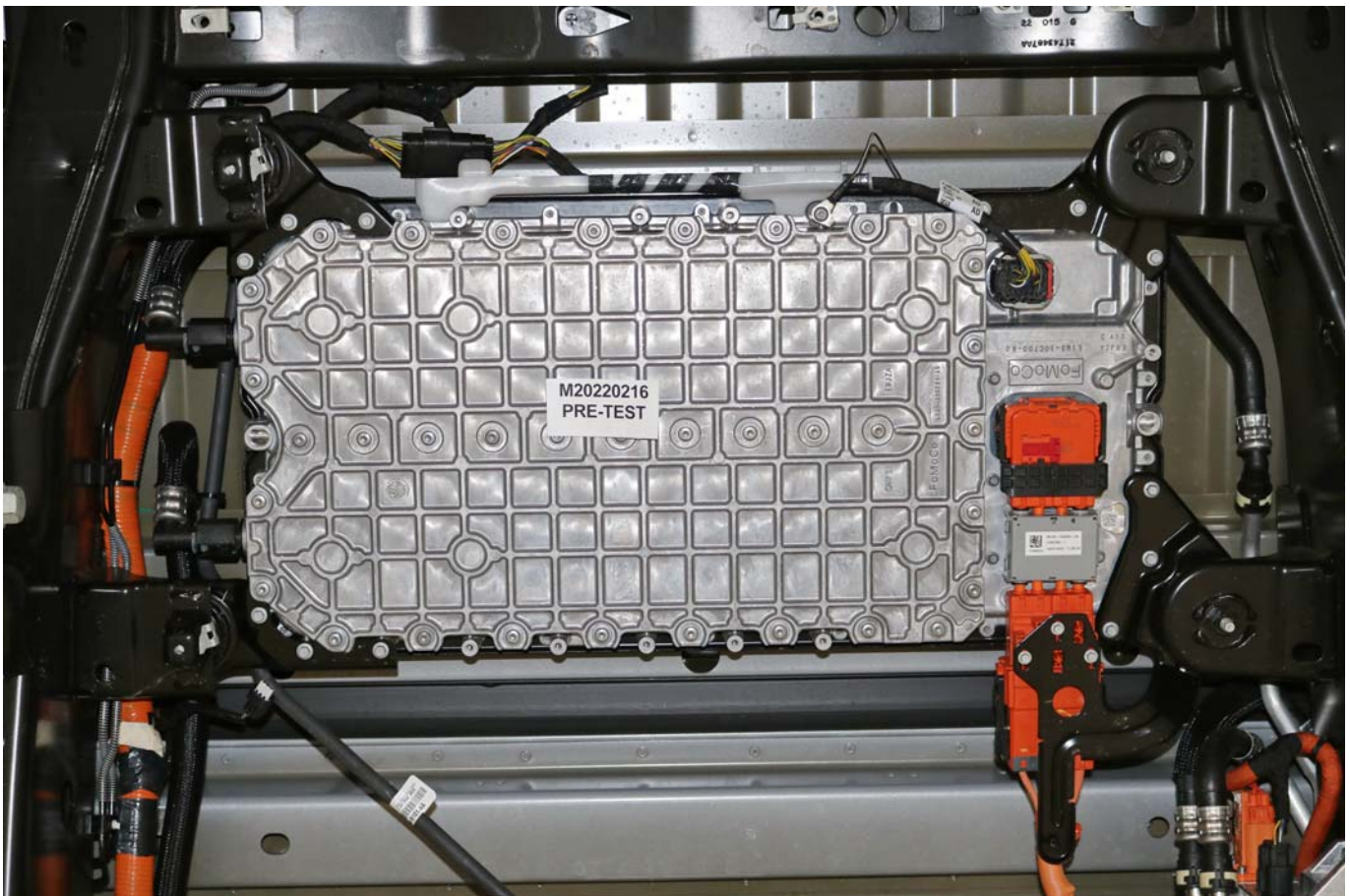
Photo No. 305-09 - Pre-Impact View of Propulsion Battery
