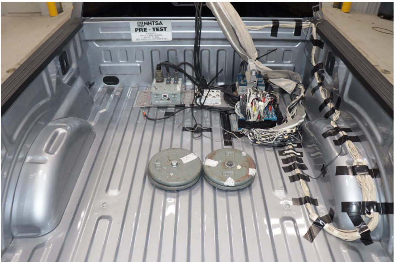
Photo No. 074 - Photograph of Ballast Installed in Vehicle
