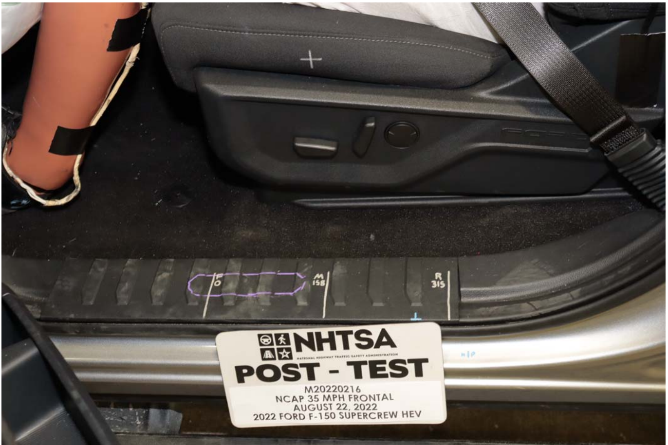
Photo No. 037 - Post-Test Driver's Seat Fore-Aft Markings
