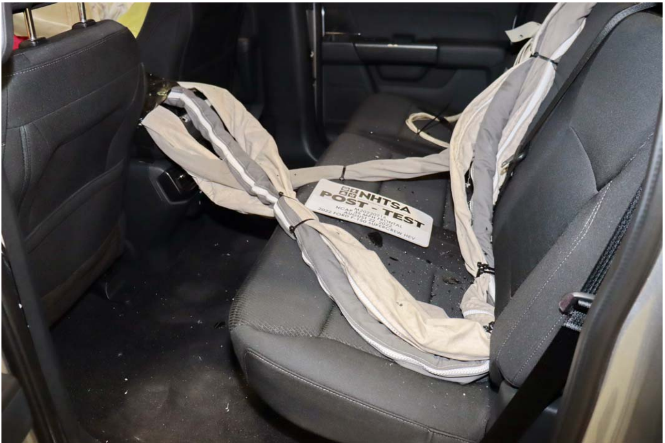
Photo No. 029 - Post-Test Dummy Cable Routing
