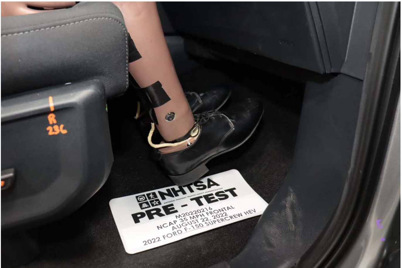
Photo No. 065 - Pre-Test Passenger Dummy Feet
