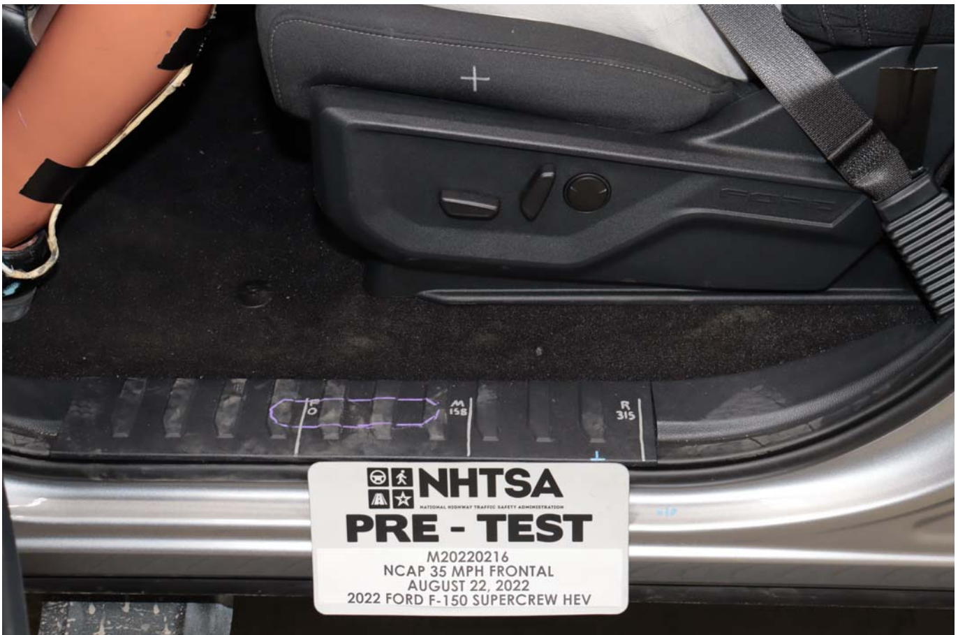
Photo No. 036 - Pre-Test Driver's Seat Fore-Aft Markings
