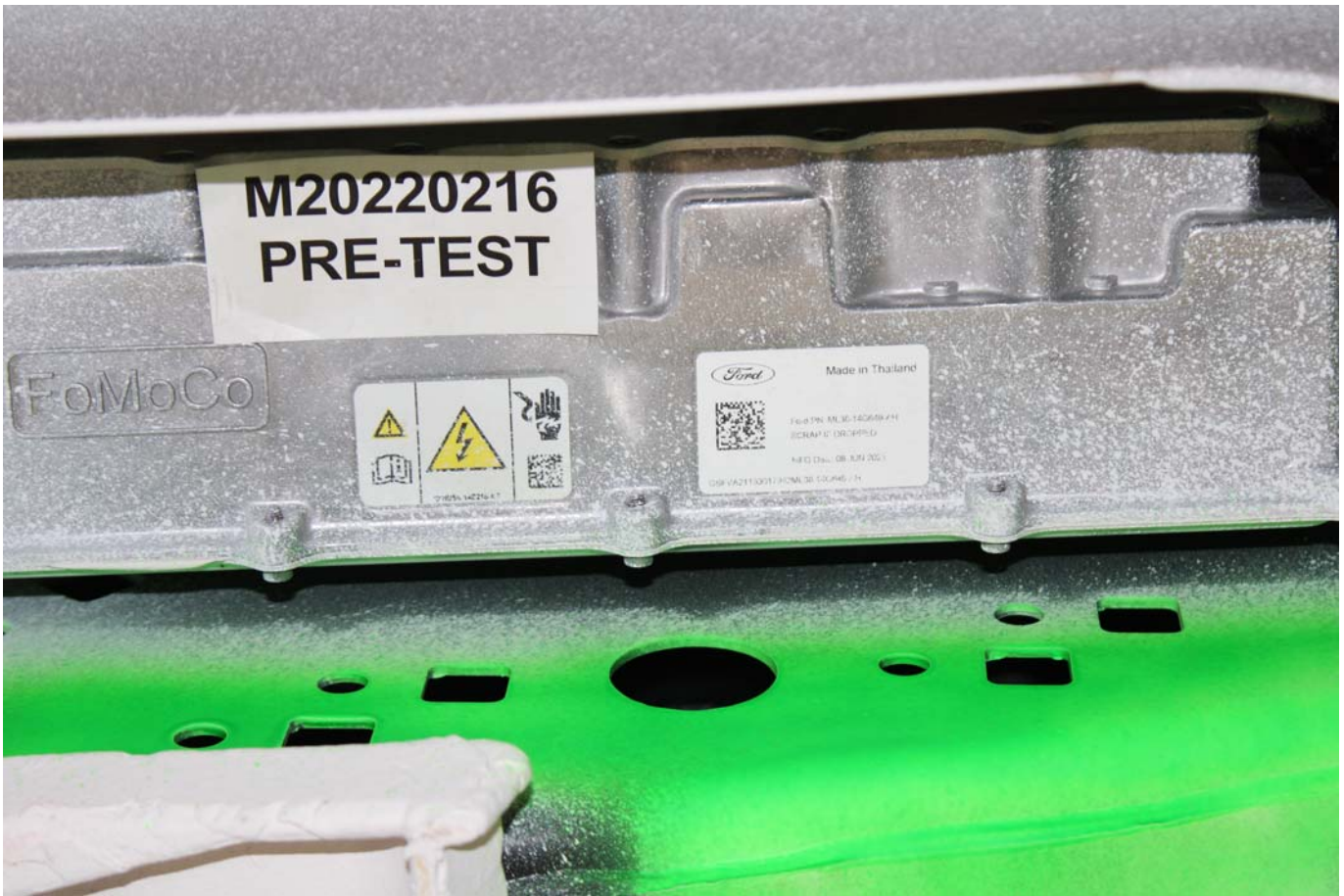
Photo No. 305-02 - Power Inverter Warning Label
