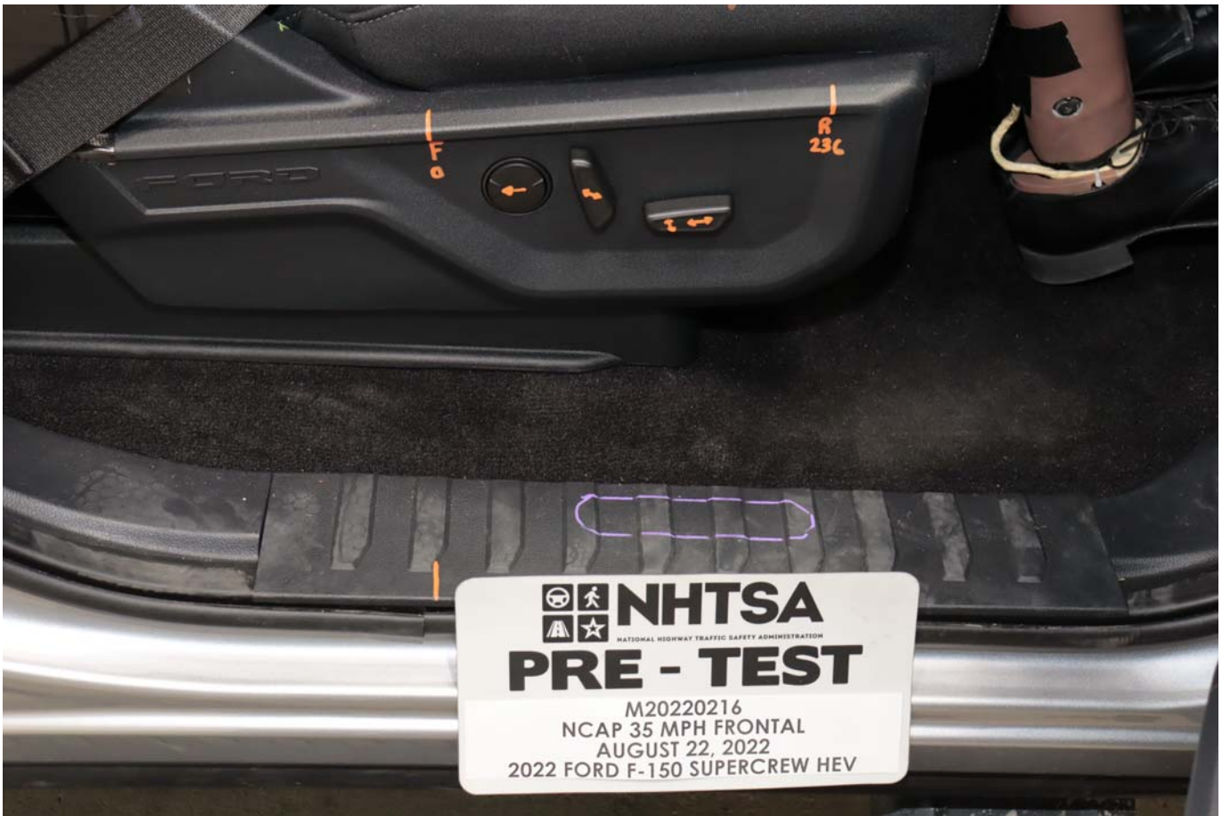
Photo No. 059 - Pre-Test Passenger's Seat Fore-Aft Markings
