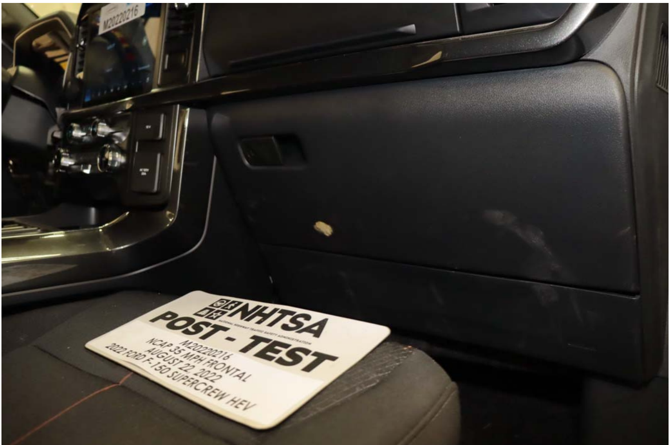
Photo No. 068 - Post-Test Passenger's Side Knee Bolster
