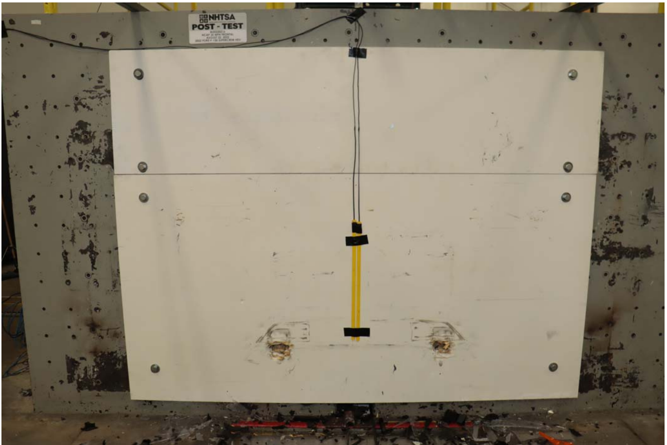
Photo No. 003 - Post-Test Load Cell Wall
