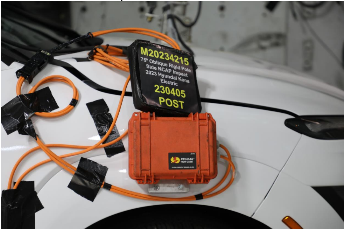
305-25 Post-Impact View of Installed Test Interface Port
