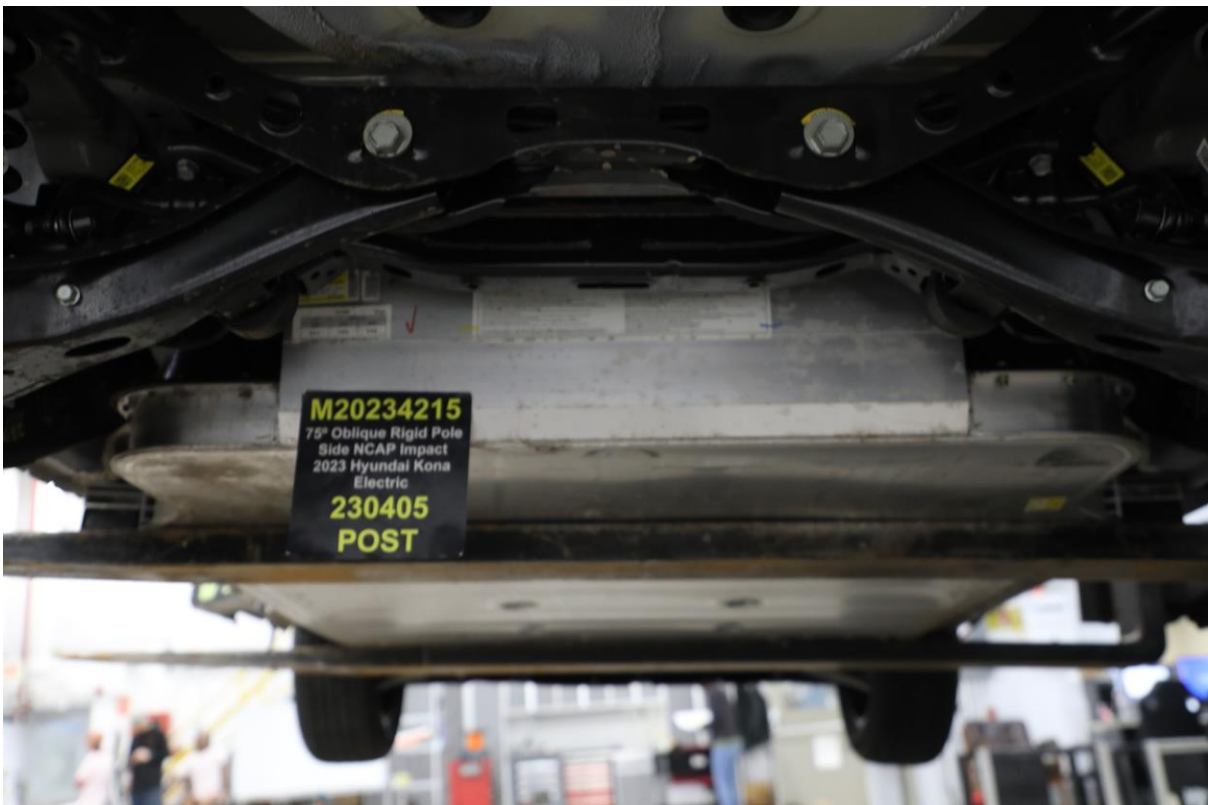
305-11 Post-Impact Rear View of Propulsion Battery
