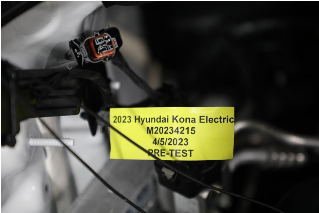
305-08 Manual High Voltage Service Disconnect Removed
