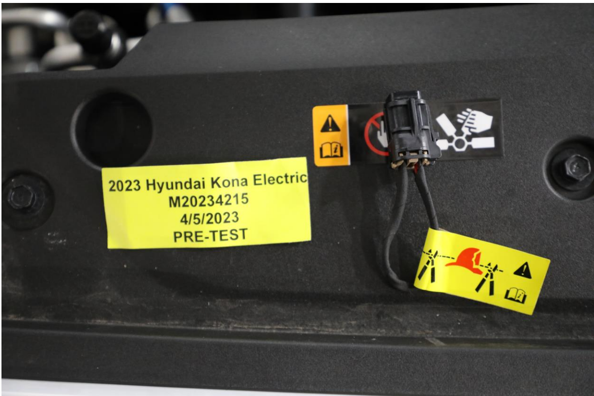
305-07 Manual High Voltage Service Disconnect Removed
