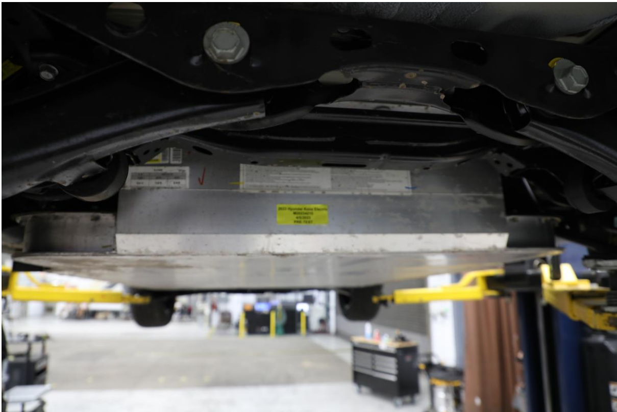
305-14 Pre-Impact View of Propulsion Battery Module(s)
