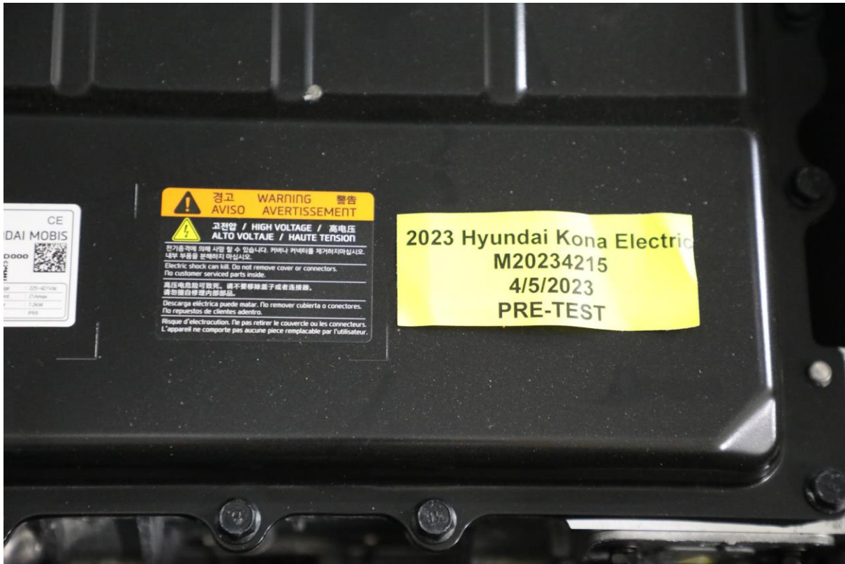
305-02 Power Inverter Warning Label
