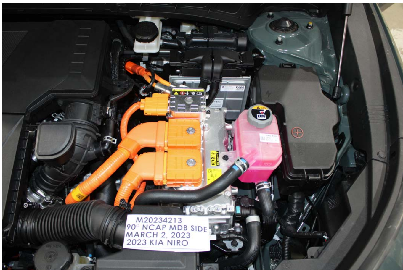
Photo No. 305-02 - Power Inverter Warning Label
