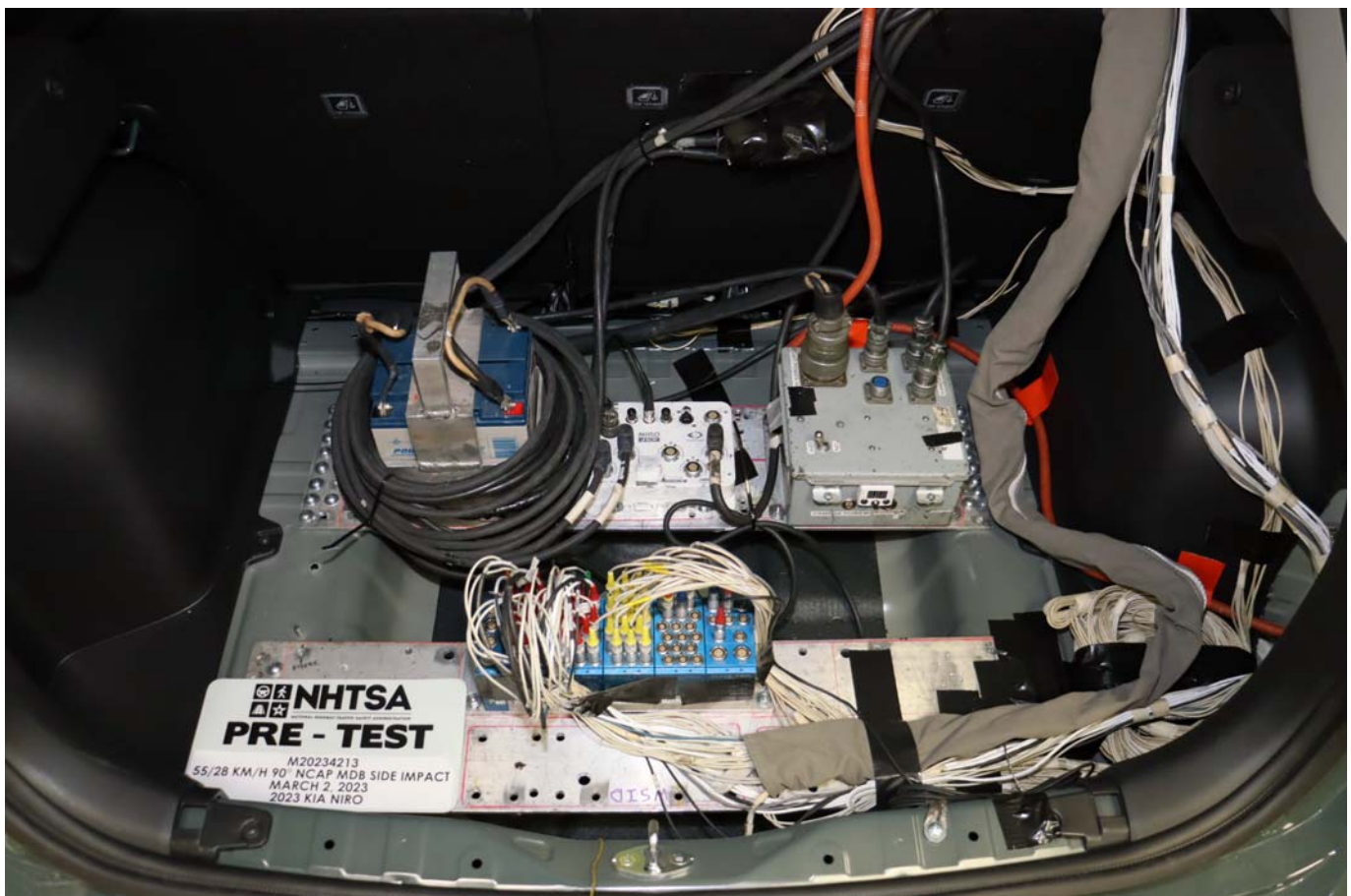
Photo No. 094 - Pre-Test Ballast View
