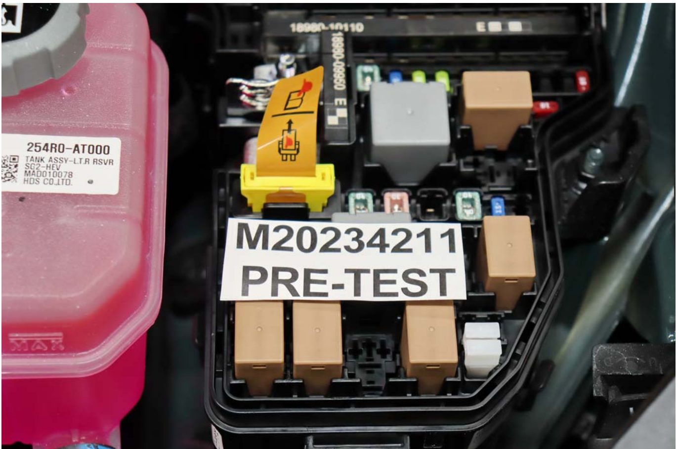
Photo No. 305-03 - First Responder Warning Label
