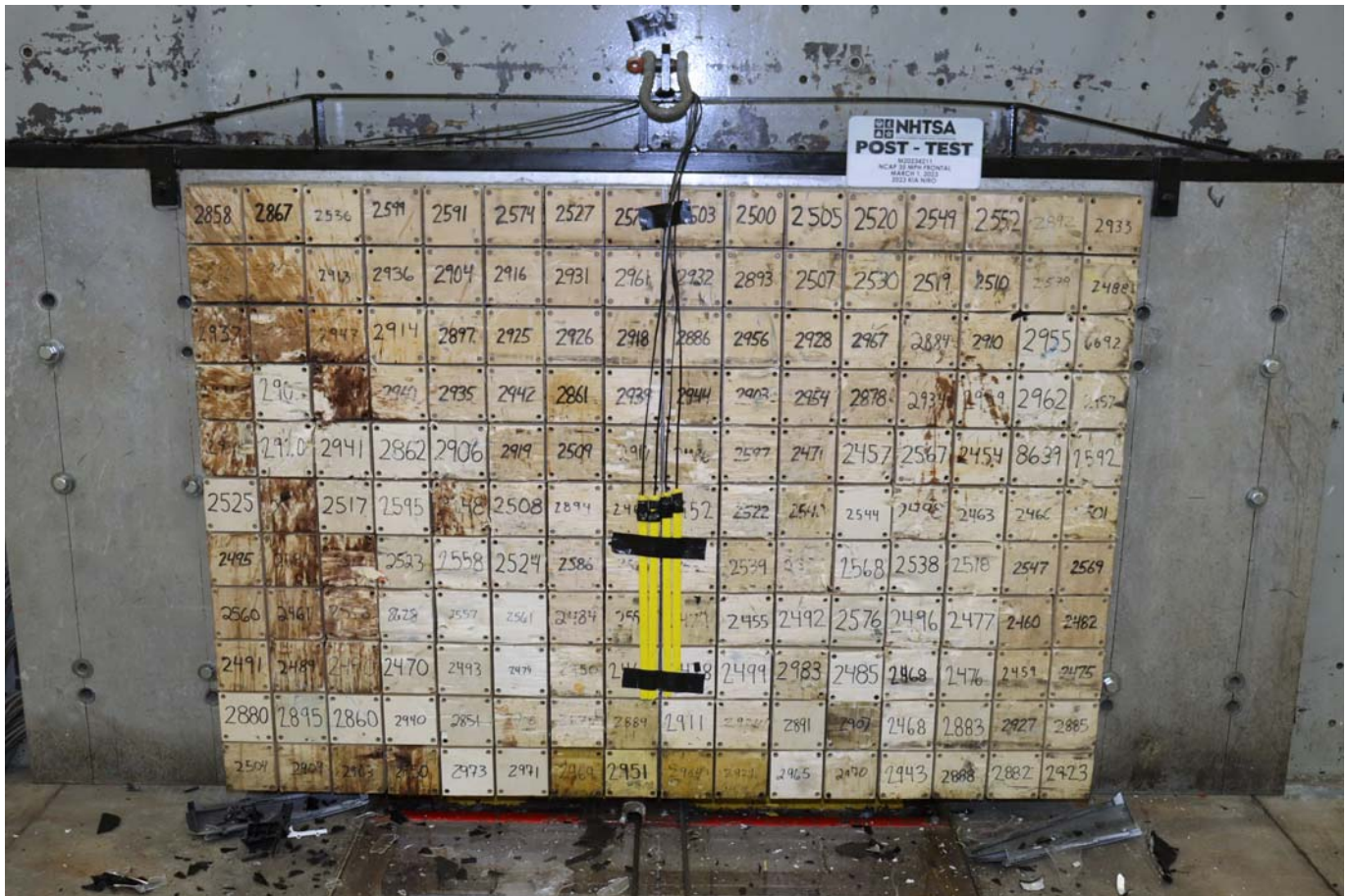
Photo No. 003 - Post-Test Load Cell Wall
