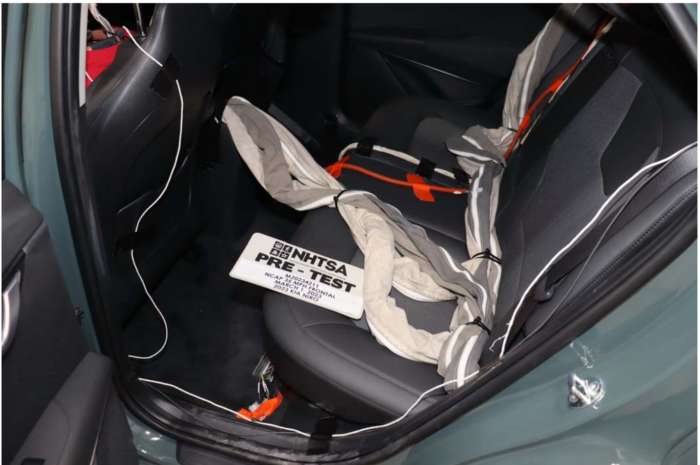
Photo No. 028 - Pre-Test Dummy Cable Routing
