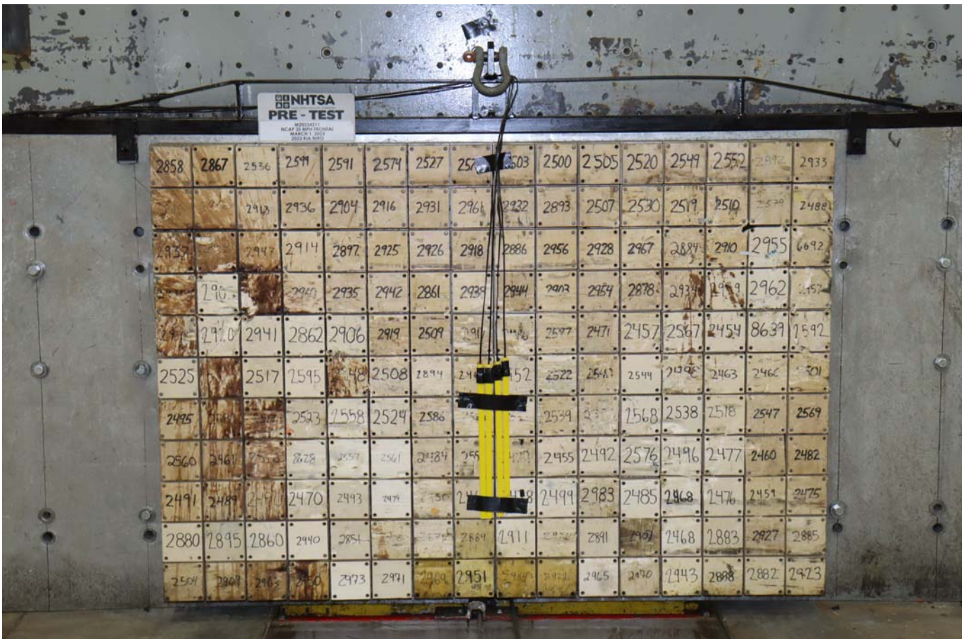
Photo No. 002 - Pre-Test Load Cell Wall
