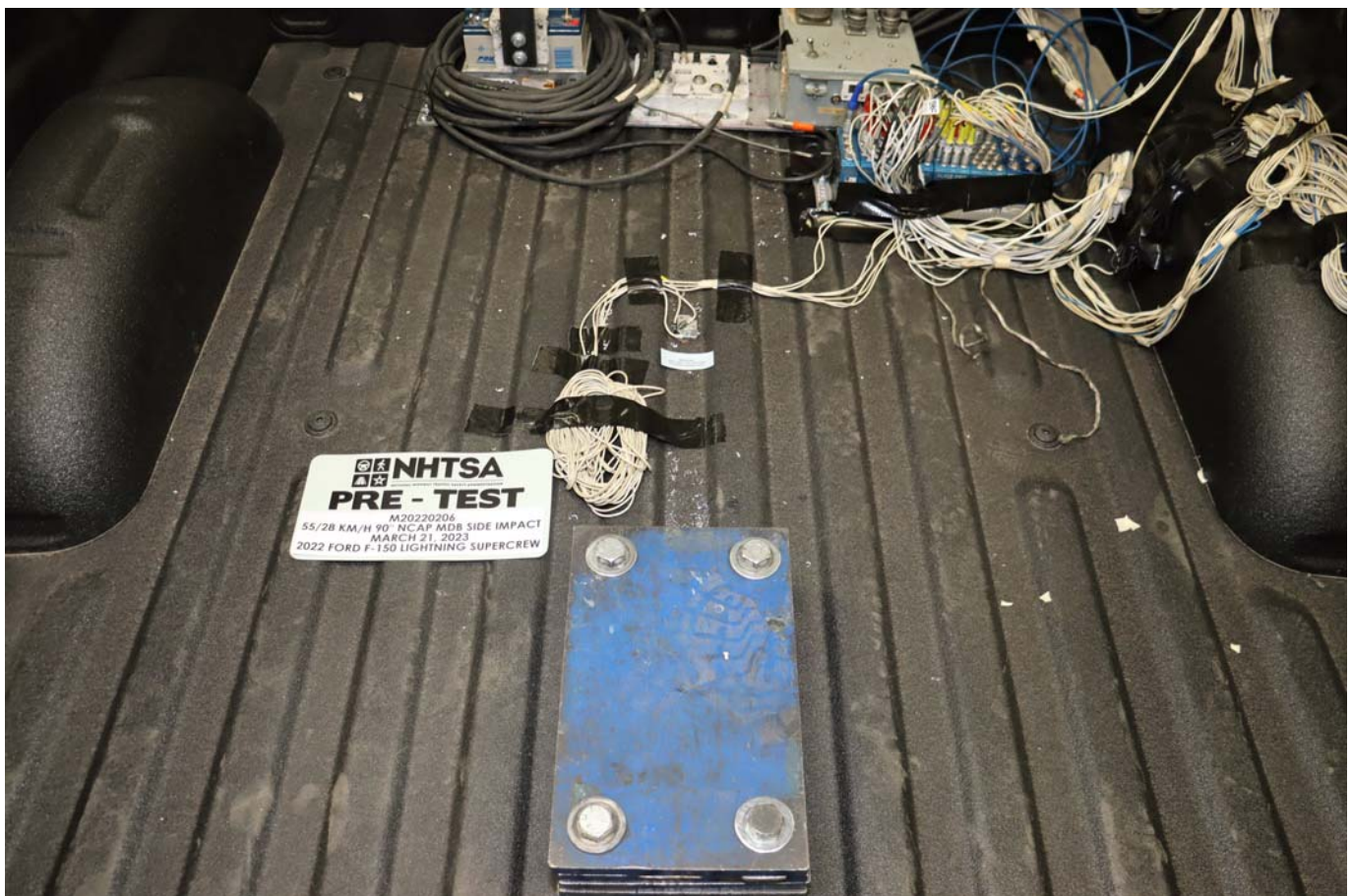
Photo No. 094 - Pre-Test Ballast View
