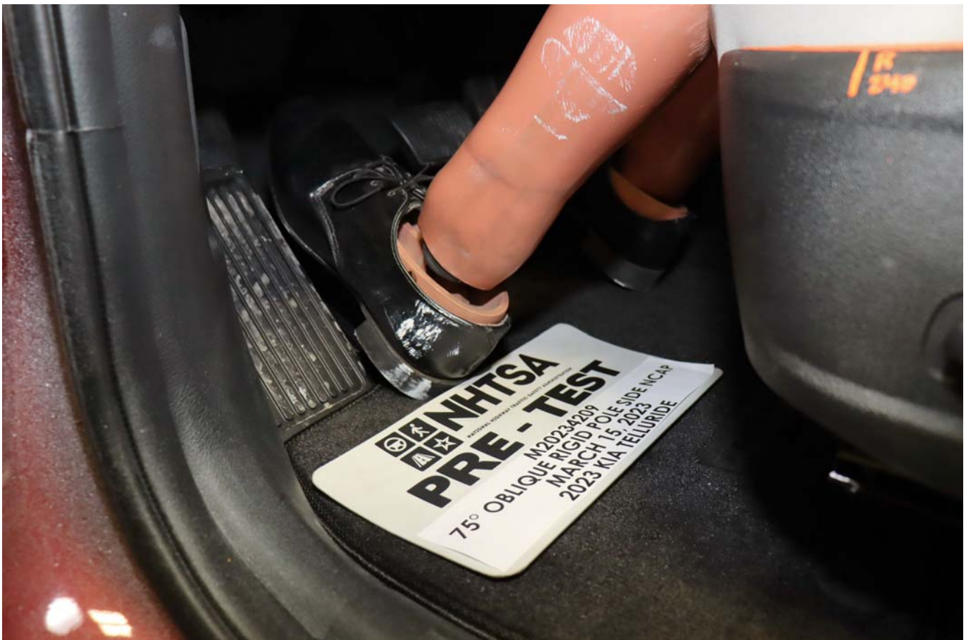
Photo No. 032 - Pre-Test Placement of Dummy's Feet
