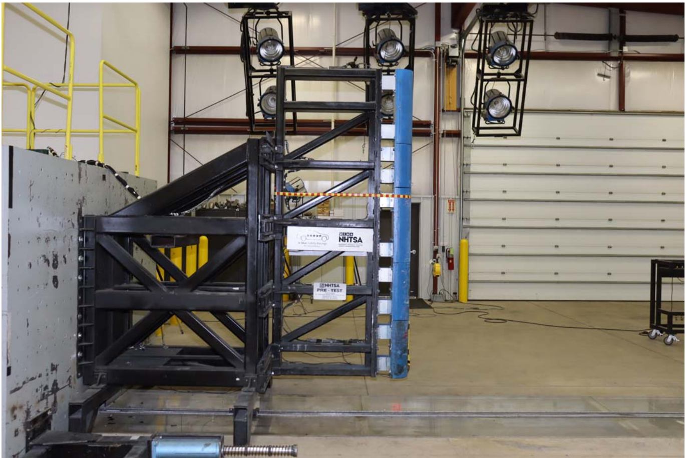
Photo No. 061 - Pre-Test Pole Barrier Side View
