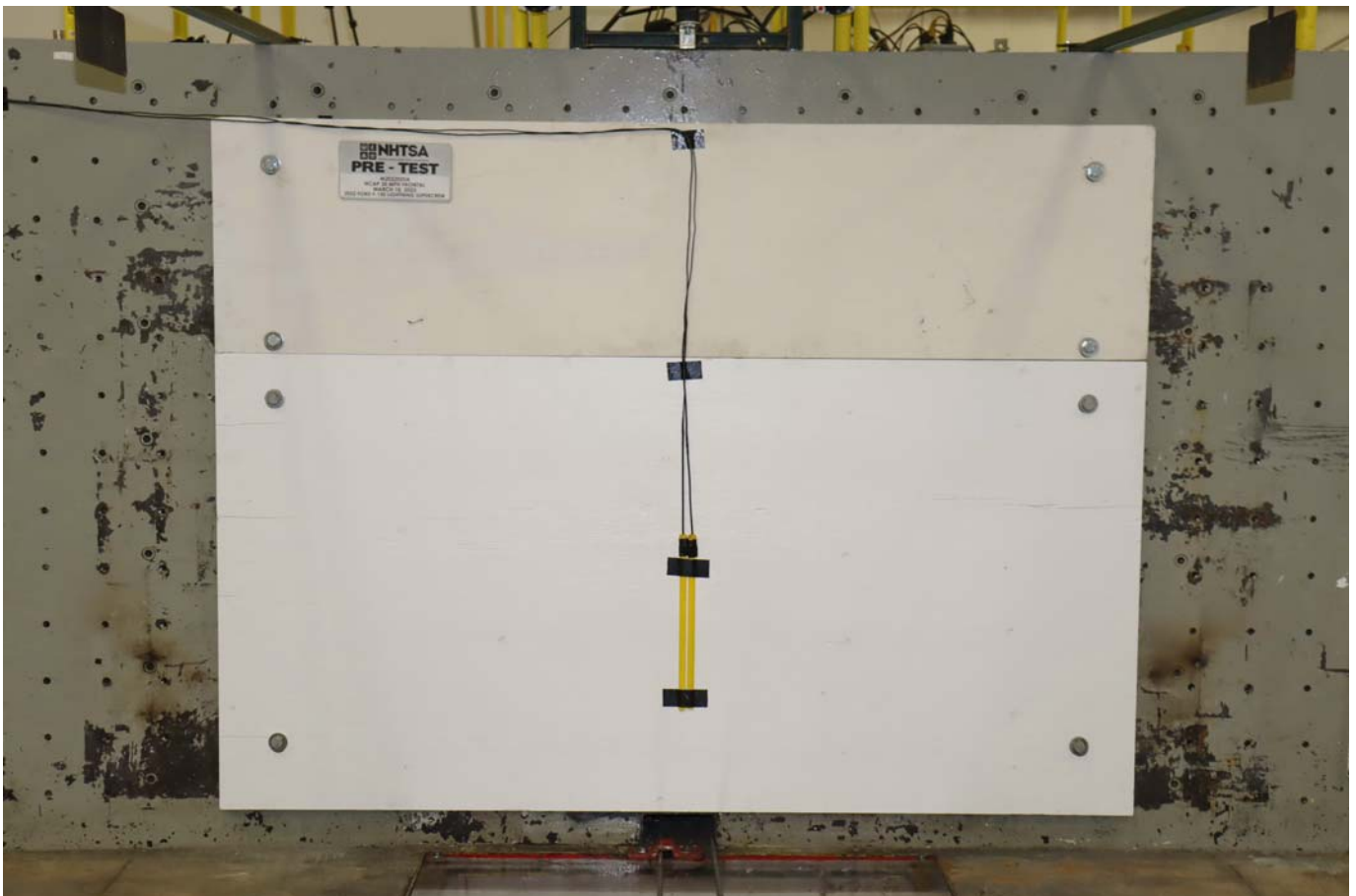
Photo No. 002 - Pre-Test Load Cell Wall
