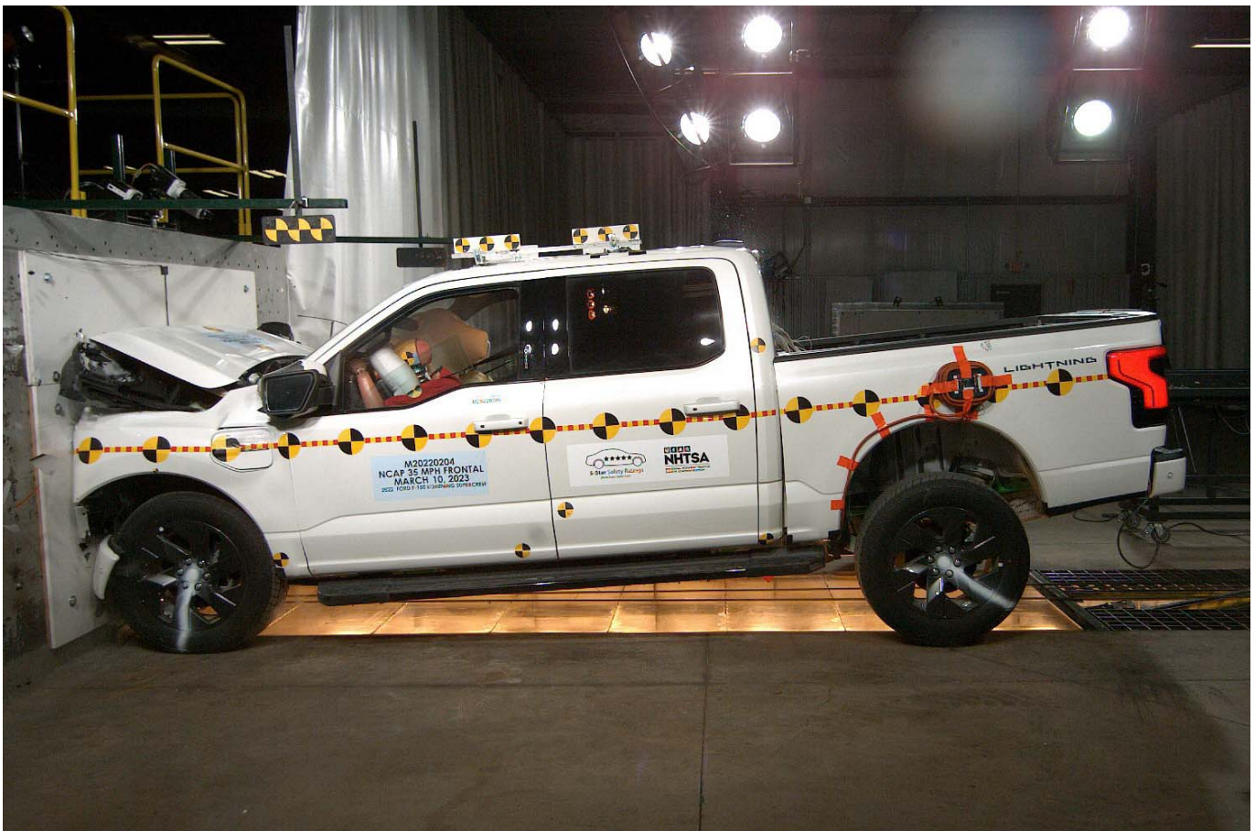
Photo No. 082 - 2022 Ford F-150 Lightning 4x4 SuperCrew Truck Frontal Impact Event
