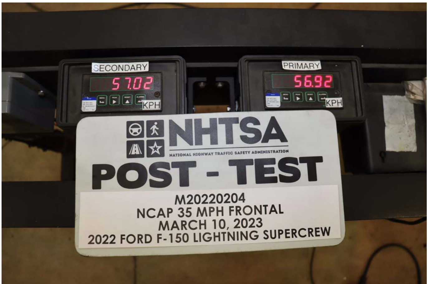
Photo No. 076 - Post-Test Speed Trap Read-Out
