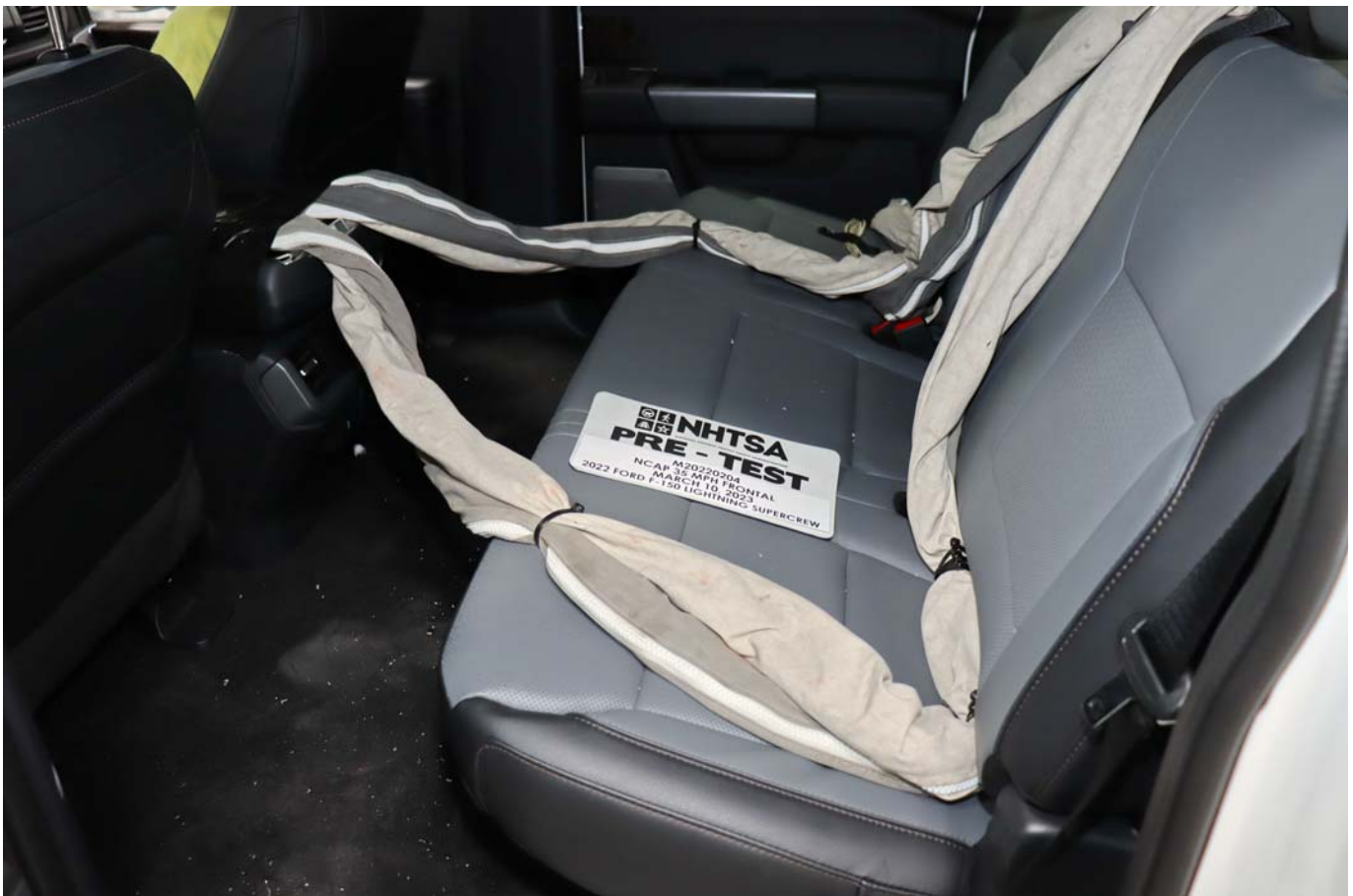
Photo No. 028 - Pre-Test Dummy Cable Routing
