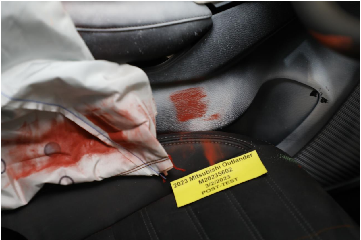
052 Post-Test Driver Dummy Close-Up Pelvis Contact View
