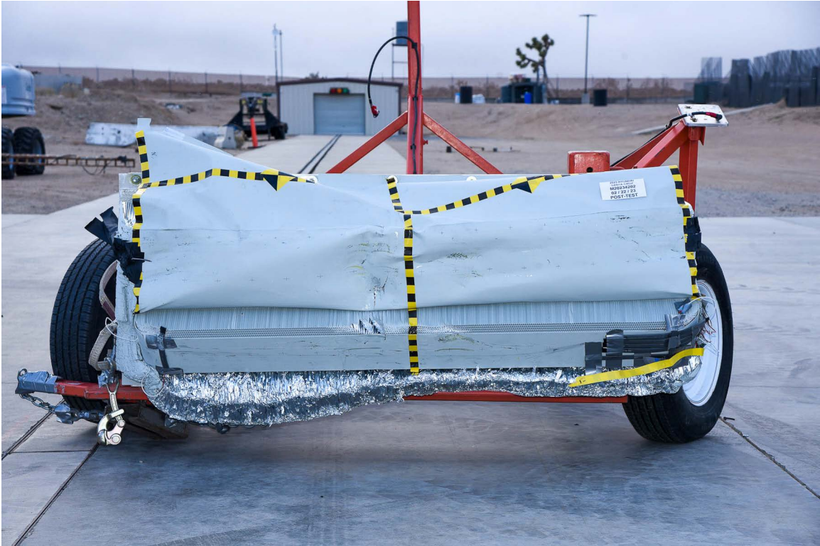
FIGURE 85. Post-Test Front View of MDB Impactor Face
