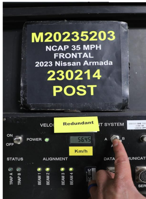
076 Post-Test Speed Trap Read out
