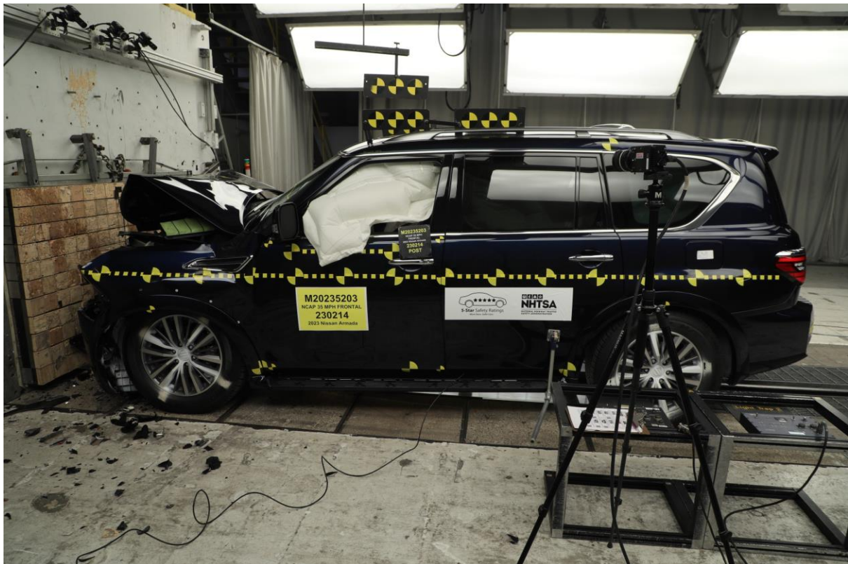
011 Post-Test Left View of Test Vehicle
