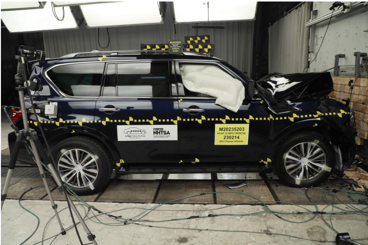
013 Post-Test Right View of Test Vehicle
