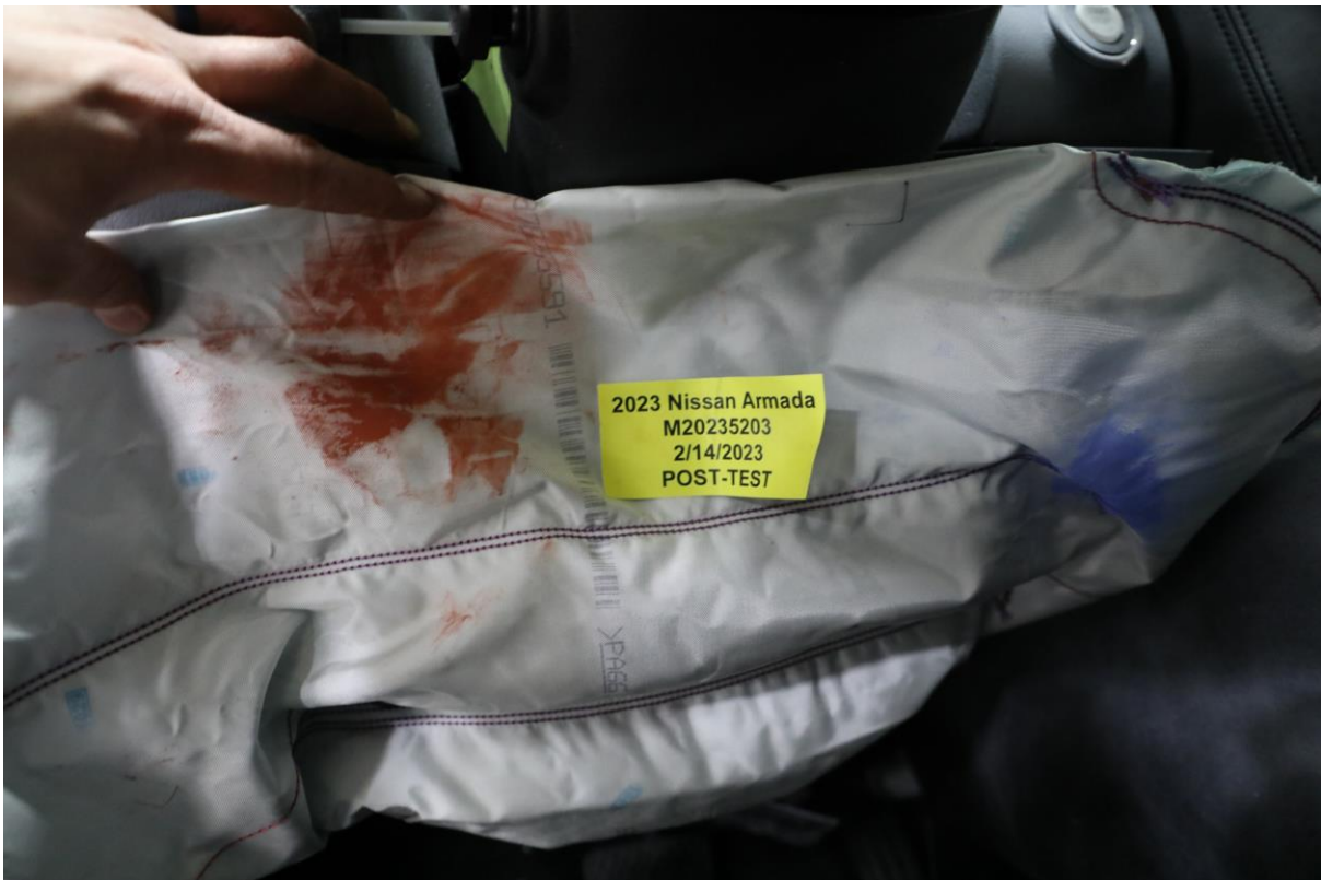
045 Post-Test Driver's Side Knee Bolster
