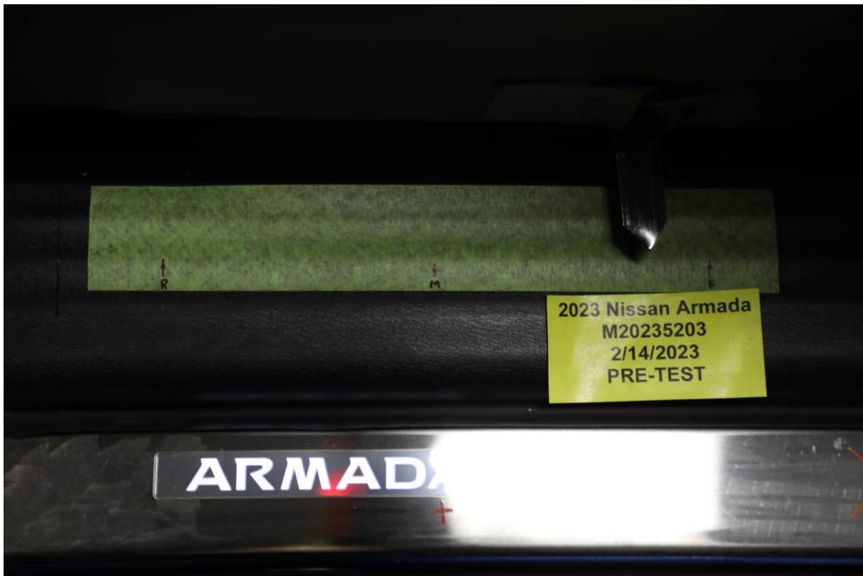
059 Pre-Test Passenger's Seat Fore-Aft Markings
