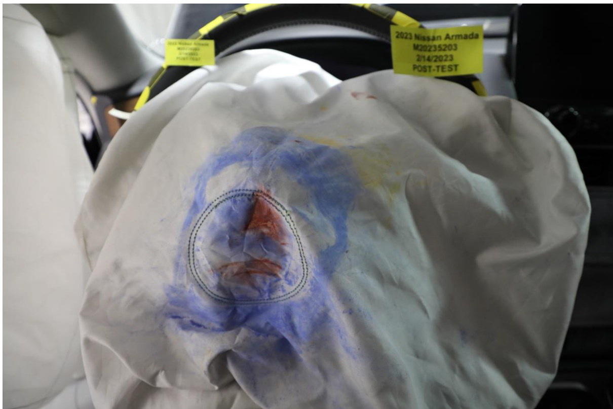
049 Post-Test Driver Dummy Contact with Airbag
