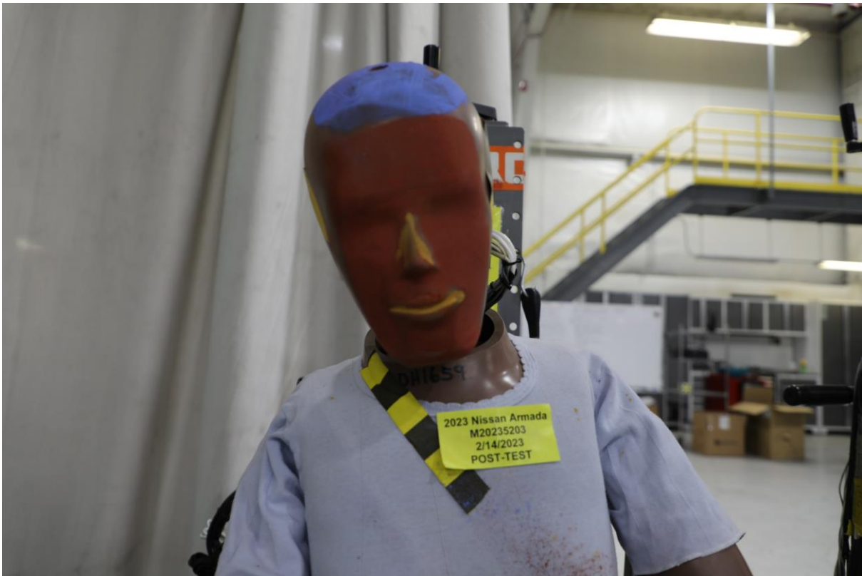
071 Post-Test Passenger Dummy Face
