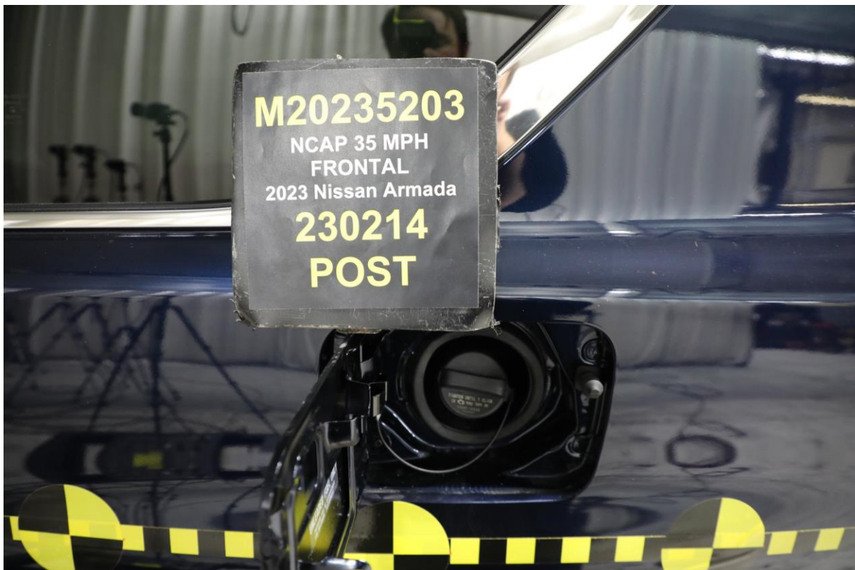
023 Post-Test Fuel Filler Cap View
