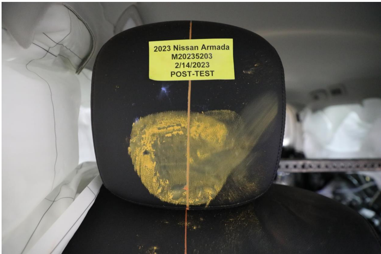
073 Post-Test Passenger Dummy Contact with Headrest
