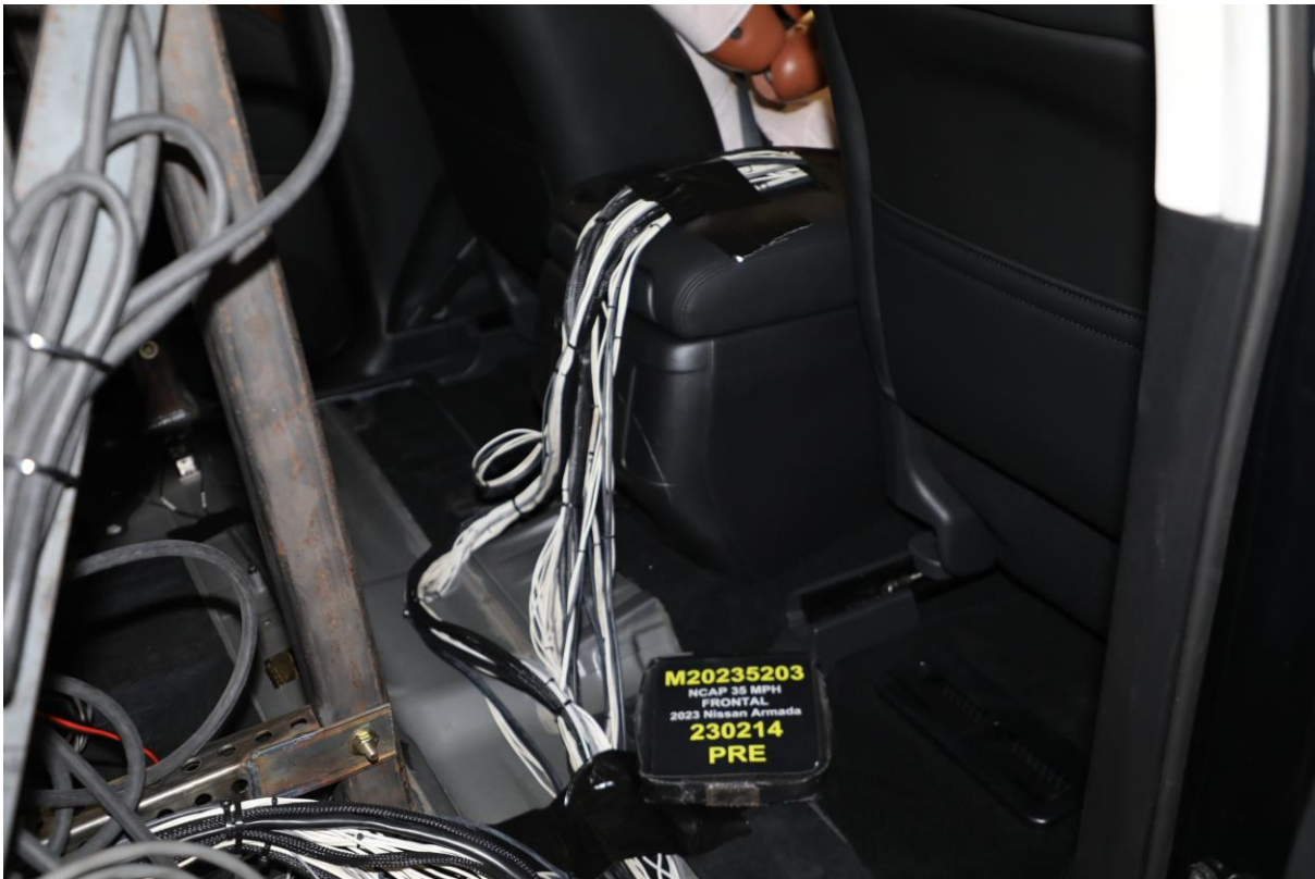
028 Pre-Test Dummy Cable Routing
