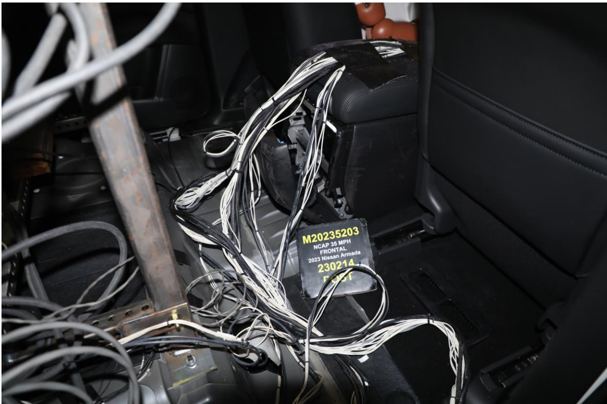
029 Post-Test Dummy Cable Routing
