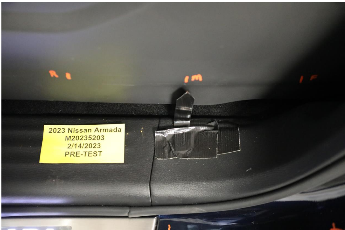
036 Pre-Test Driver's Seat Fore-Aft Markings
