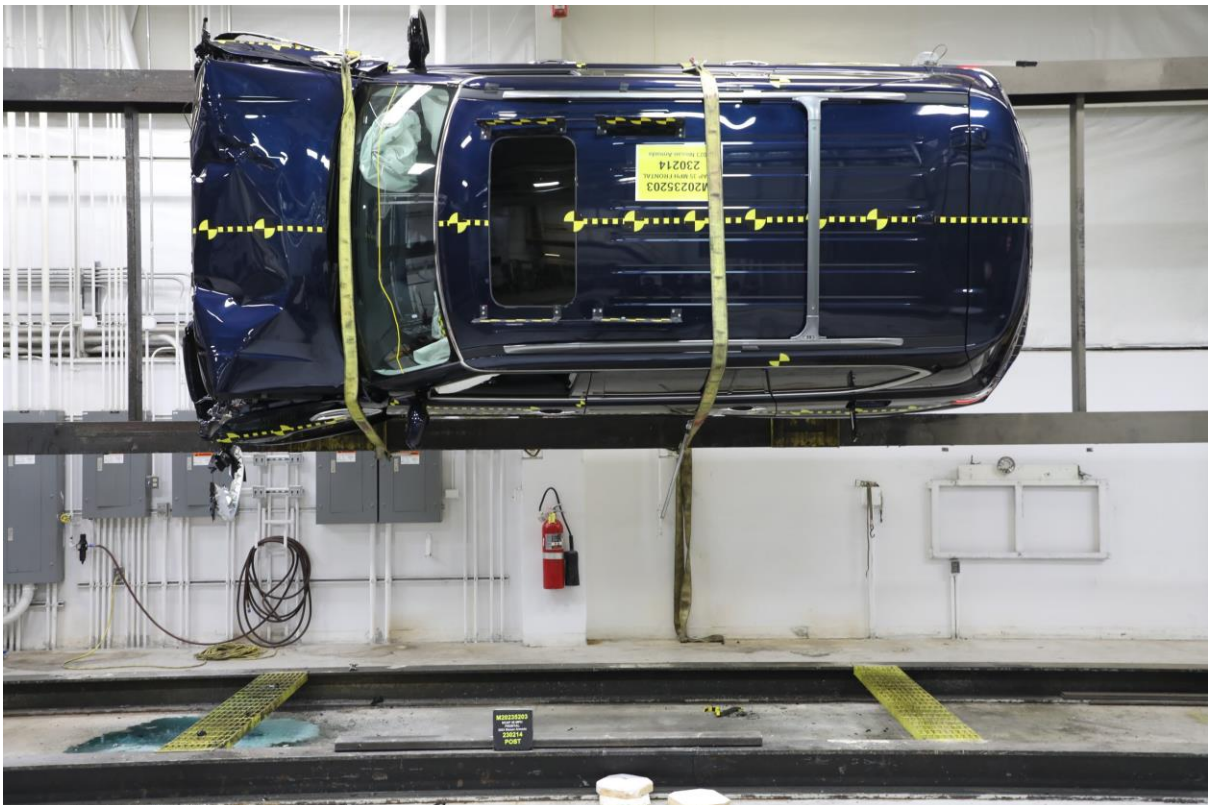
078 Vehicle at 90° on Static Rollover Device
