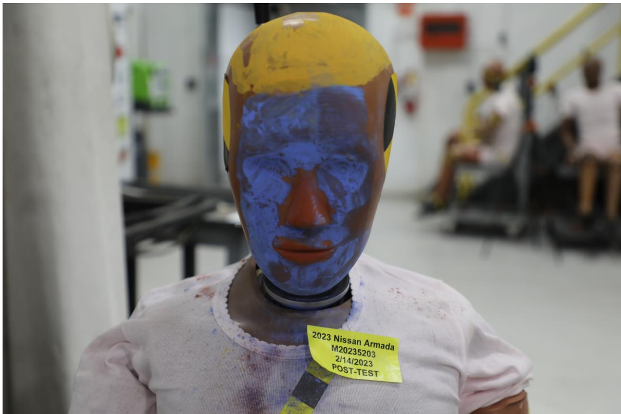
048 Post-Test Driver Dummy Face
