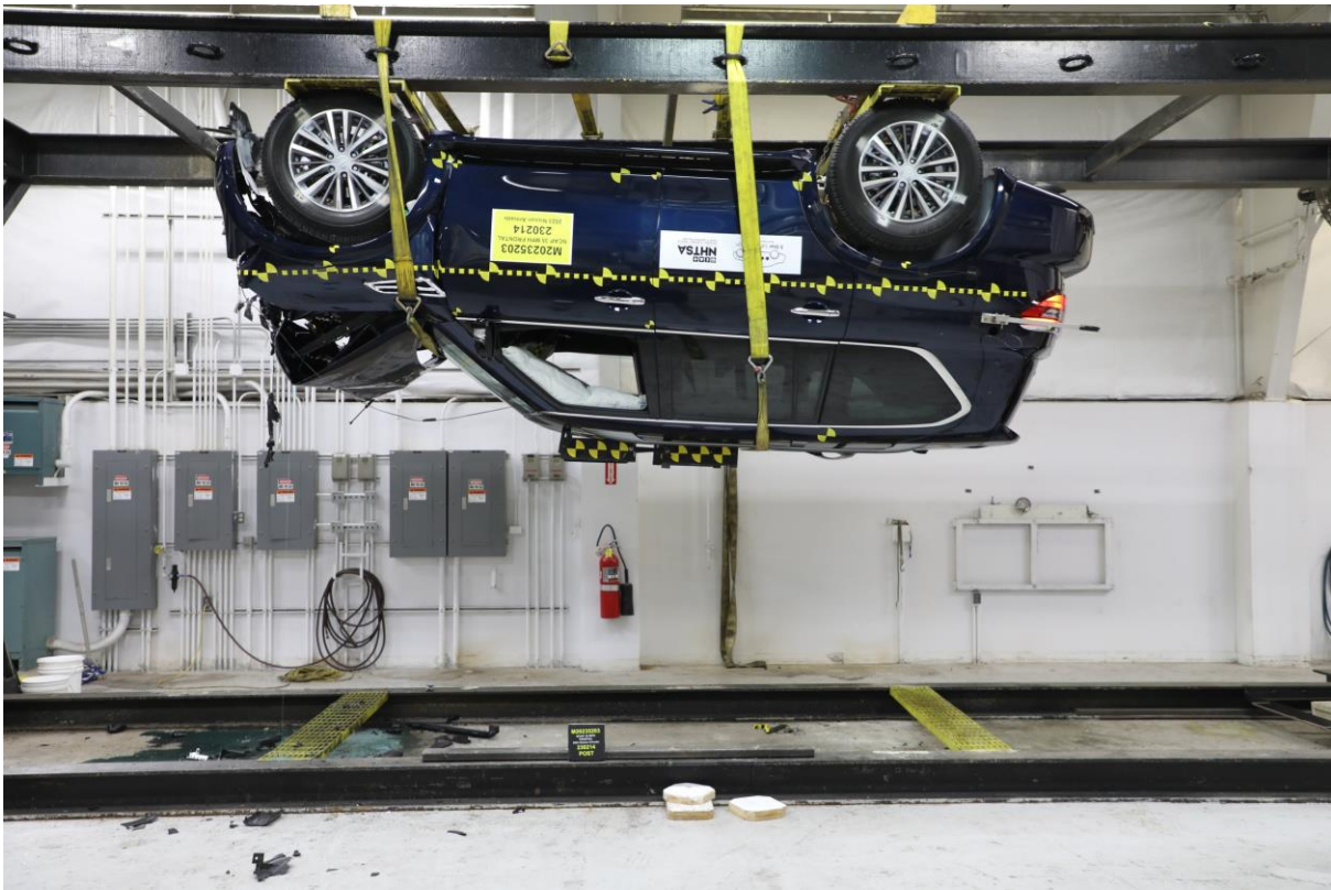
079 Vehicle at 180° on Static Rollover Device
