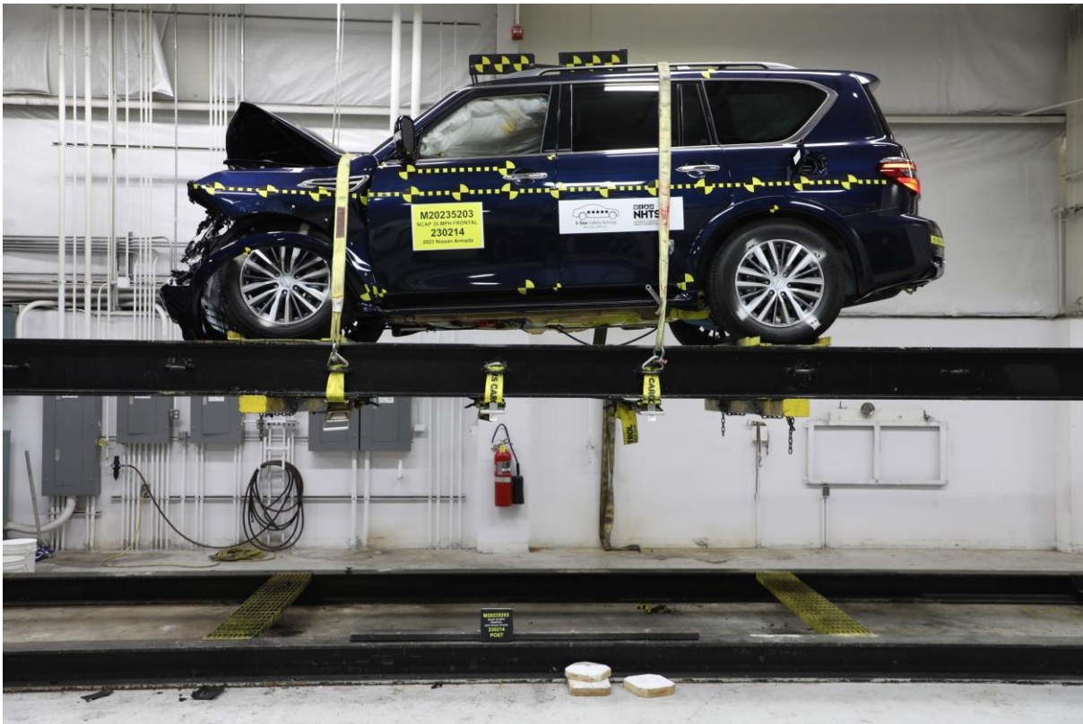
077 Vehicle at 0° on Static Rollover Device
