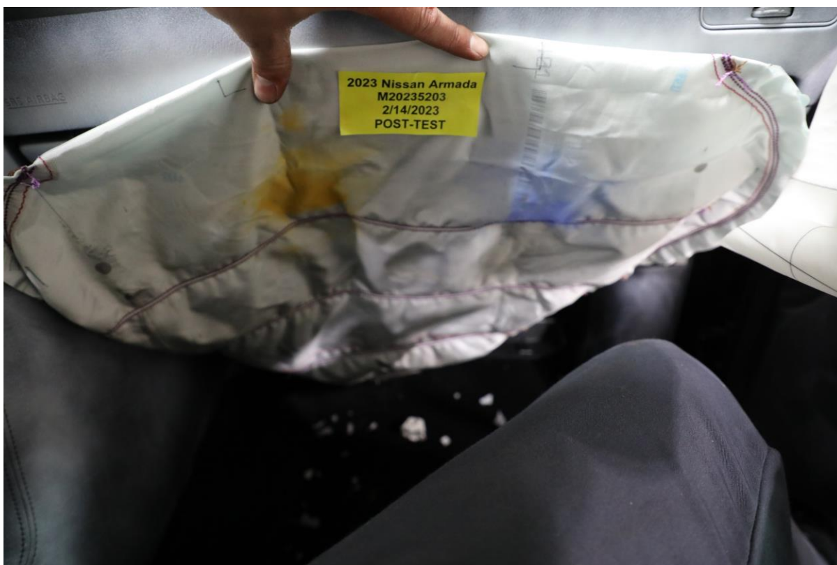
068 Post-Test Passenger's Side Knee Bolster
