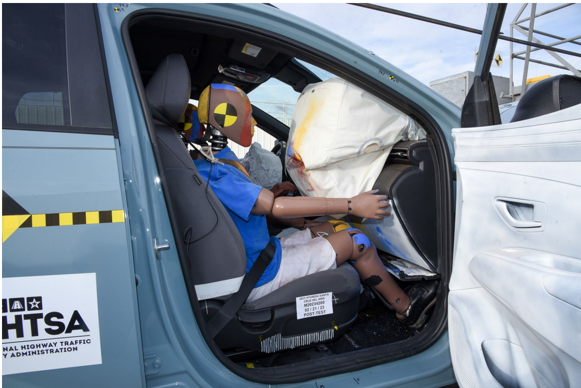
FIGURE 58. Post-Test Passenger Dummy and Vehicle Interior View
