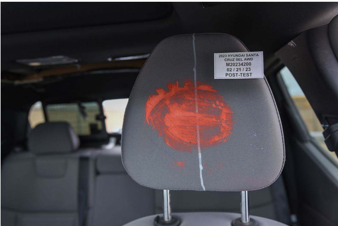
FIGURE 50. Post-Test Driver Dummy Contact with Headrest
