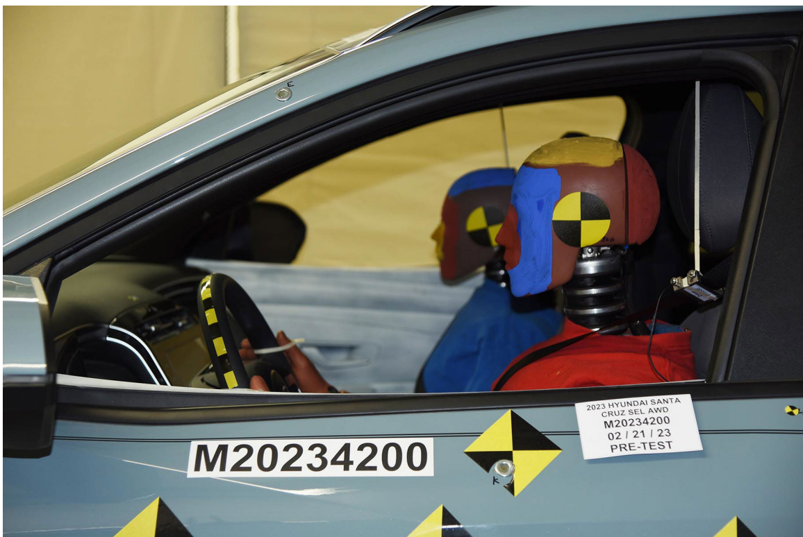
FIGURE 32. Pre-Test Driver Dummy Window View
