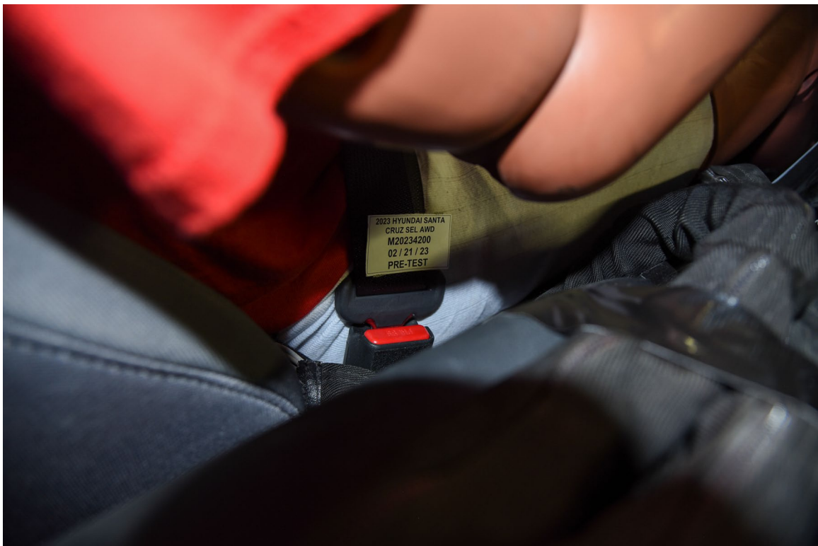
FIGURE 40. Pre-Test View of Belt Buckle and Latch Plate for Driver Dummy
