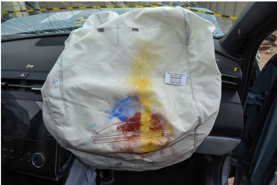
FIGURE 72. Post-Test Passenger Dummy Contact with Airbag
