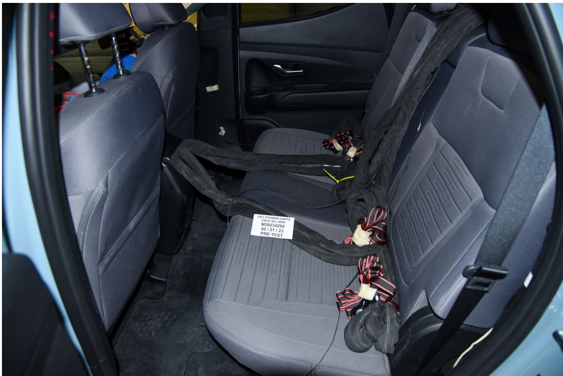
FIGURE 28. Pre-Test Dummy Cable Routing
