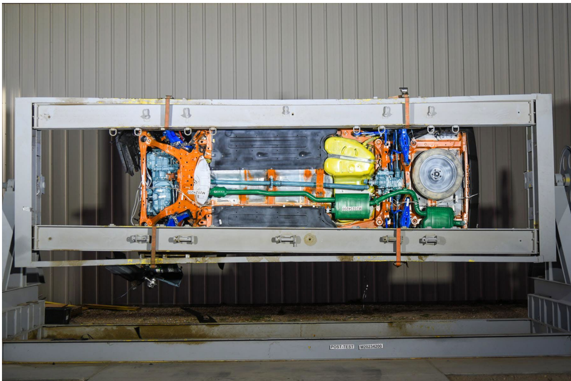
FIGURE 80. Vehicle at 270° on Static Rollover Device
