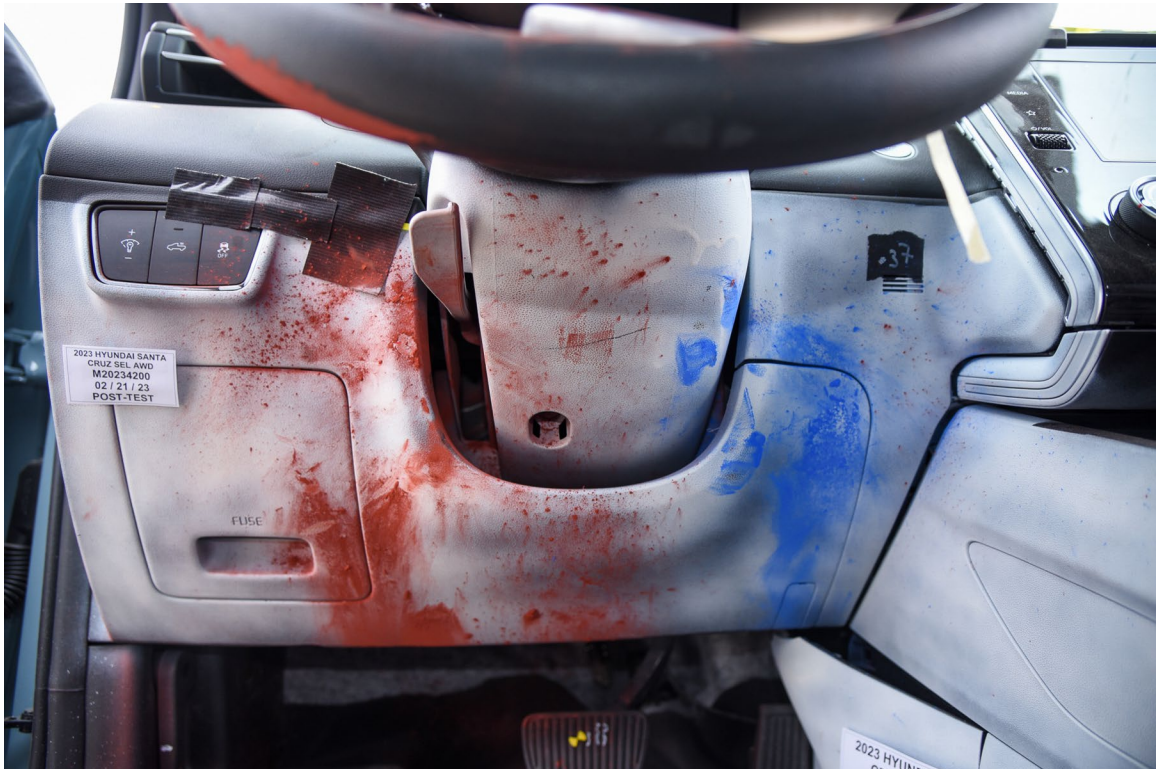
FIGURE 45. Post-Test Driver's Side Knee Bolster
