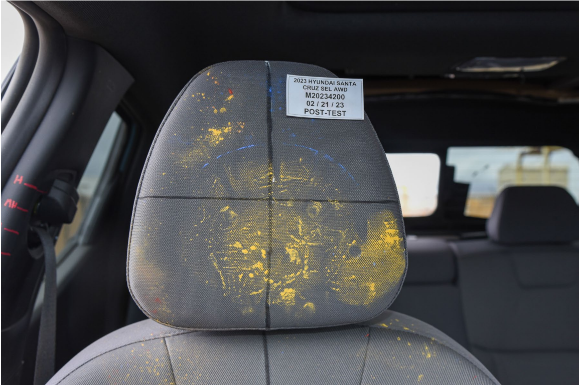
FIGURE 73. Post-Test Passenger Dummy Contact with Headrest
