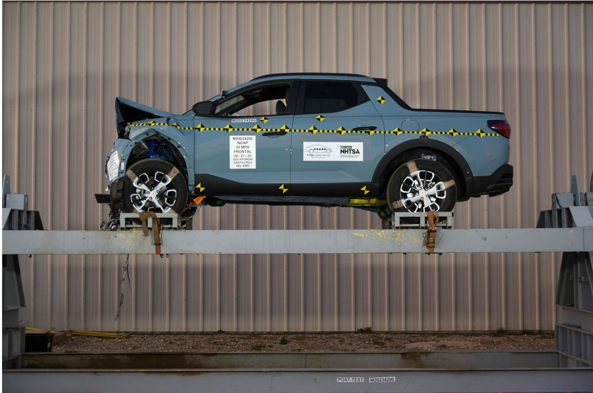
FIGURE 77. Vehicle at 0° on Static Rollover Device
