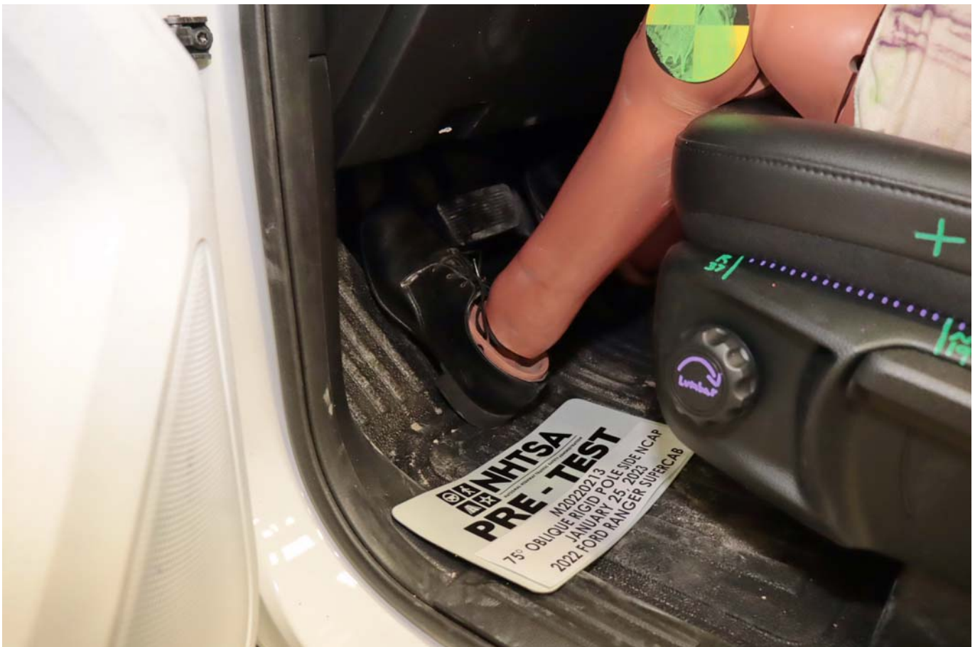
Photo No. 032 - Pre-Test Placement of Dummy's Feet
