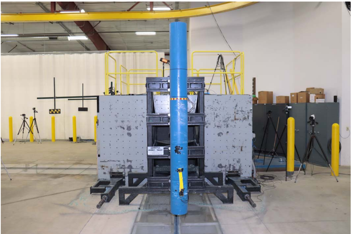
Photo No. 060 - Post-Test Pole Barrier Front View
