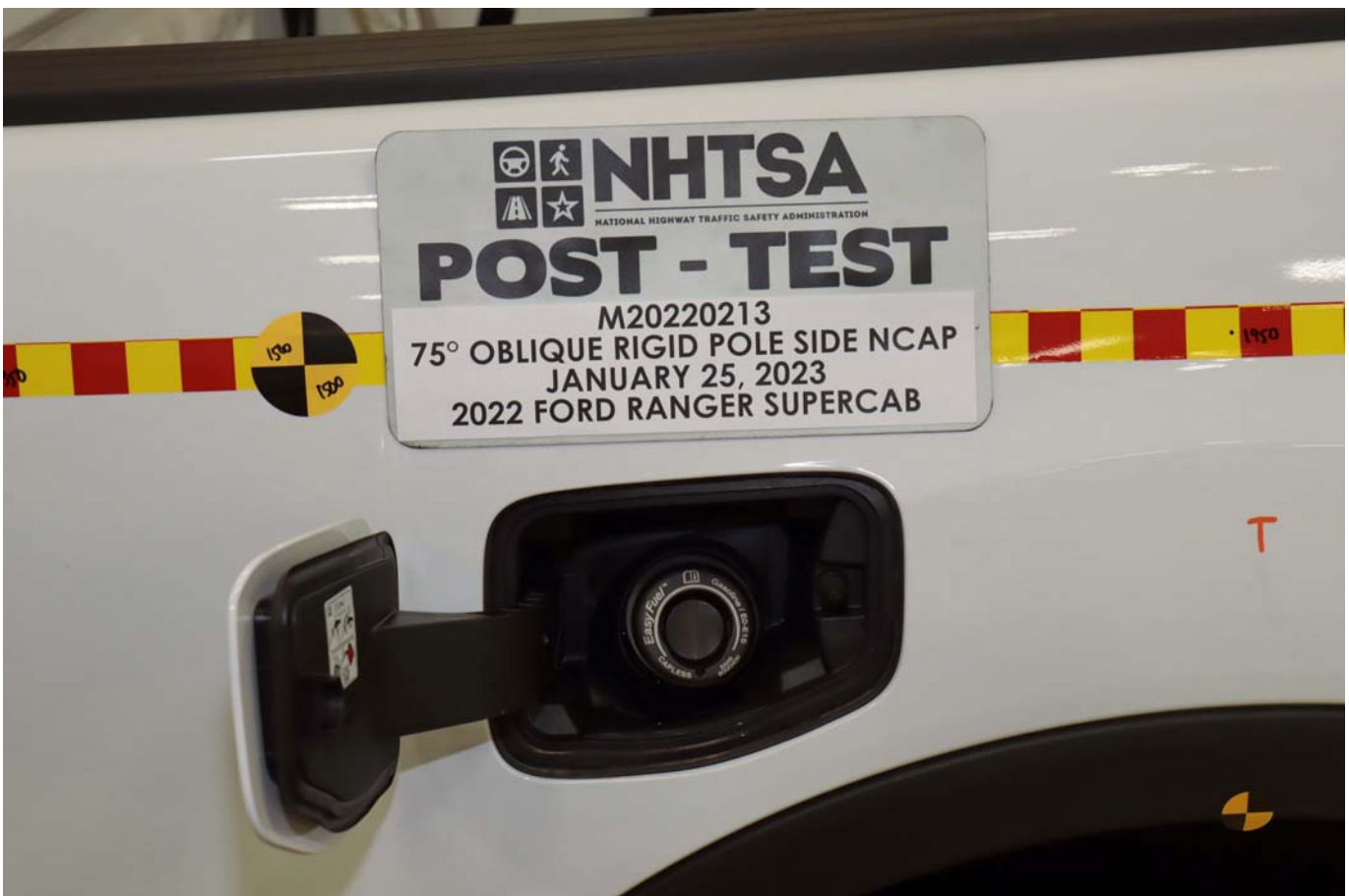
Photo No. 056 - Post-Test View of Fuel Filler Cap or Fuel Filler Neck
