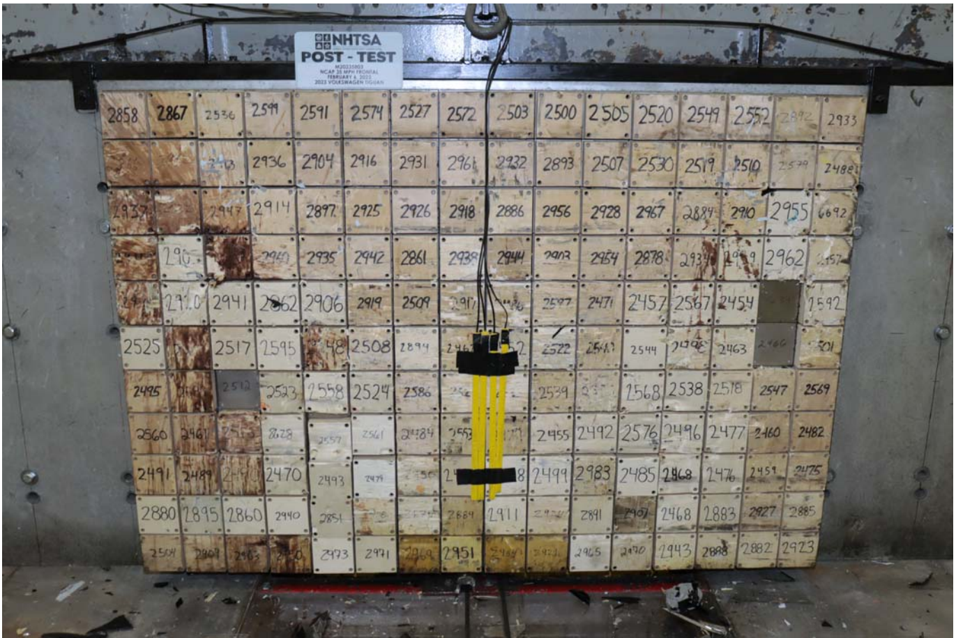
Photo No. 003 - Post-Test Load Cell Wall
