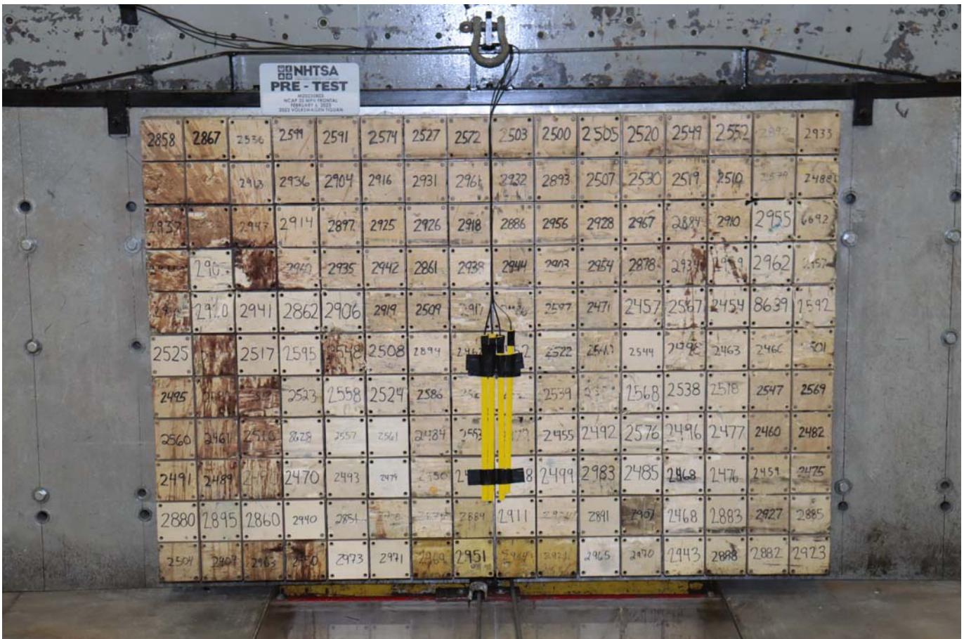
Photo No. 002 - Pre-Test Load Cell Wall
