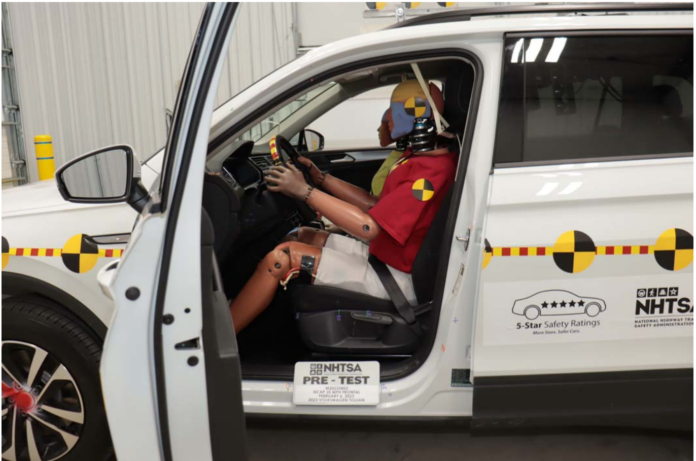
Photo No. 034 - Pre-Test Driver Dummy and Vehicle Interior View
