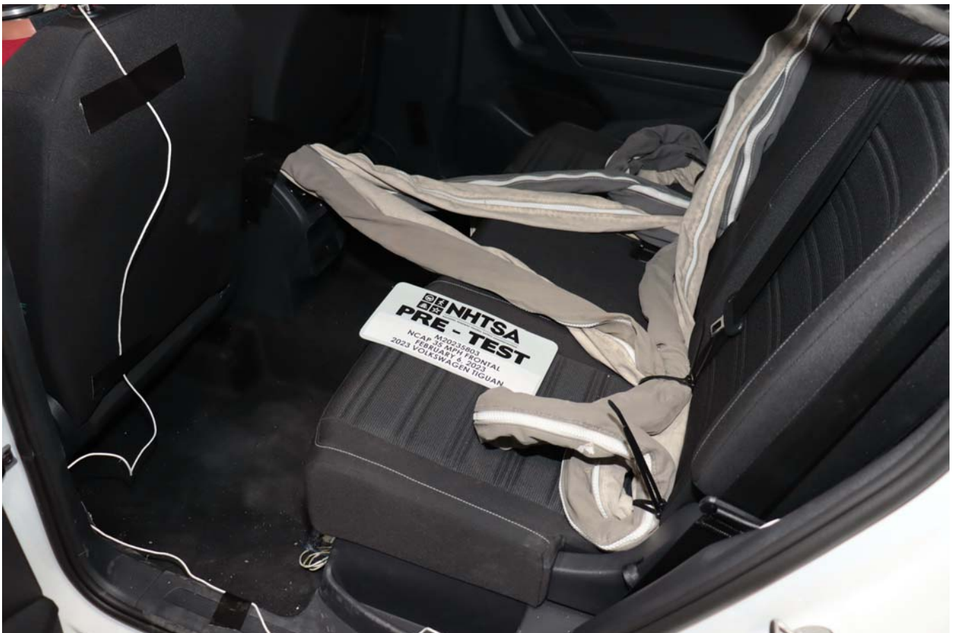
Photo No. 028 - Pre-Test Dummy Cable Routing
