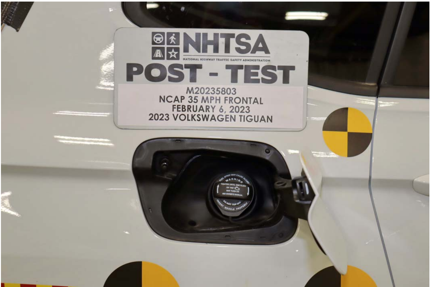
Photo No. 023 - Post-Test Fuel Filler Cap View
