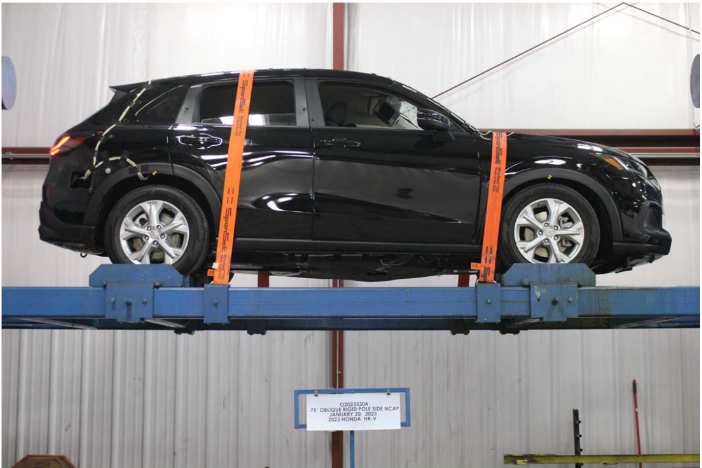
Photo No. 069 - FMVSS Photo No. 301 Static Rollover 360 Degrees
