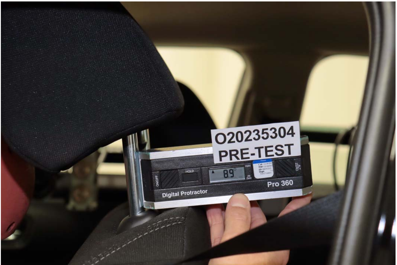
Photo No. 039 - Pre-Test Close-Up View of Driver Seat Back or Head Restraint
