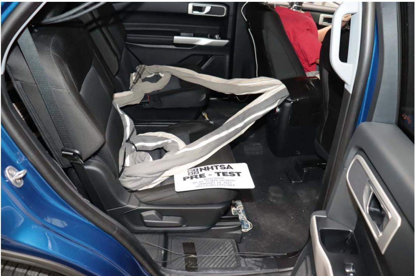
Photo No. 028 - Pre-Test Dummy Cable Routing
