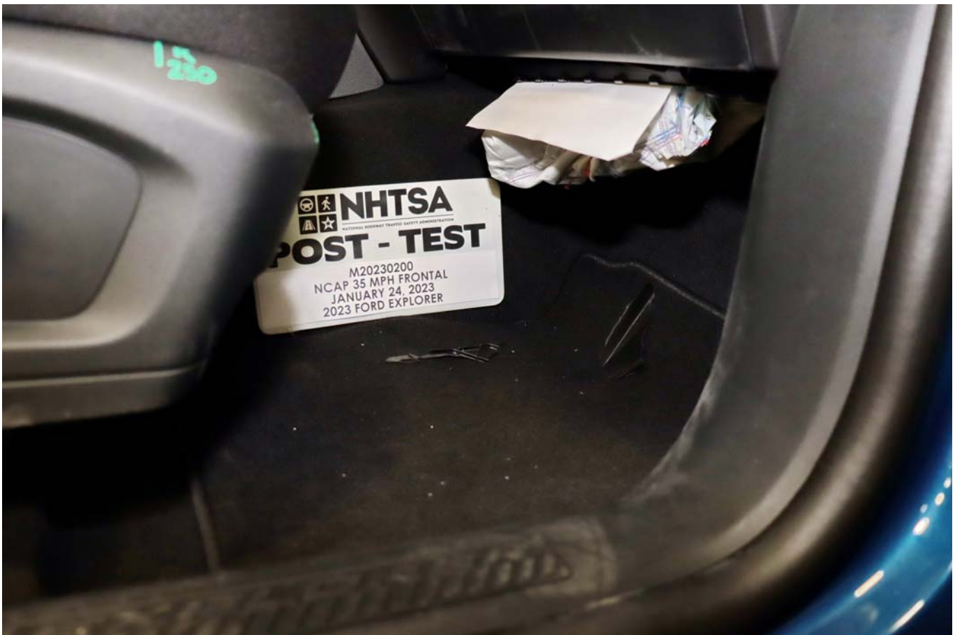
Photo No. 070 - Post-Test Passenger's Side Floorpan
