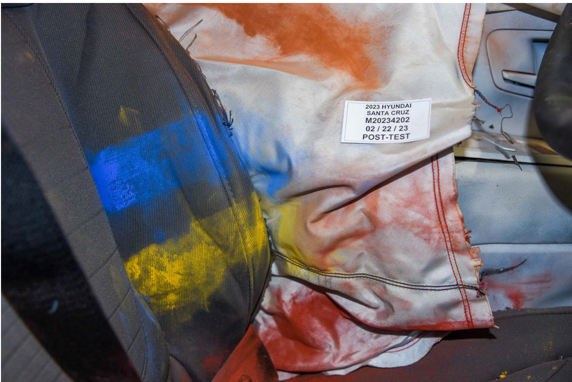
FIGURE 48. Post-Test Dummy Close-Up Torso Contact With Vehicle Interior View. Incorrect Placard. Correct NHTSA No. M20234201 and Test Date 2/23/23
