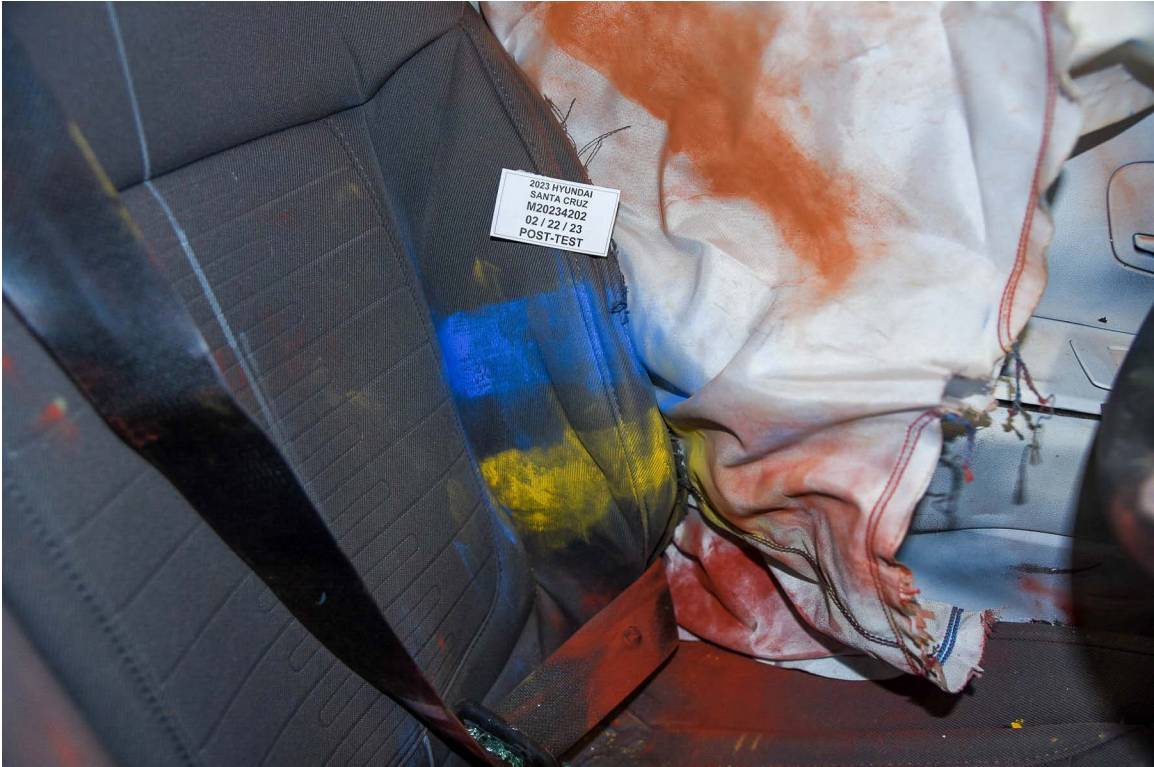
FIGURE 49. Post-Test Dummy Close-Up Torso Contact With Side Airbag View. Incorrect Placard. Correct NHTSA No. M20234201 and Test Date 2/23/23
