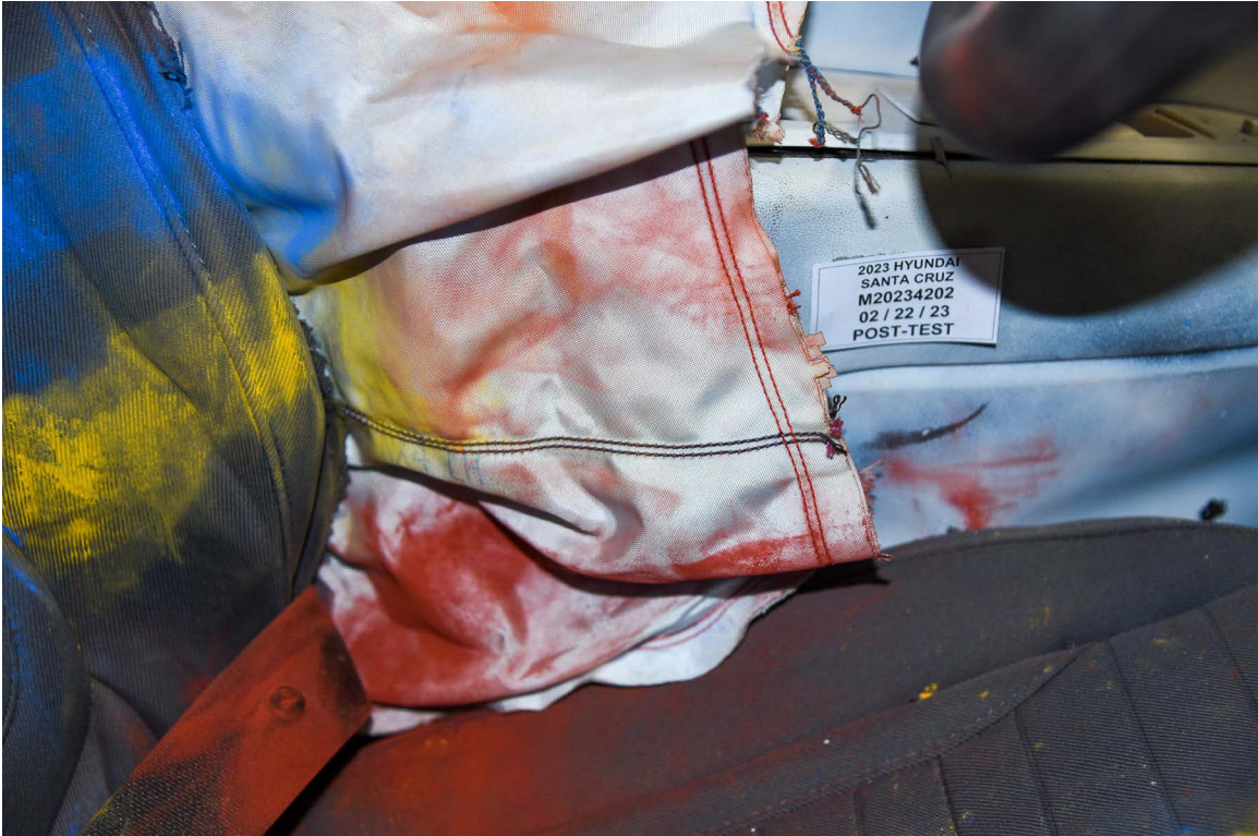
FIGURE 51. Post-Test Dummy Close-Up Pelvis Contact With Side Airbag View. Incorrect Placard. Correct NHTSA No. M20234201 and Test Date 2/23/23
