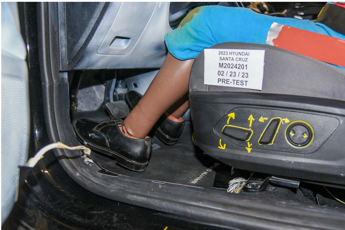
FIGURE 32. Pre-Test Placement of Dummy's Feet Incorrect Placard. Correct NHTSA No. M20234201
