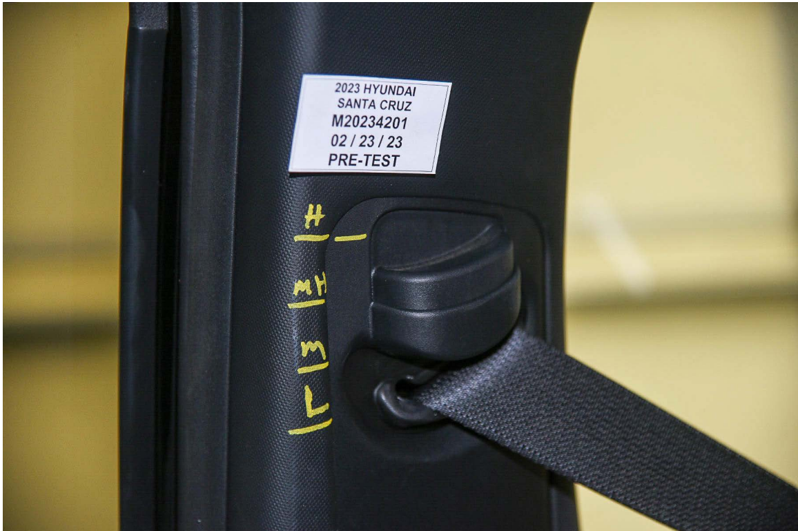
FIGURE 33. Pre-Test View of Belt Anchorage for Dummy
