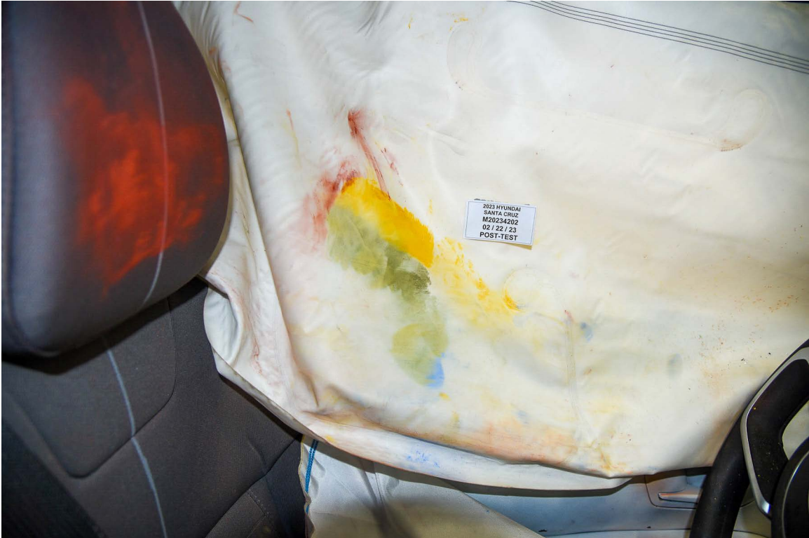
FIGURE 47. Post-Test Dummy Close-Up Head Contact With Side Airbag View. Incorrect Placard. Correct NHTSA No. M20234201 and Test Date 2/23/23
