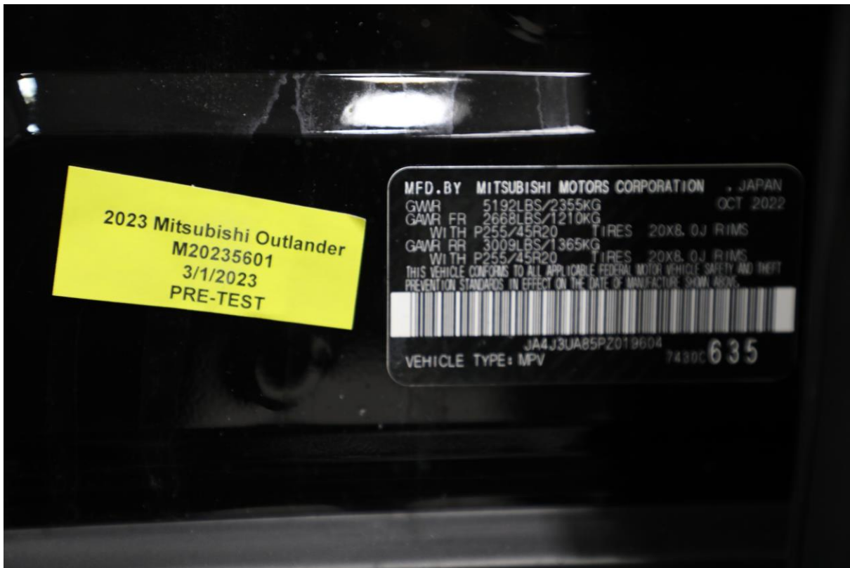
No. 057 Close-Up View of Vehicle Certification Label
