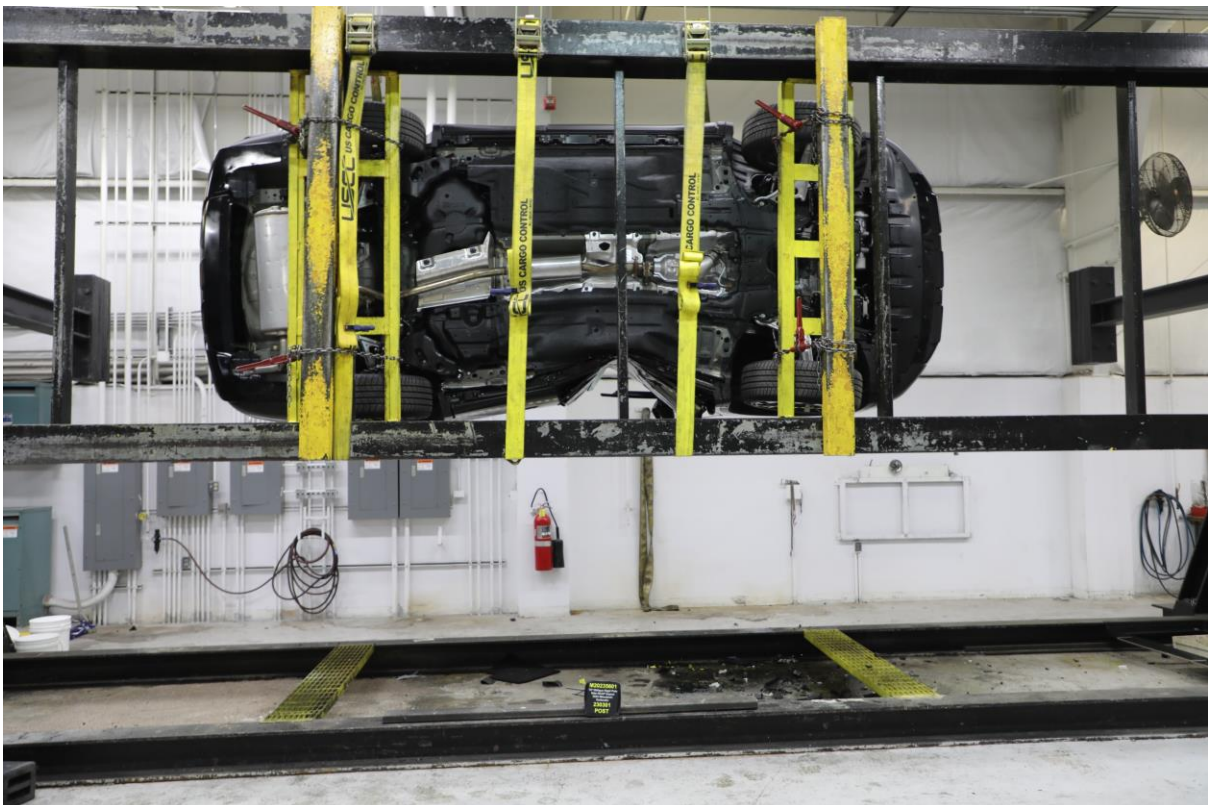
No. 068 FMVSS No. 301 Static Rollover 270 Degrees
